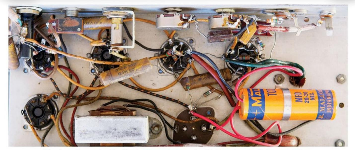
Simple as it may be, the Century's control panel with three inputs, Volume and Tone controls, and independent power switch offered more than many amps of its day. Within the simple folded-steel chassis, components were wired in the true point-to-point style of the era. The only replacement part is the "newer" orange-and-blue Mallory electrolytic cap — evidence of maintenance performed many years ago.
