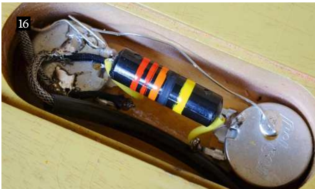
16. The new Junior's circuit appears very similar to the original, without the dust!
