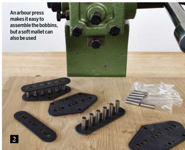
The main components for T-type pickups include top and bottom flats, baseplates, eyelets, magnetic slugs and magnet wire
