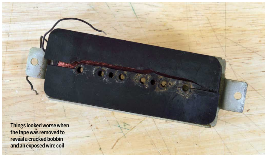
The broken bobbin and baseplate arrived wrapped in tape and didn't look promising, but the parts were all from a 1950s P-90
