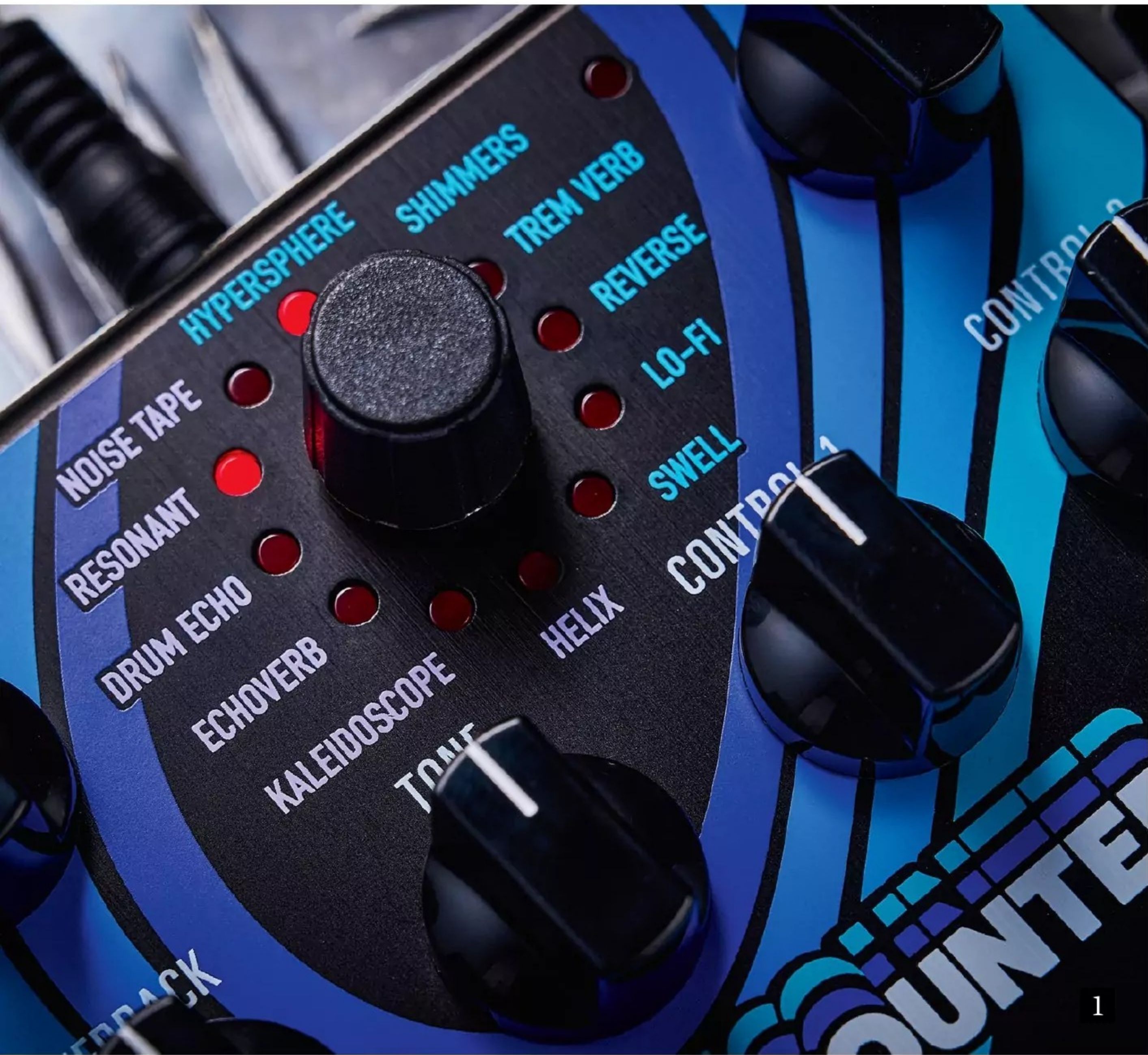
1. The Control 1 and Control 2 knobs manage engine-specific parameters such as Modulation and Phase Shifter for the Hypersphere reverb, Tremolo Depth and Rate for the Trem Verb, or Wash and Rhythmic Patterns for the Drum Echo
