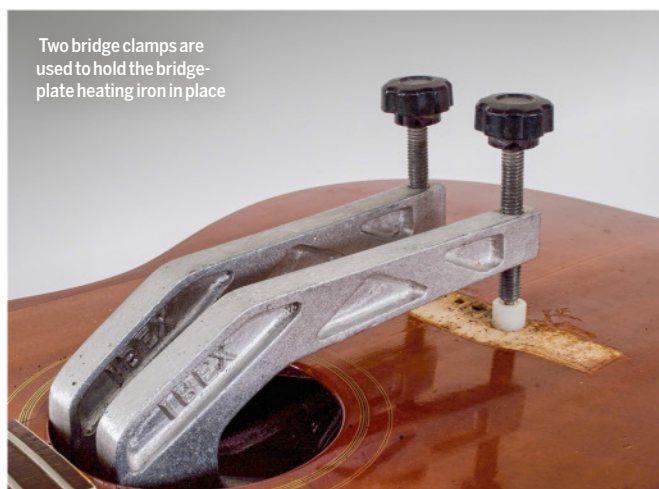
With thick sheets of cardboard protecting and insulating the top, a travel iron is used to soften the glue holding the bridge
