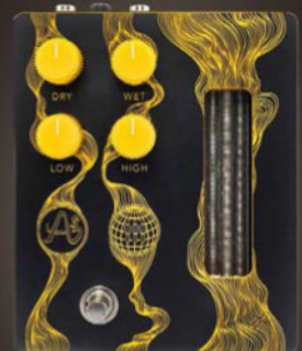
La Grotte by Anasounds/Third Man Hardware is a feature-packed pedal with real springs
