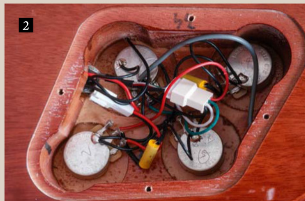
1. Typical Gibson USA components here, and you can clearly see the modern-wired capacitors
