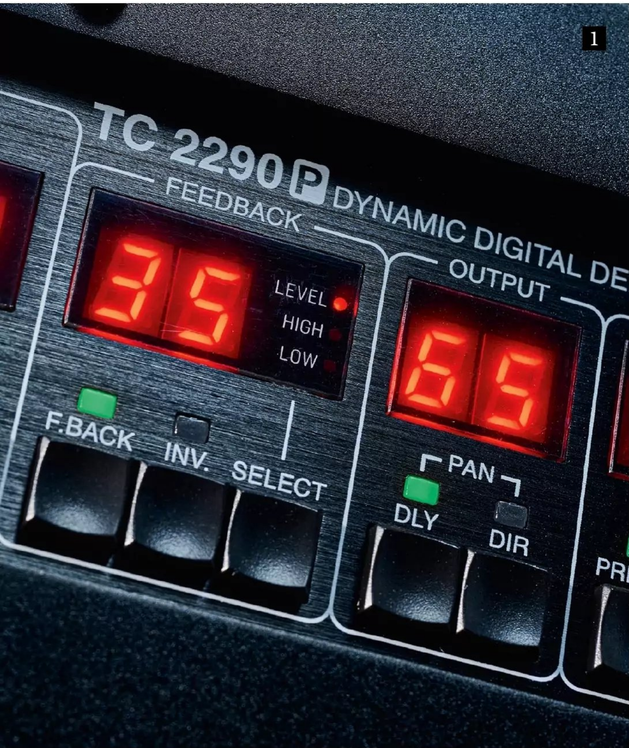
1. The front panel is split into various sections. For example, you can set the amount of feedback and invert the phase of it here; plus select the High and Low filters to adjust the tone of the repeats. The Output section is where you set the mix of direct and delay sound, between a value of 0 and 99. Press the two buttons together to set left/right panning
