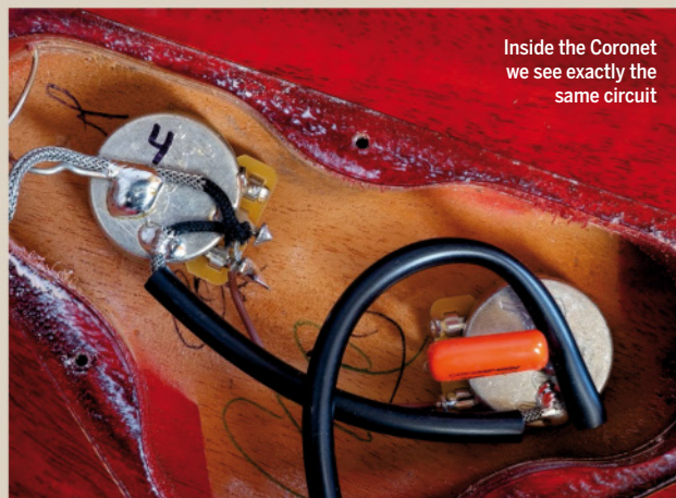
The Junior's control cavity has just enough room for the two pots and capacitor
