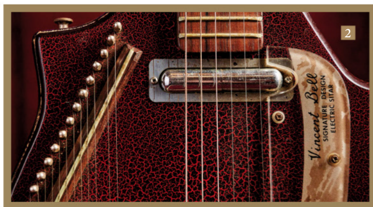
2. Sympathetic 'drone' strings, 13 in number, provide some of the shimmer of a real sitar. They are tuneable and have their own dedicated pickup
