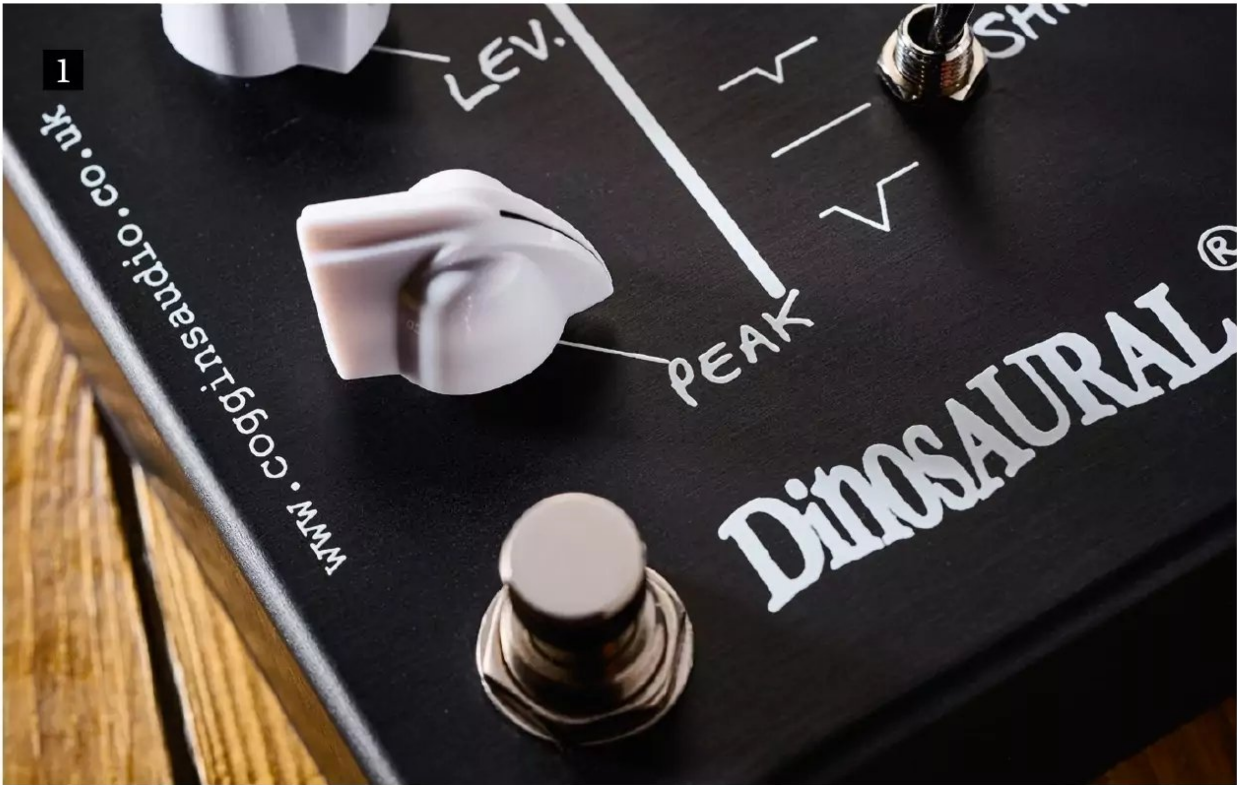
1. This Peak knob offers increasing distortion with progressively higher gain but narrower bandwidth midrange boost
