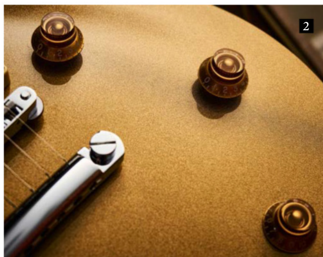
2. Via a push-push switch, the volume control doubles as a mute/kill switch. The middle tone control has a push-push out-of-phase switch. The lower control is Wilkinson's Varicoil to single coil Varicoil control
