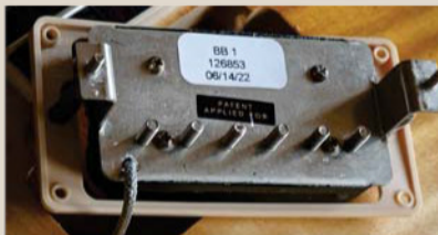
Top: Both our SG and 60s LP use the same 61 Burstbuckers – all appear to have been wax potted Above: The 50s LP uses a Burstbucker 2 at the bridge and a 1 (pictured) in the neck position
