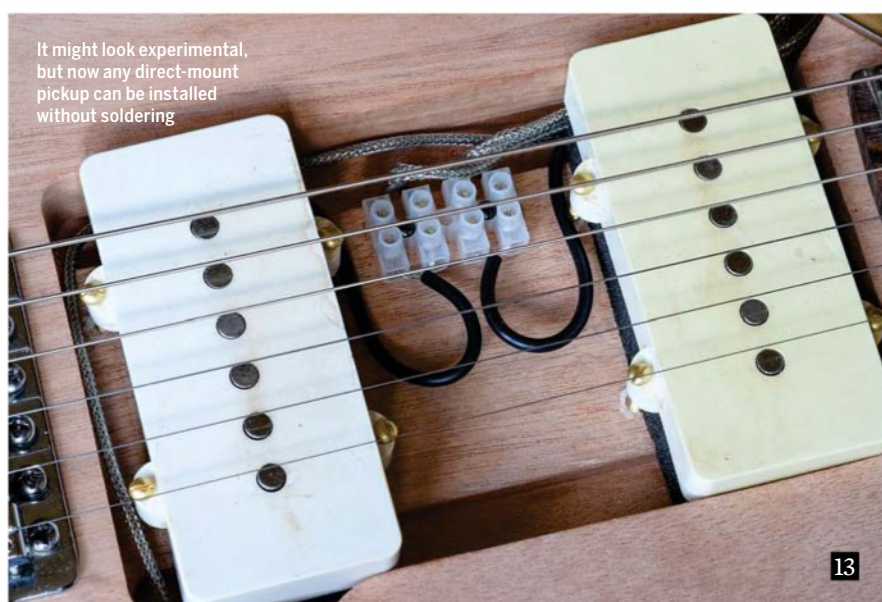
12 Finding the right screw for the job isn't always easy. These brass pickup mounting screws are perfect!
