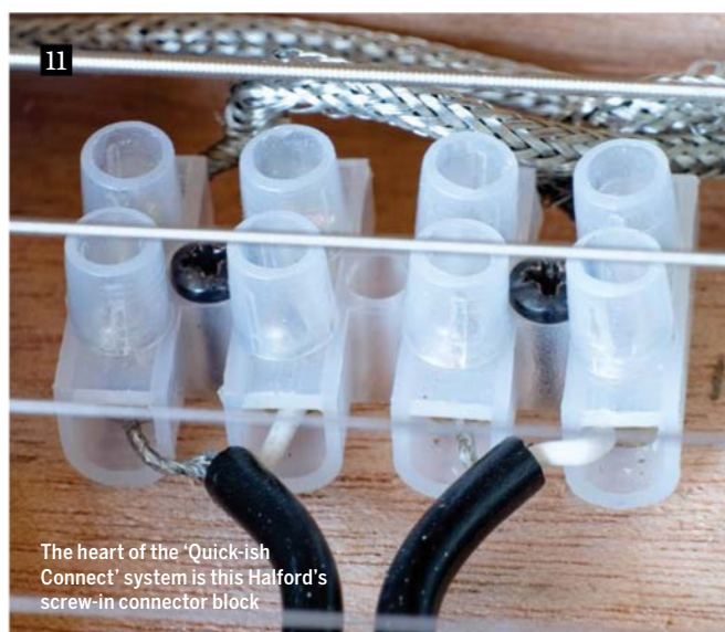
It might look experimental, but now any direct-mount pickup can be installed without soldering
