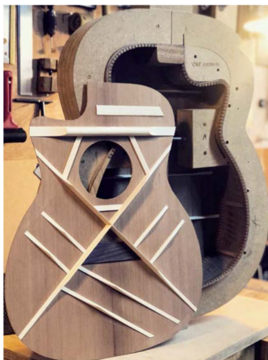
Alex creates his X-braces with smaller 'fingers' to help deliver a more pleasing tone
