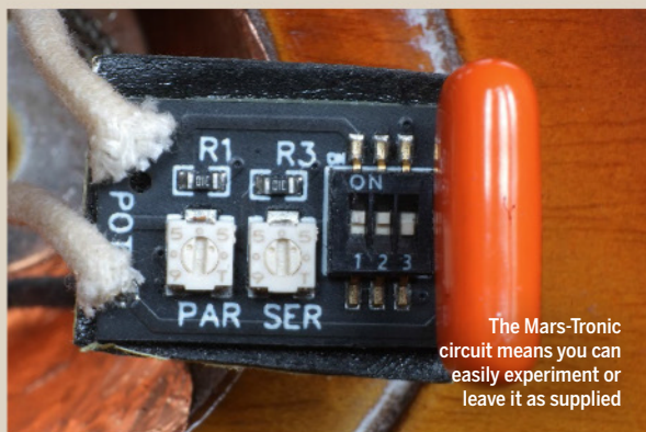
The tidy wiring is dead simple as from the variable treble bleed circuit
