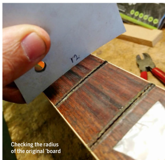
Initial levelling of the fingerboard
