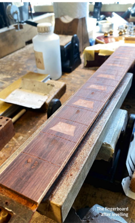
You can still see a little wear left after levelling
