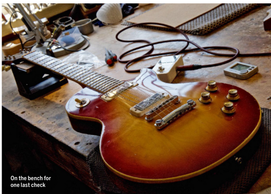
Final intonation check on the newly installed Faber bridge
