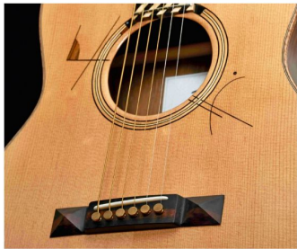
This attractive 'pyramid' fixed bridge demonstrates both technical skill and artistic flair
