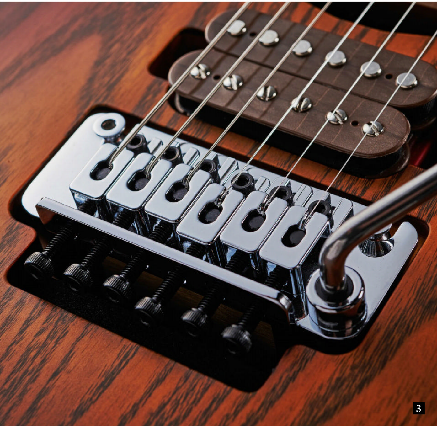
3. This wide-travel vibrato, based on the Floyd Rose design, is recessed into the body and back-routed. It's an all-steel design with brass block and push-in, tension-adjustable arm
