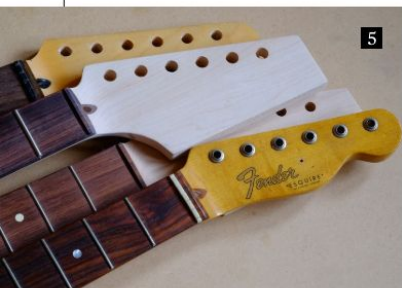
Three potential bodies for our partscaster build (4). The HSH Guitarbuild body is flanked by two Fender Roadworn bodies in various states of repair. Unless the supplier is licensed by Fender, you'll have to cut your own outline from the 'paddle' headstock (5)
