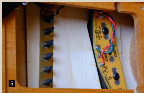
5. With the central rear cover removed, you can see the Noiseless Telecaster pickup, but there's no body sensor, as with the USA models
