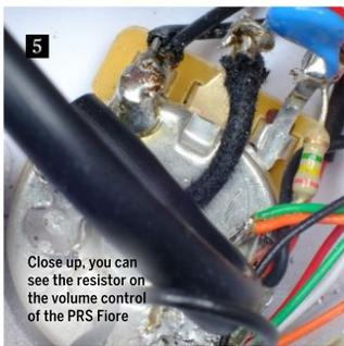
Close up, you can see the resistor on the volume control of the PRS Fiore
