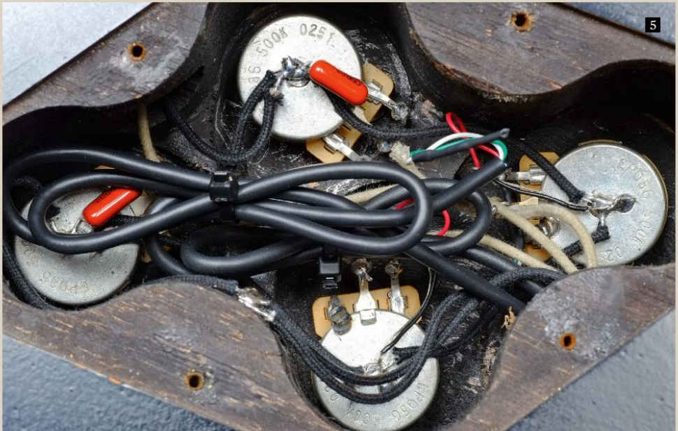
5. There's plenty of wire packed into the V100, but it's a vintage-style circuit again
