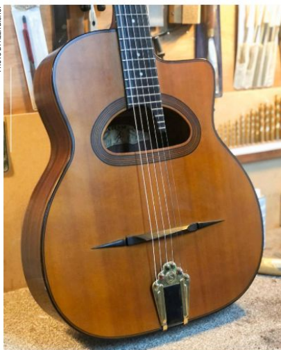
Alex's exemplary work on this Gypsy-style guitar included moving the fret dots and making the moustache ends
