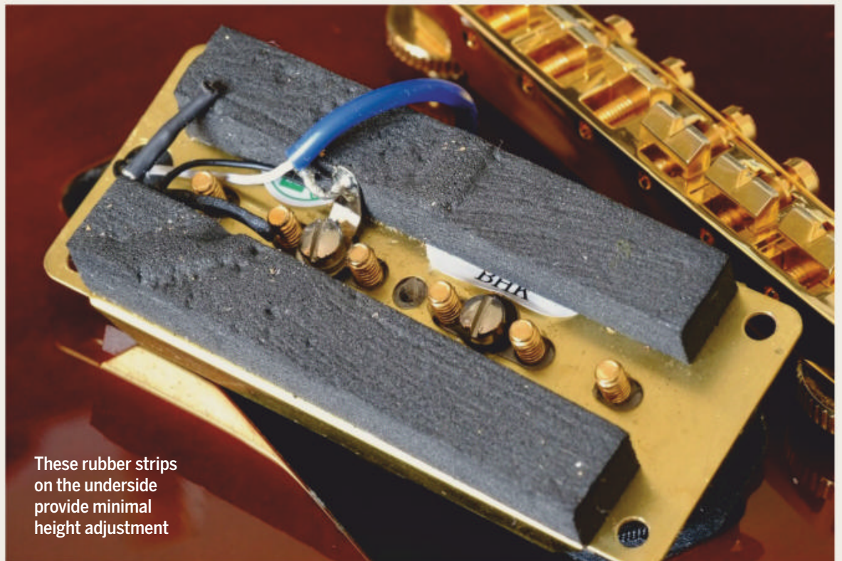
The circuits are the same on both guitars, although the P90 (here) doesn't have the pull/push switched volumes
