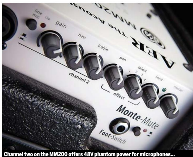
Channel two on the MM200 offers 48V phantom power for microphones...
