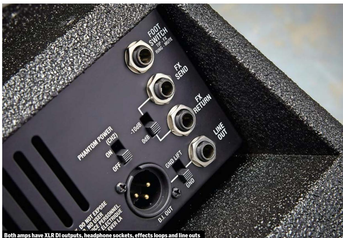
Both amps have XLR DI outputs, headphone sockets, effects loops and line outs
