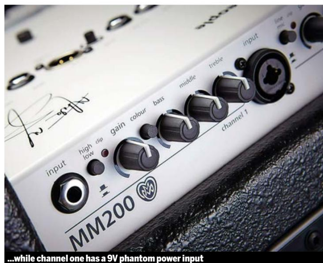
...while channel one has a 9V phantom power input
