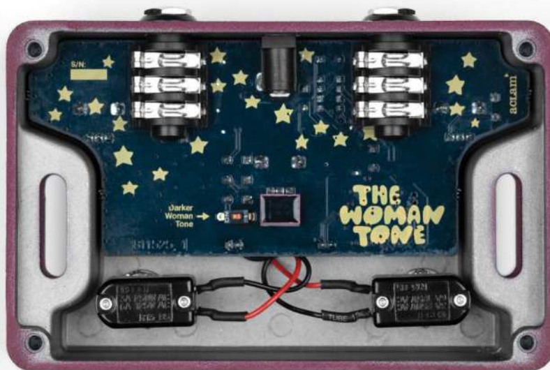
The Darker Woman Tone switch is located inside the pedal.
