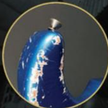
Nitrocellulose lacquer finish and detailed aging process
