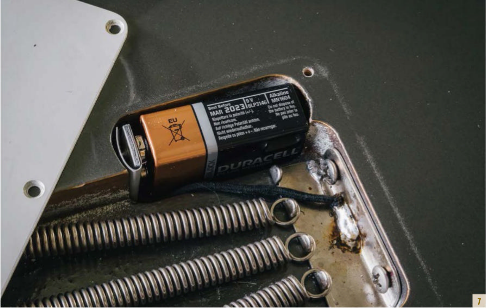
7 The battery wedges into this recess adjacent to the vibrato springs, and the plastic cover holds it in place
