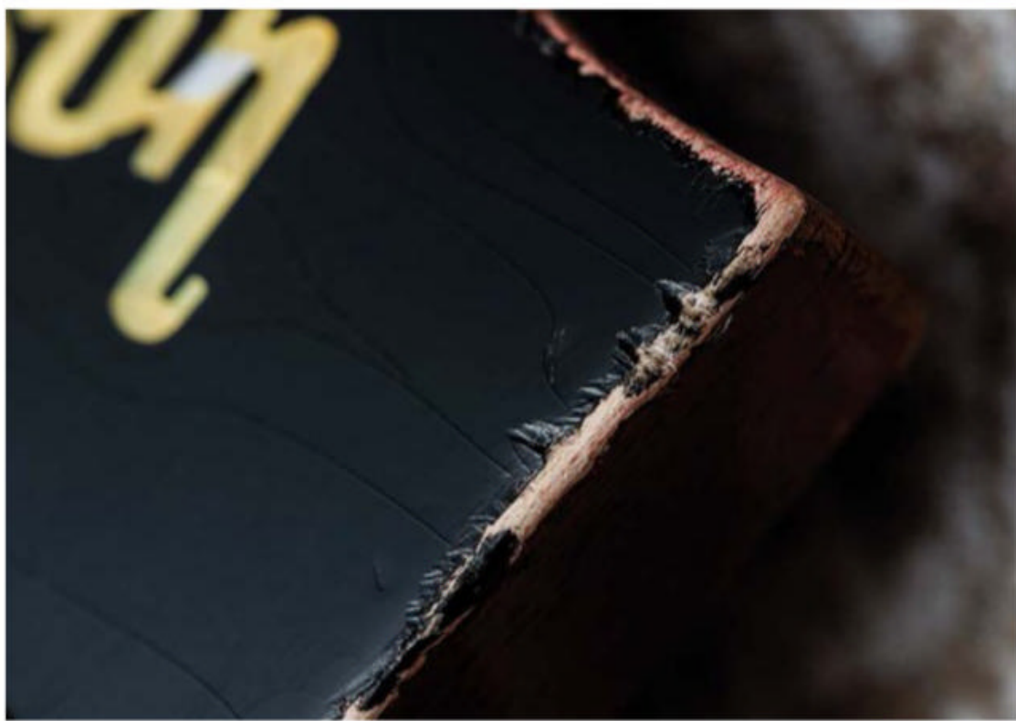
The finish chipping on the Light Aged model's headstock reveals how thinly the Murphy Lab lacquer has been applied
