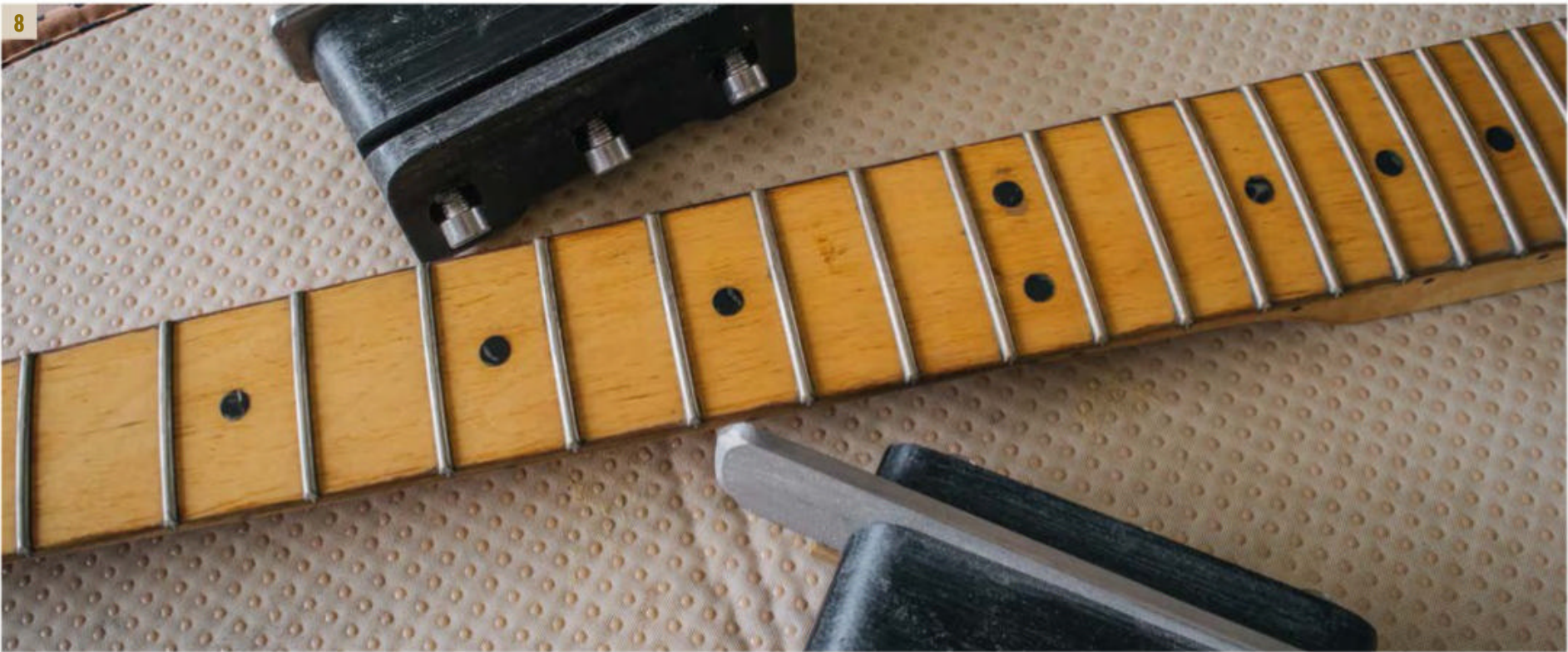
8 Fret-bevelling tools with diamond files can smooth and tidy up the fret ends
