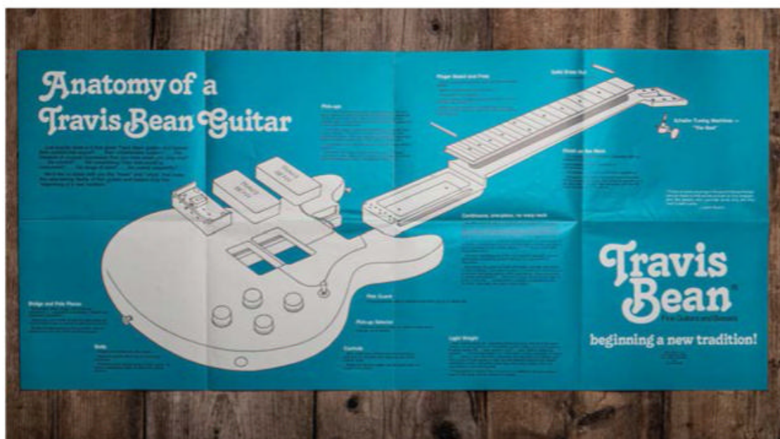
Travis Bean's TB1000S had an innovative aluminium alloy through-neck design
