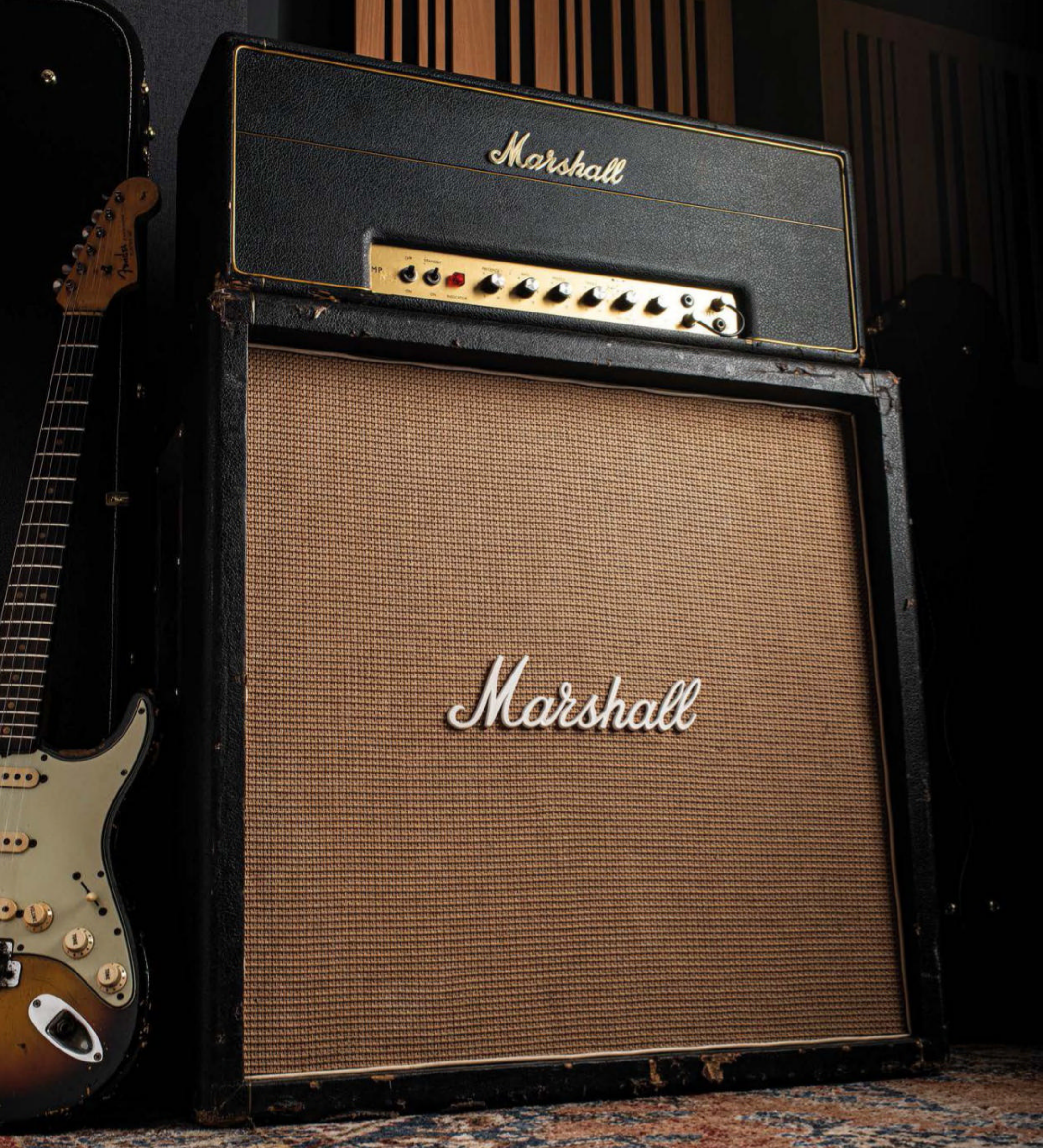
ABOVE A Marshall 4 x 12 cabinet loaded with Celestion Greenback speakers is the ideal match for a 100W Super Bass
