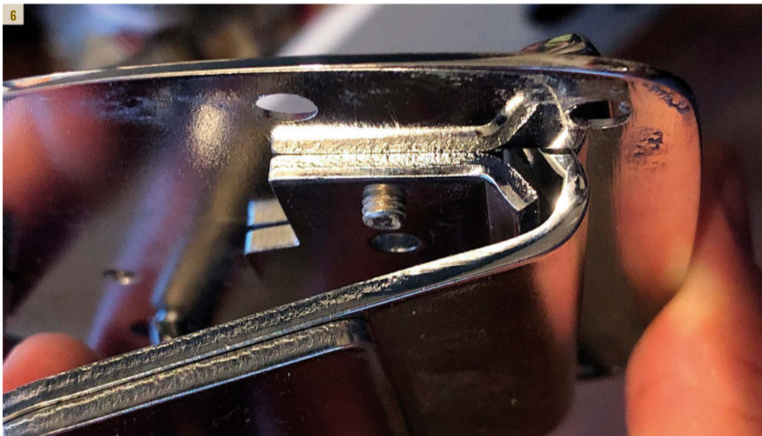
4 It's crucial to smooth out the side of the legs that make contact with the anchor plate
