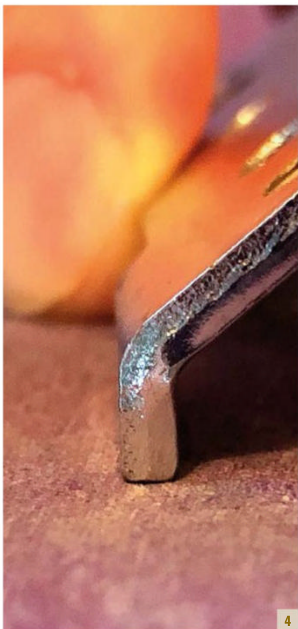
4 It's crucial to smooth out the side of the legs that make contact with the anchor plate
