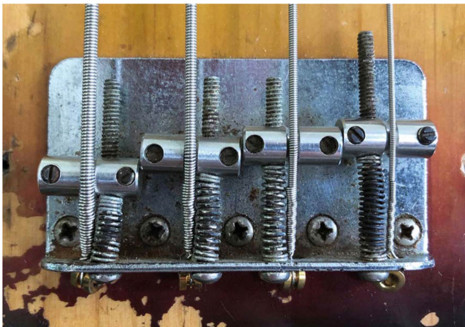
Most electric guitars and basses have adjustable saddles of some description, and these are the key to getting your instrument perfectly intonated
