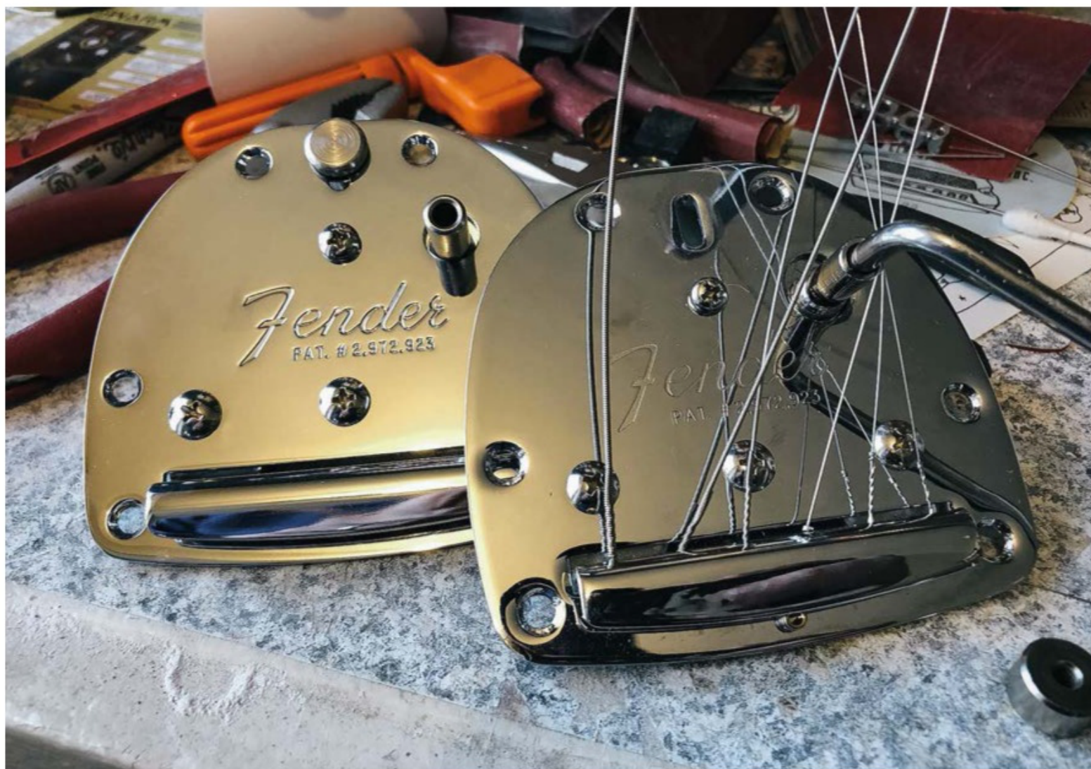
There are a few differences between the vibratos found on AVRI (left) and Classic Player models (right), most notably the screw-in arm on the Classic Player
