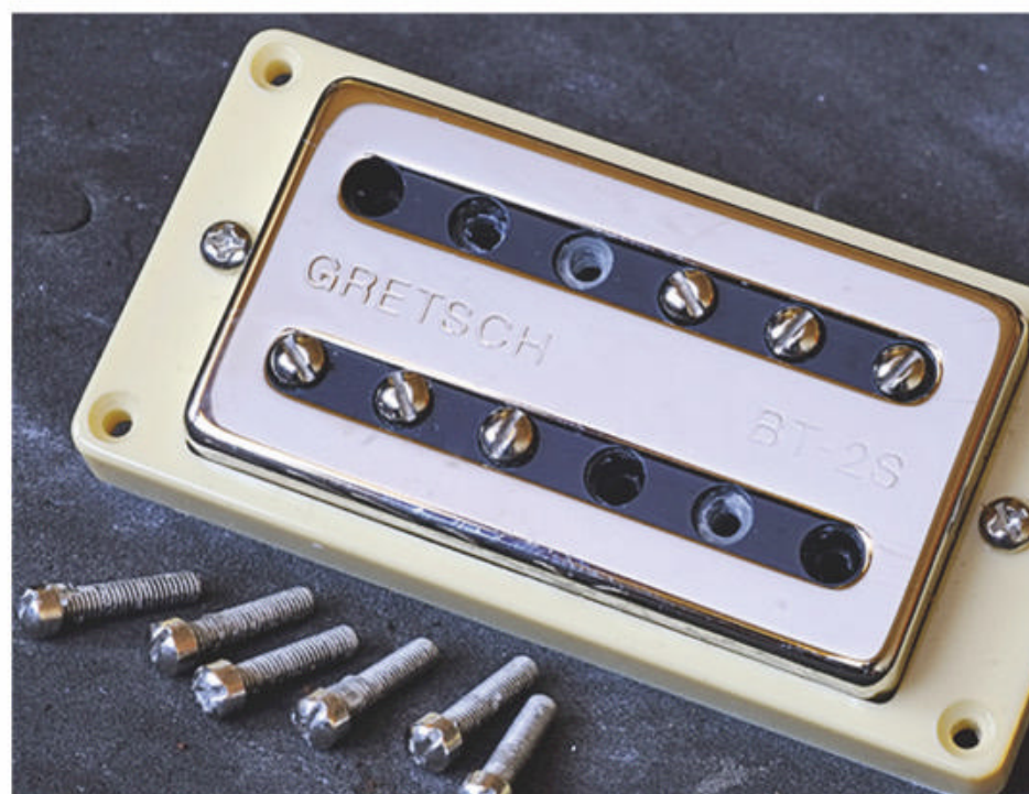
Inspired by Cream T's Original Banger (left), the Gretsch Broad'Tron BT-25 (right) has half its screw slugs removed – the lower three of the top coil and the top three on the lower coil nearest the bridge.
