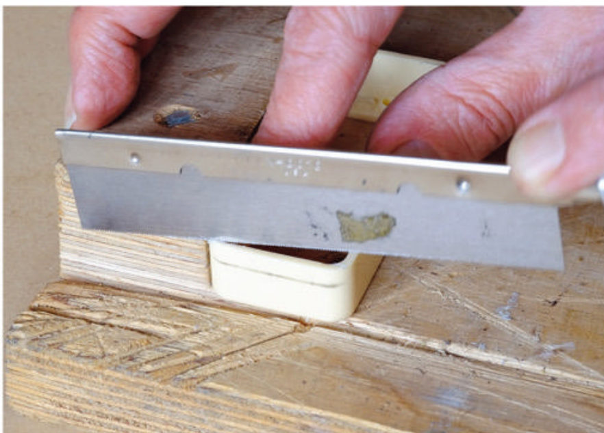
Cutting the mounting ring walls so the oversized ring will sit over the pickup rout
