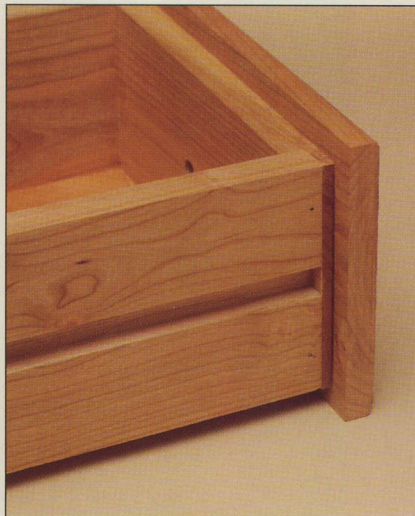
Lipped front: A rabbeted front creates a lip that is useful for concealing commercial runners when the drawer is closed. Lip performs double duty as drawer stop
