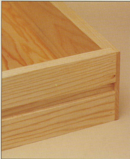
Flush front: Allows the drawer to fit entirely within the carcass; also known as an inset drawer
