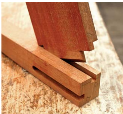
To maximize the length of the tenons in the rear legs, the ends are mitered.
