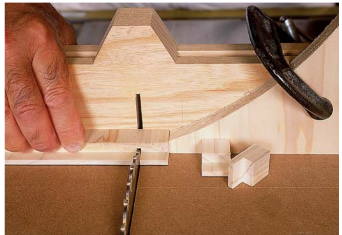
Cut a rabbet across the end of a wide board, then cut off a strip as long as you want the buttons to be. Clip the strip into uniformly sized buttons.
