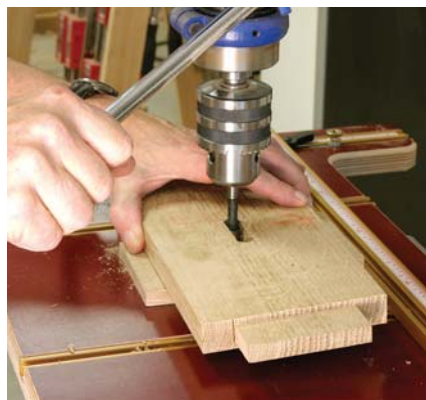
The angled mortises on the lower rails were roughed out with a Forstner bit on the drill press. A tapered block under the workpiece makes the holes at the correct angle.
