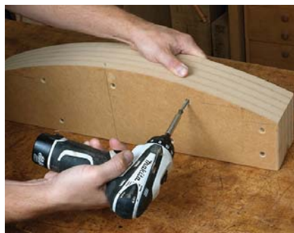
After band sawing the curves, template-rout multiple layers of MDF and screw them together. Once the form is assembled, make sure the face is smooth and fair.
