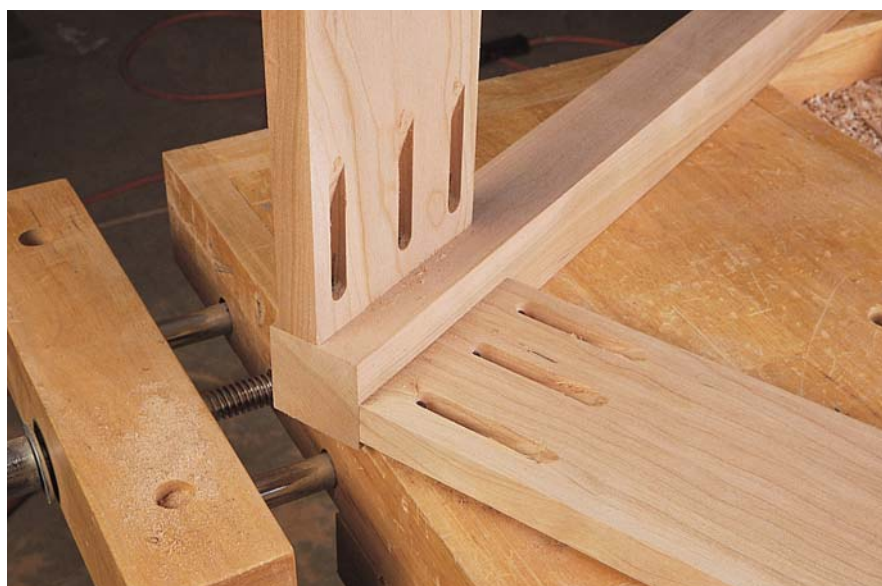
Pocket screws aren't my first choice for building dining tables, but for a small occasional table, it'll work.
