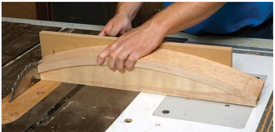
Made of scrap band sawn to the shape of the inner curve and screwed in position, this simple jig positions the workpiece against a miter gauge to trim the ends square at the table saw.
