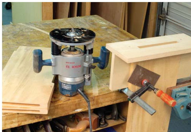
Loose tenons make quick, strong joints. Using a series of templates and a guide collar locates and cuts mortises for loose-tenon joinery.
