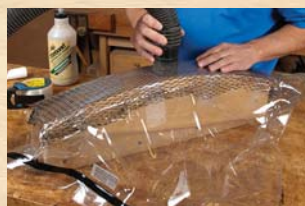
7. Once the bag is sealed, a shop vacuum sucks the bulk of the air out of the bag.
