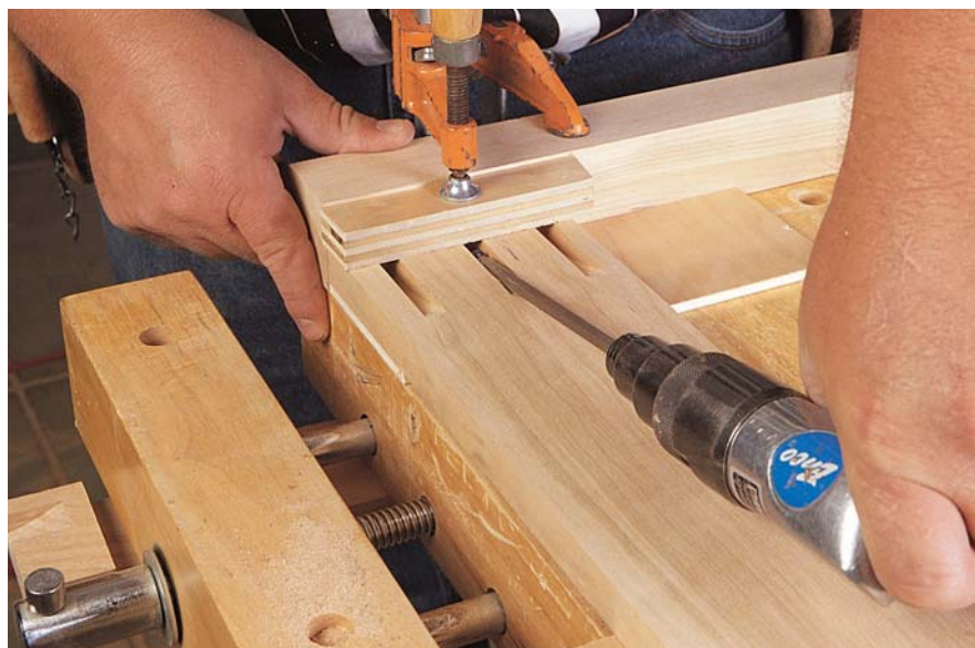
Be sure to glue the joint and hold the leg and apron together tightly while screwing it together.
