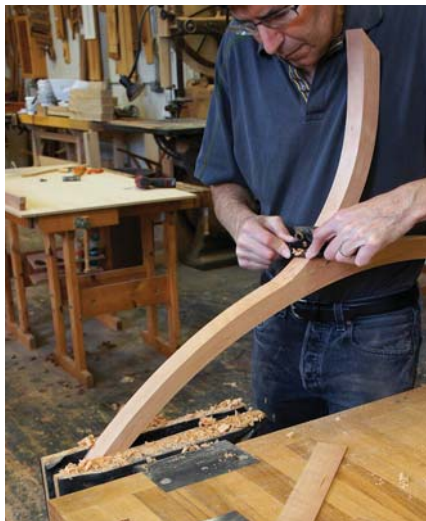
Clean up the transition between the wing and the arch to provide a smooth bed for the last laminate.
