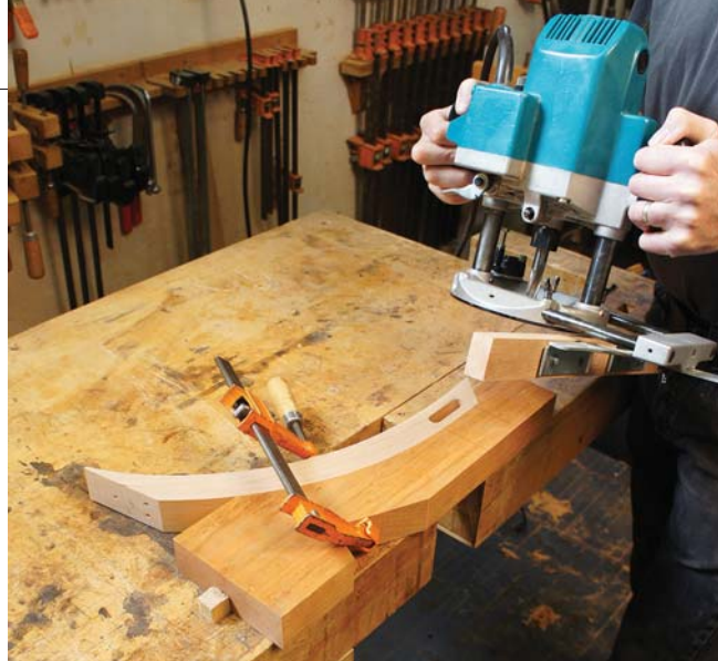
This jig provides a flat reference for the router fence and holds the wing securely to make the mortise.
