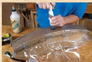
8. Use the hand pump that comes with the veneer kit to remove the last of the air from the bag.
