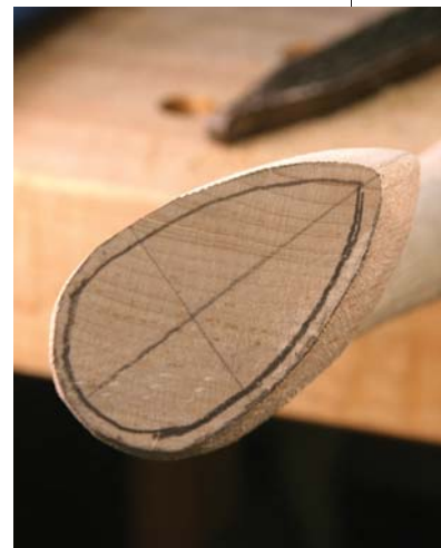
The edges of the feet taper \frac{1}{8}" while the heel continues to roll to the floor. Draw the inner profile freehand.
