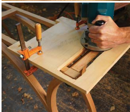
This jig provides a flat surface for the router base, bringing the front-to-back rails and the tops of the wings flush with the aprons.
