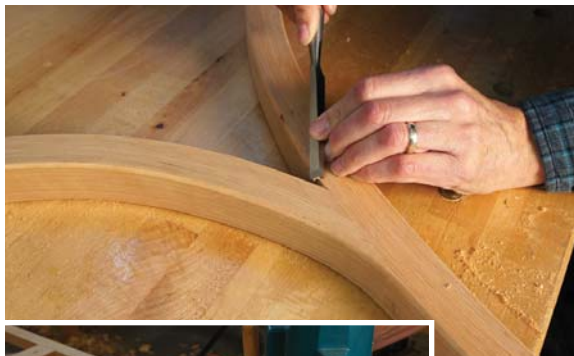
A router bit won't reach the inside corner to shape the edge. Carve into the corner from both directions.
