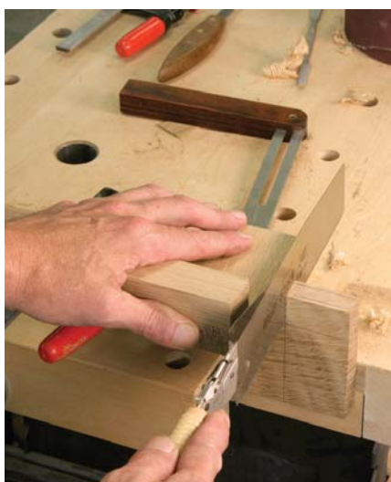
The quick and easy way to make the angled cuts for the through tenons is with a handsaw, guided by an angled block of wood.
