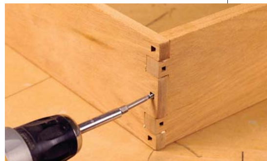
Screws hold the drawer joints together and are hidden when the ebony plugs are put in.
