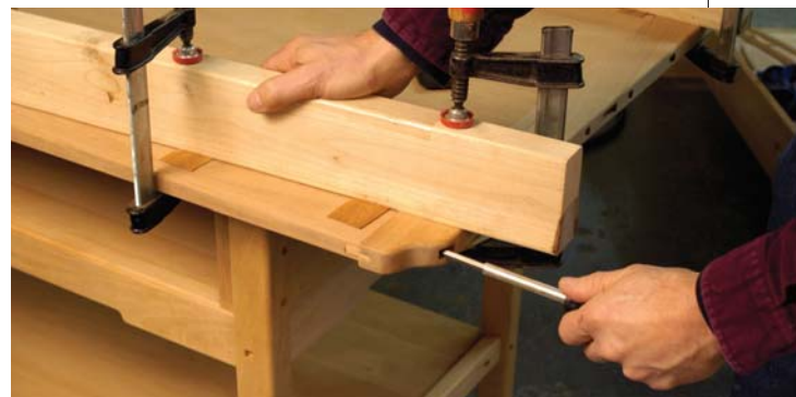
The 2x4 caul keeps the face of the breadboard end parallel to the face of the top. Veneer under the caul keeps the surfaces aligned.
