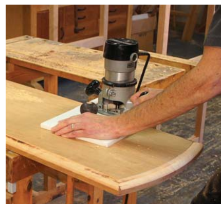
After shaping and finishing the top, attach it to the base with screws through the front-to-back rails.
