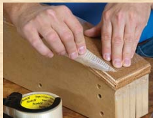
4. Apply a flexible \frac{1}{8} " Masonite or plywood platen over the top and tape the entire stack to the form.
