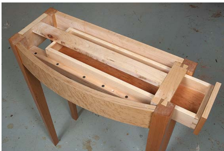
The assembled base is outfitted with drawer runners, a kicker and guides. The false drawer front looks like an apron when the drawer is closed – you can't even tell it's there.
