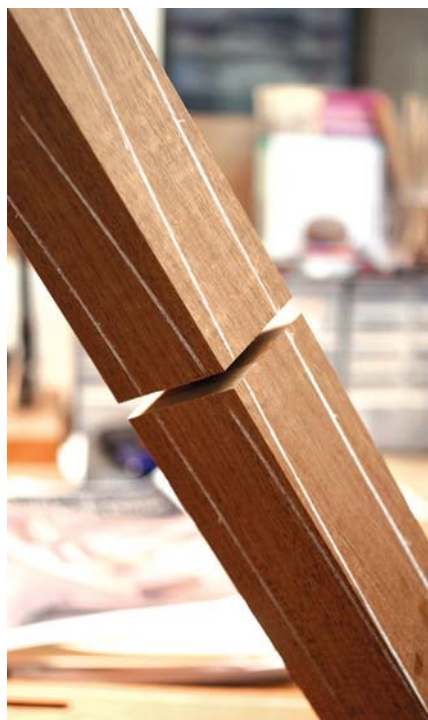
Before cutting the legs to shape, the dados for the bead are cut at the table saw. The dados on the back and inside are not as deep as on the front and outside.
