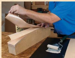
2. After your first unglued face is on the form, stack subsequent veneer layers in place with the glued face down.
