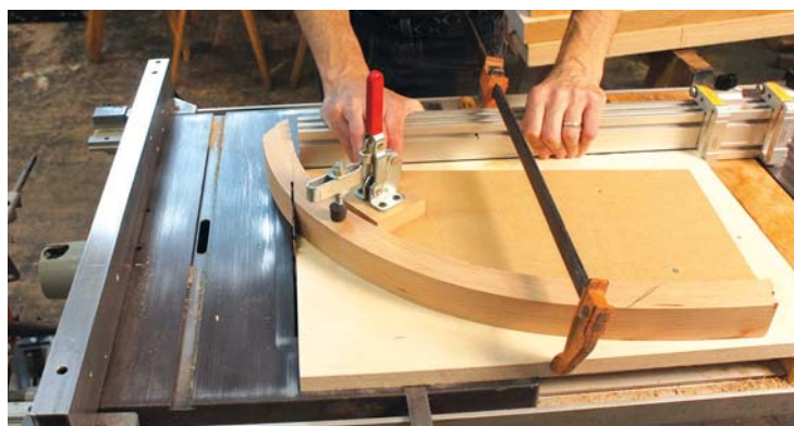
The jig holds the curved part securely to make the cut, creating a flat surface to attach the wing to the arch.
