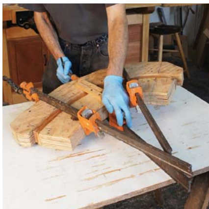
A form for the outside of the curve helps to spread clamp pressure, reducing the number of clamps needed.
