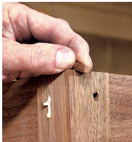
Split out the pegs. Then shave them to size with a paring chisel.
