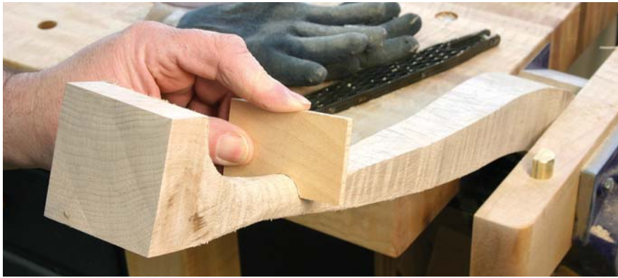
A simple shop-made jig is the perfect tool for defining the shape of the ankle of a cabriole leg. This slim tea-table ankle is 1".
