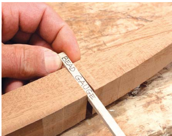
After shaping the leg, the dados should all be the same depth. I use a simple gauge block to check the dados and adjust as necessary.
