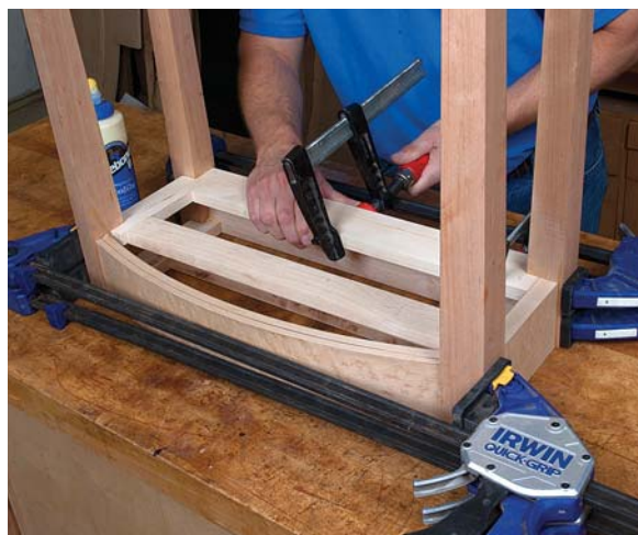
Clamp up the long aprons and add the drawer runners and kicker. Runners and the kicker are tenoned at both ends. The rear runner is also glued to the rear apron.
