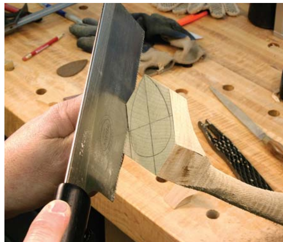
The majority of the waste in shaping the slipper foot is removed with a saw. It's important to plan the layout lines and cut to those lines. Deviations could alter the foot shape.
