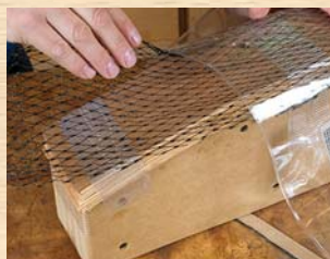
6. Netting over the top of the veneered stack provides a pathway for excess air to be sucked out of the bag once it's sealed.
