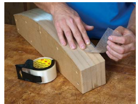
Skip the finish or wax altogether – a layer of slick packing tape is all you need to make sure glue squeeze-out won't stick to the form.
