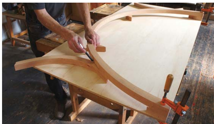
A piece of plywood locates the corners of the large arch and the wings. Mark the wings from the flats on the arches.
