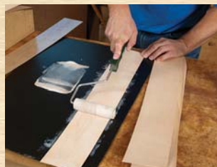
1. Spread a thin, even layer of glue on one face of the veneer. A 4" paint roller makes this work easy.
