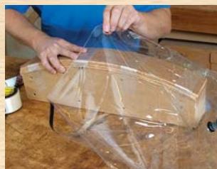
5. With the glued bundle of veneer taped in place on the form, slide the assembly into the vacuum bag.
