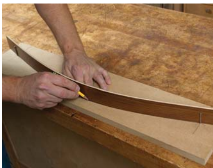
Bow a batten between finish nails driven into MDF and mark the curve. Remember to add length beyond the nails to allow for trimming and tenons.
