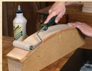
3. Spread glue on the opposing face (that way, if you miss a spot on one face the glue-up will still be OK).
