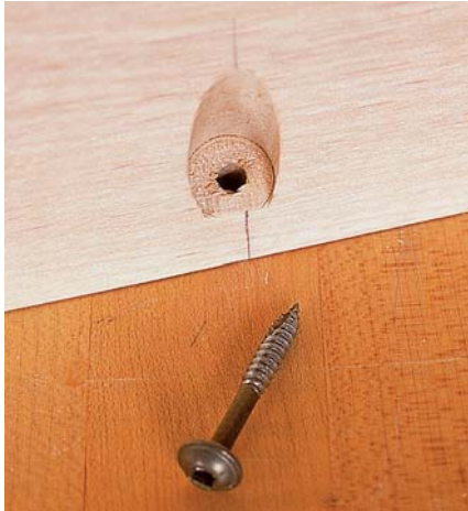
The completed pocket is flat-bottomed and large enough for a screw with an integral washer.
