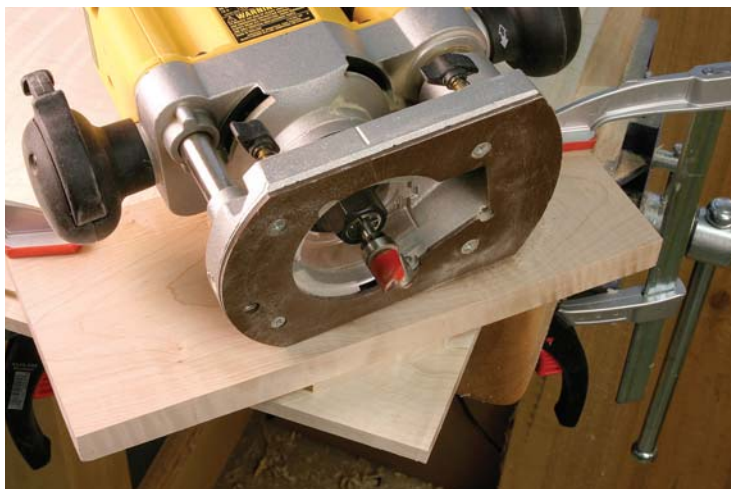
Any straightedge and a pattern router bit, in this case a \frac{5}{8} "-diameter bit, produces a clean cut at the top corners to allow for the recessed top to fit in position.
