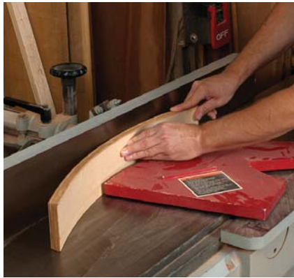
Joint one edge of the assembled front apron. Be sure one hand holds the apron flush to the fence as you square the edge to the face.
