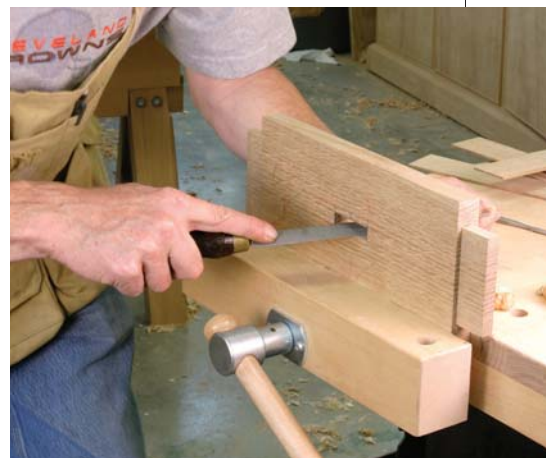
After squaring the corners of the mortise with a chisel, I use a rasp to finish smoothing the inside of the angled joint.
