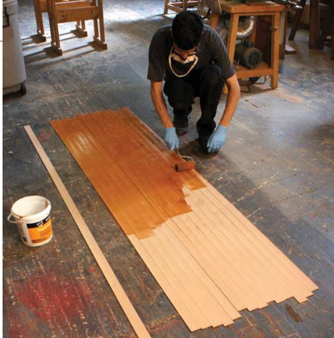
A paint roller makes quick work of spreading the glue evenly on all of the laminations.
