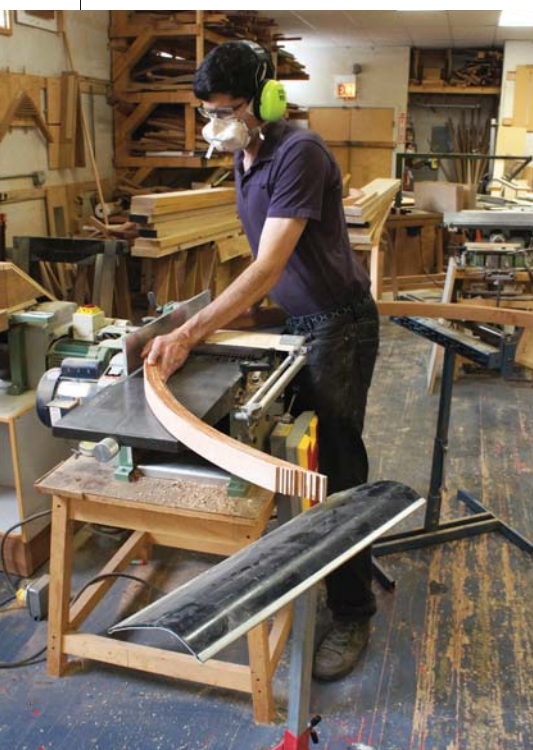
The jointer levels the surface of the lamination. Infeed and outfeed supports help keep the material flat on the machine bed.
