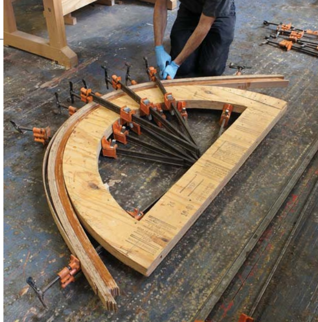
Before you add glue, do a dry run to ensure you've enough clamps – and that when the glue is on, you know where to place them.
