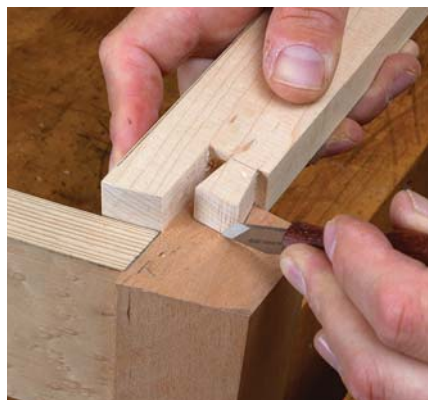
The stretcher above the drawer is marked to length, notched and dovetailed. The dovetail is then transferred to the top of the leg. The bulk of the dovetail slot is routed out, then chiseled to fit.
