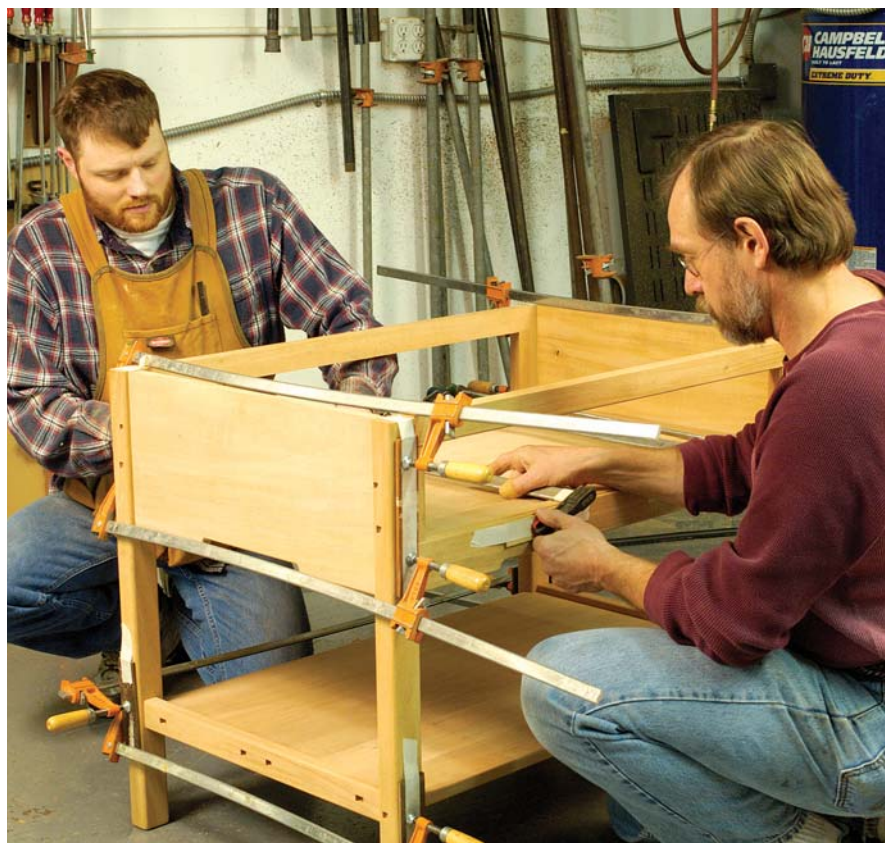
Assembling a complicated project goes smoothly when the process is viewed as a series of subassemblies.
