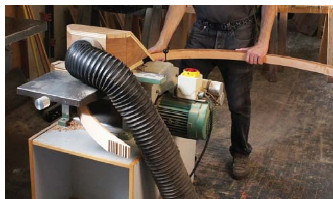
The opposite side of the glued lamination is surfaced with the planer.
