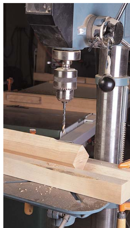
Use the bracket as a template for locating the holes for the corner bracket. Then use a drill press to make your pilot holes.
