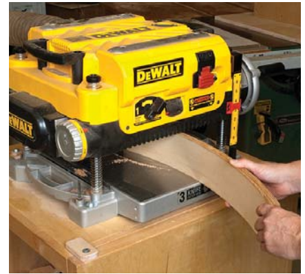
With the flattened edge facing down, guide the curved apron through the planer to square and bring the other edge parallel to the first.
