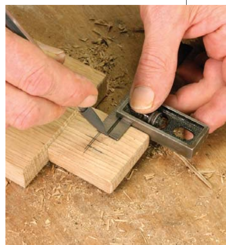
After fitting the through tenon, the location of the second mortise is laid out, keeping the back of the hole just behind the face of the rail.
