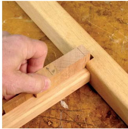
The end cut scrap is used again to check the width of the notch in the leg.
