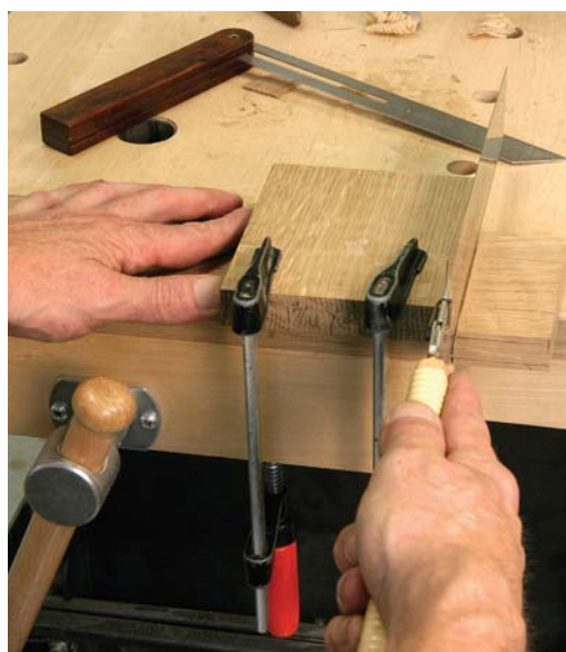
These angled shoulder cuts would be tricky to make with power tools.
