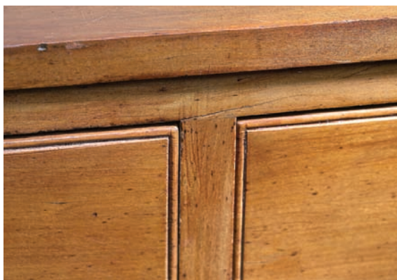
The scratch-stock cock bead on this chest of drawers retains a crisp appearance even in this close-up.
