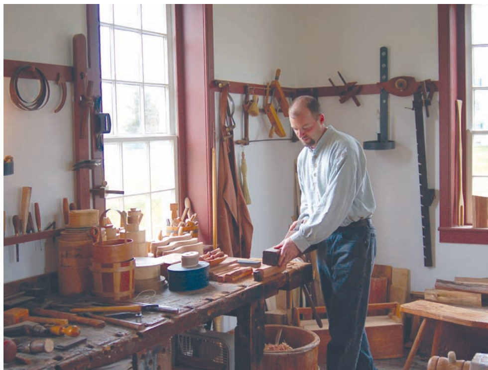
ABOVE Bob Roemisch levels a surface on a turning blank using an antique trying plane, not of Pleasant Hill origin.
