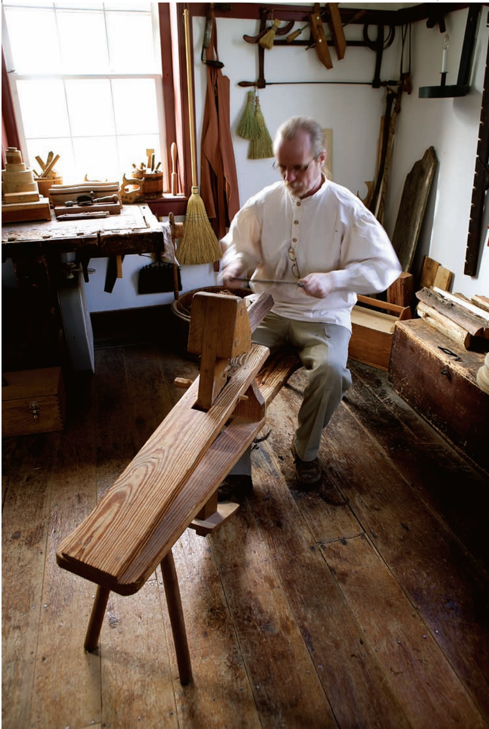
LEFT Mark Ross, a costumed interpreter who demonstrates woodworking techniques, uses a drawknife on work held in place by the head of a shaving horse. The work is held in place by the action of the user's feet, freeing both hands for the drawknife.
