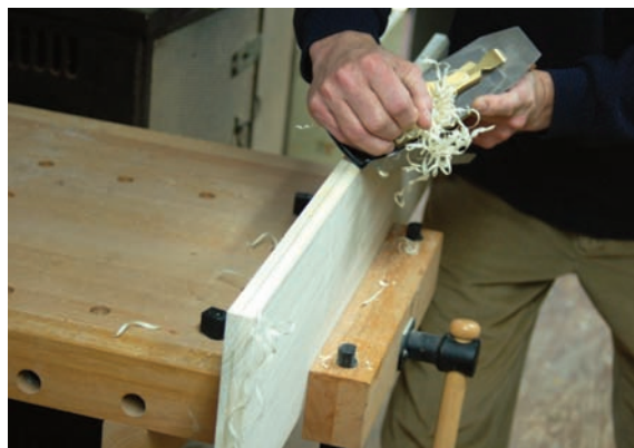
TOP The junction of the horizontal and vertical beads must be completed with a little paring-chisel work.
