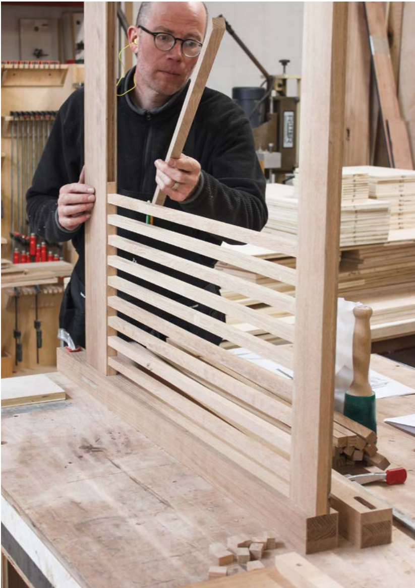
SPINDLES AND SPACERS IN PLACE. Glue the rails to one post, then begin alternating a spacer and a spindle in the grooves in the rails.
