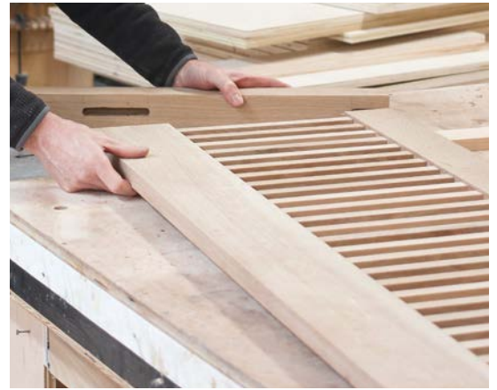
ADD A POST. Once you have all the spindles and spacers in place, glue on the second post.
