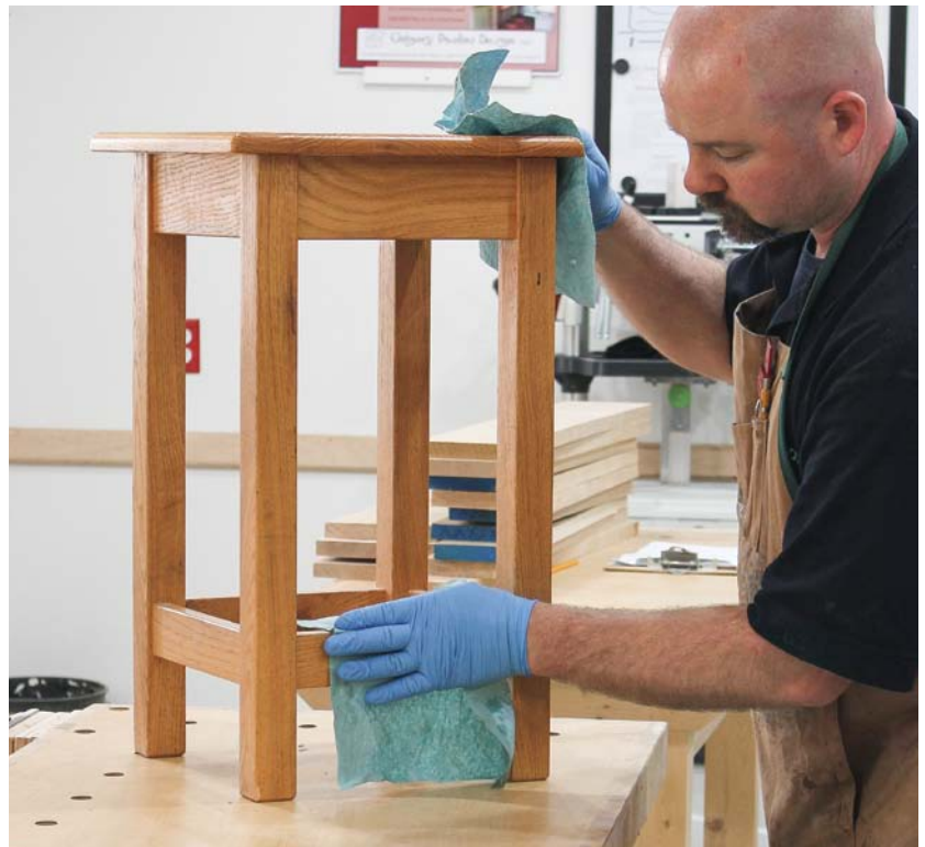
WIPE AND WIPE. I use two rags at a time to wipe off finish. The one in my left hand removes excess liquid, while the one in my right hand absorbs the residue. As the left-hand rag becomes saturated, I replace it with the rag from my right hand and get a clean rag for that hand.
