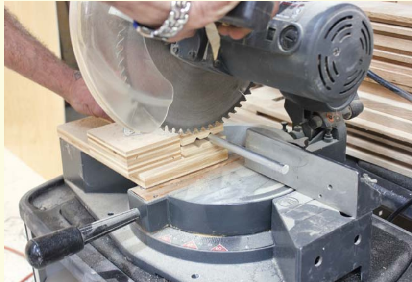
BAR STOCK HOLDER. Make a jig like this to secure the aluminum rod so that the force of the sawblade doesn't pick up and throw the metal.
