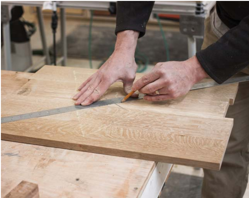
FIND THE CENTER. With a long ruler or straightedge, draw diagonals from corner to corner to find the center of the top piece.
