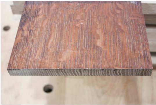
DYED OAK. Dyes color wood consistently and uniformly, regardless of the grain structure or porosity.
