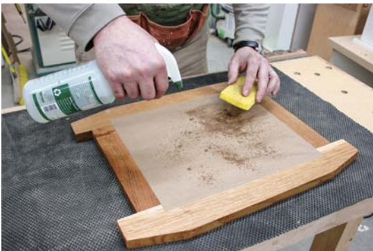
GIVE IT A SPRITZ. Spray the paper with a light mist of water. You want it to be only slightly damp, not soaked.
