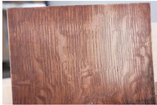
DON'T OVERDO THE SANDING. Scuff-sanding can produce a slight color variation, shown on the left side of the board. That's normal. Areas sanded through (right side of board), obviously need to be touched up with more dye.
