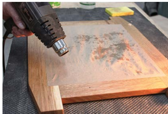
HEAT-SHRINK. A blast from a hair dryer or heat gun quickly dries the paper and shrinks it tight.
