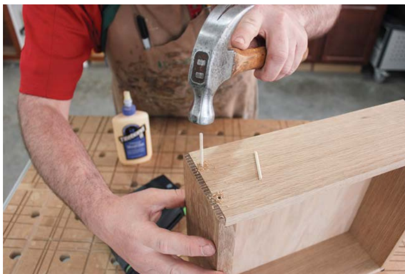
BRING IN REINFORCEMENTS. Drill holes in the drawer sides, then glue and tap in dowels to reinforce the rabbet joints. It's nice to use contrasting wood—lighter, as here, or darker.
