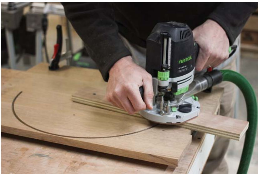
ROUND AND ROUND. Attach the trammel to the centerpoint and insert the router bushing into its hole. Then make a series of shallow cuts, moving the router counter-clockwise, to cut the circle.
