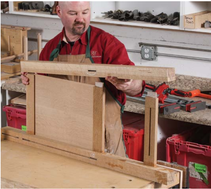
SIDES FIRST. Begin assembling the sideboard by gluing up the two side assemblies.
