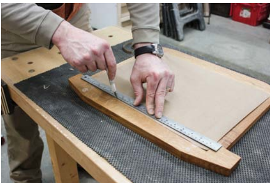
TRIM THE EDGES. Use a sharp razor knife and a straightedge to trim the paper.
