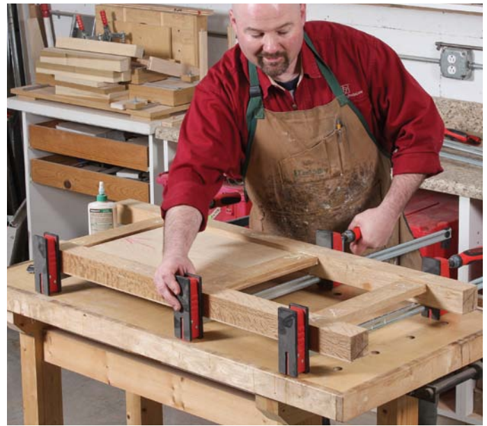
POSITION THE CLAMPS. Center the clamps over the stretchers. Be sure to check everything for square.
