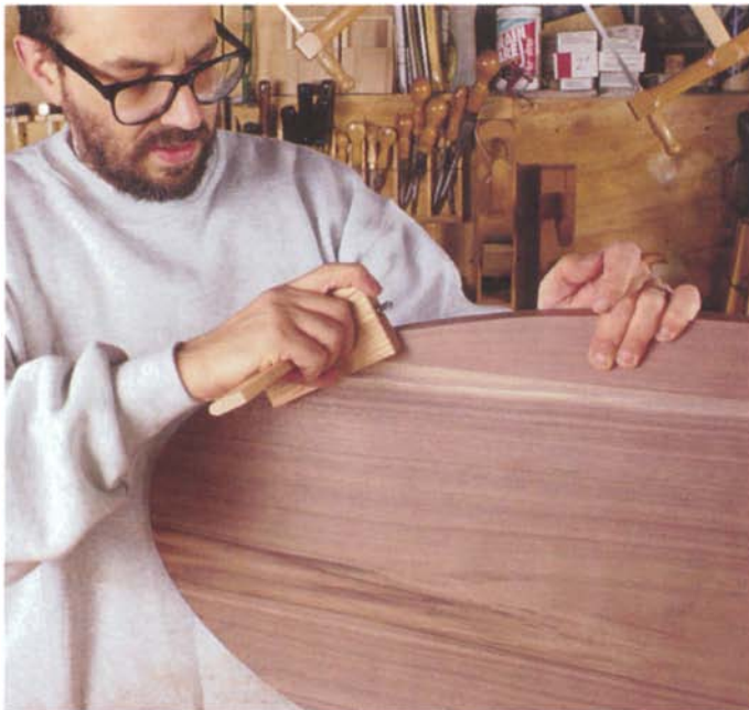
Photo D: Registering a marking gauge against the top face of the tabletop, mark a line on the edge of the top to define the outer edge of the chamfer.
