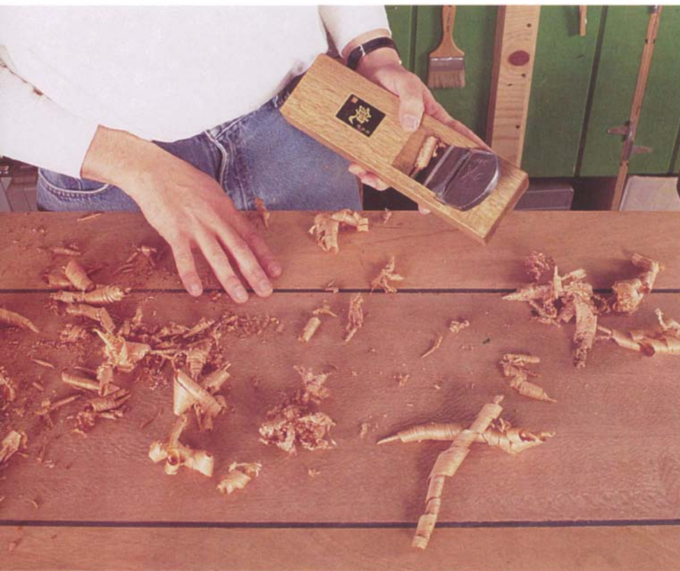
Photo C: Use a smoothing plane to level the frame to the panel. To prevent planing through the thin veneer, use a sharp scraper for your final passes.
