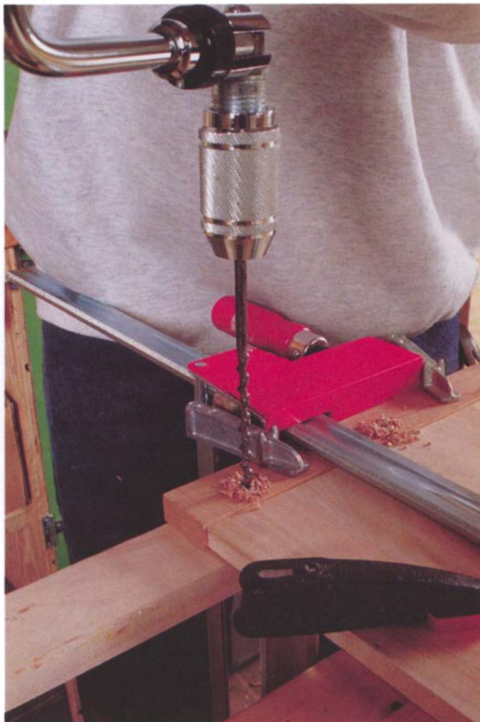
Photo C: Dry-clamp the breadboard end onto the plank, then drill the dowel holes. The backer block clamped to the underside prevents exit tearout.
