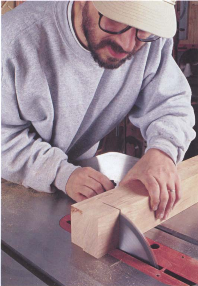
Photo F: After ripping and jointing the leg blanks to thickness, crosscut them to length.
