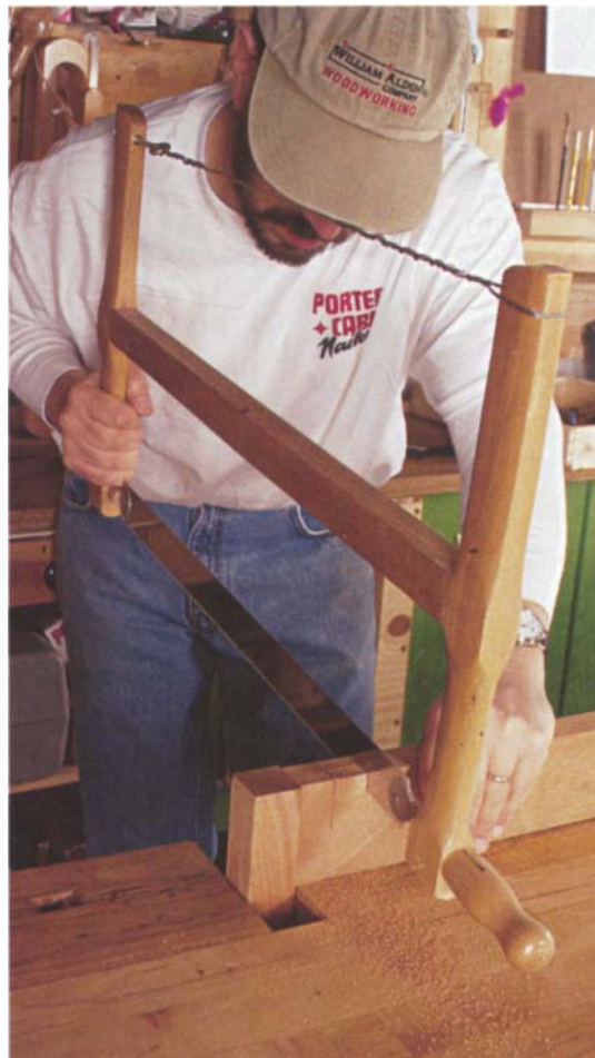
Photo J: After gluing up the long apron and leg assemblies, cut the half-lap notches in all of the aprons.
