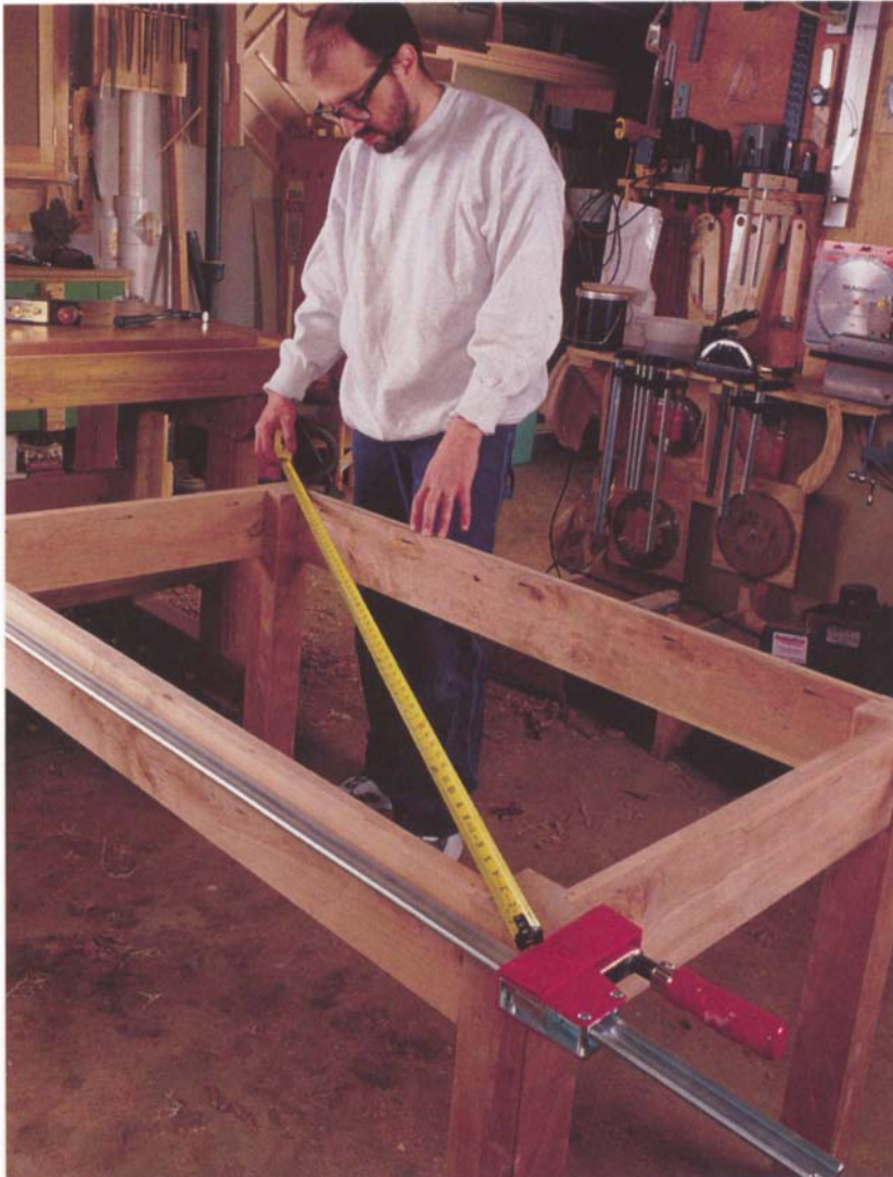
Photo L: After gluing the end assemblies to the long aprons, check the table for square by comparing the diagonals across the top.
