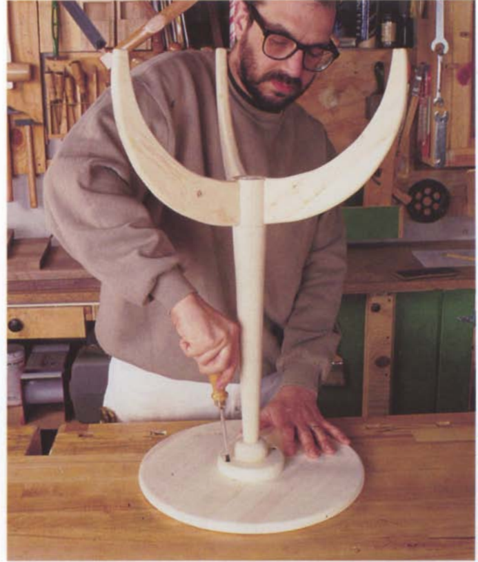
Photo M: Attach the top with two 1-in.-long screws driven through the mounting ring. Orient the screws diagonally to the grain of the top to prevent wood movement problems.
