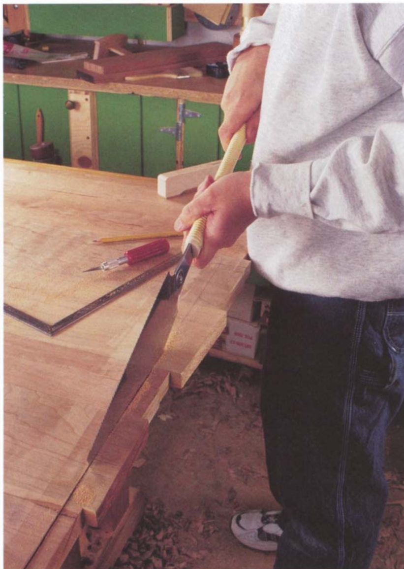
Photo B: Because the tabletop is too large to crosscut on the table saw, it must be cut to length with a handsaw or portable circular saw. I use a Japanese ryoba saw.
