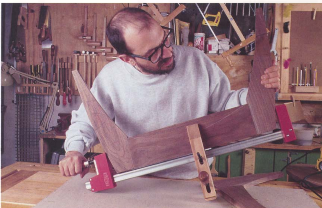
Photo G: I clamp two legs to each rail using a deep-throat bar clamp. A handscrew clamped to the rail prevents the bar clamp from sliding off the curves of the legs.
