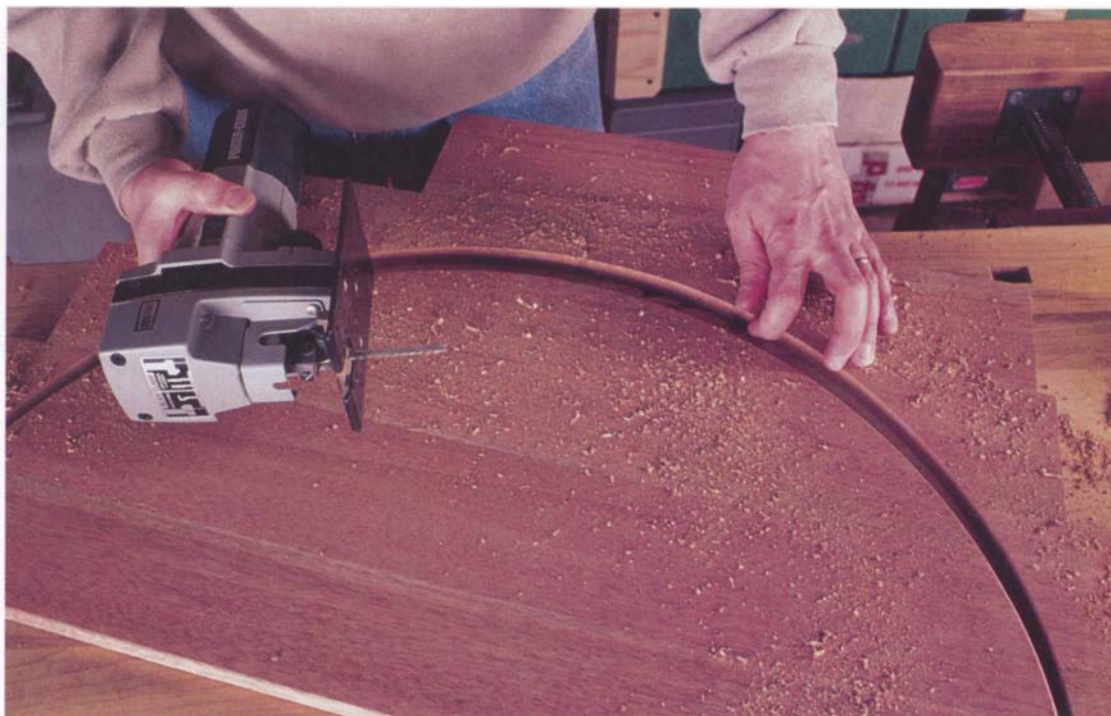
Photo A: Use a jigsaw to cut the half-round top from the blank.
