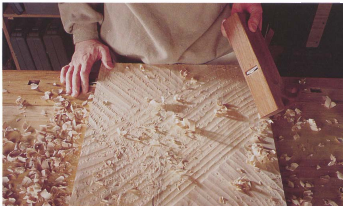
Photo A: Begin flattening the blank for the top by planing diagonally with a scrub plane to remove the high spots.
