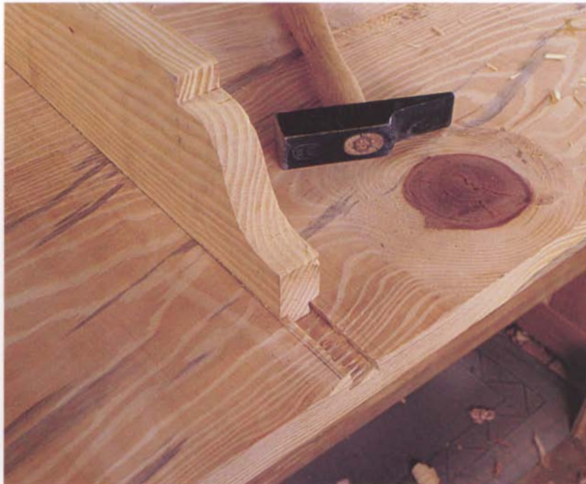
Photo D: When the dovetail is fairly snug along its length and is sitting a couple of inches from the end of the slot, it's ready to be glued and tapped home.
