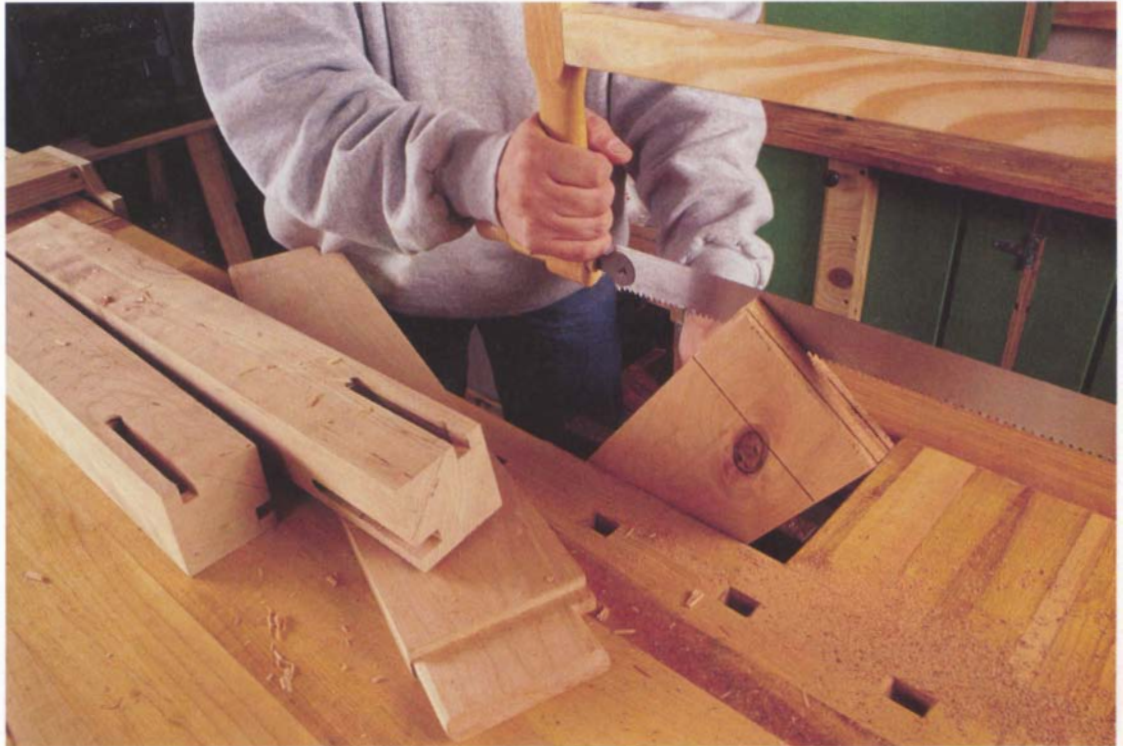
Photo H: I use a bowsaw to cut the apron tenons. I start by cutting the waste diagonally from opposing corners, then finish up by sawing straight downward toward the tenon shoulder.
