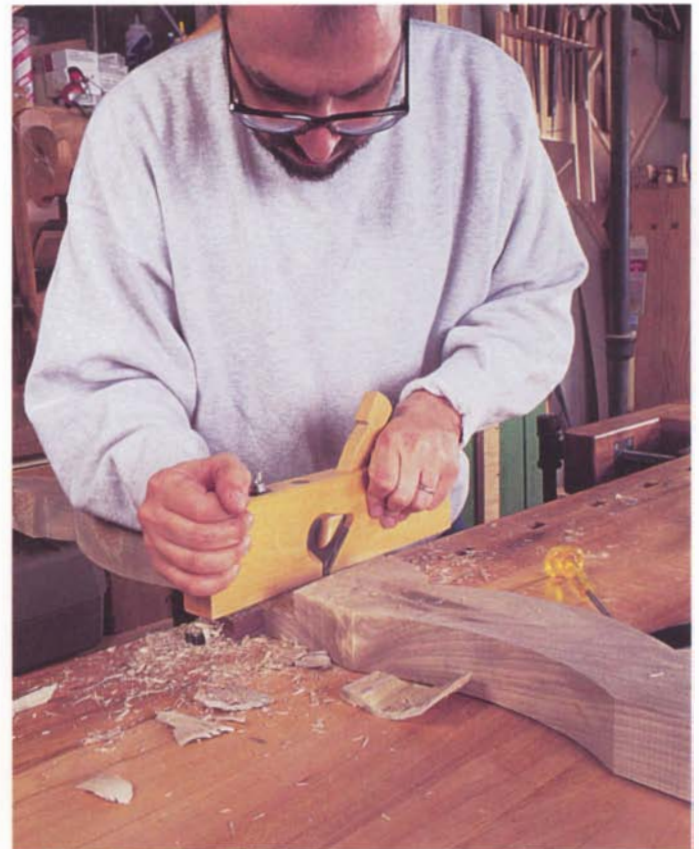
Photo H: Do the final cleaning of the notch bottom with a rabbet plane.
