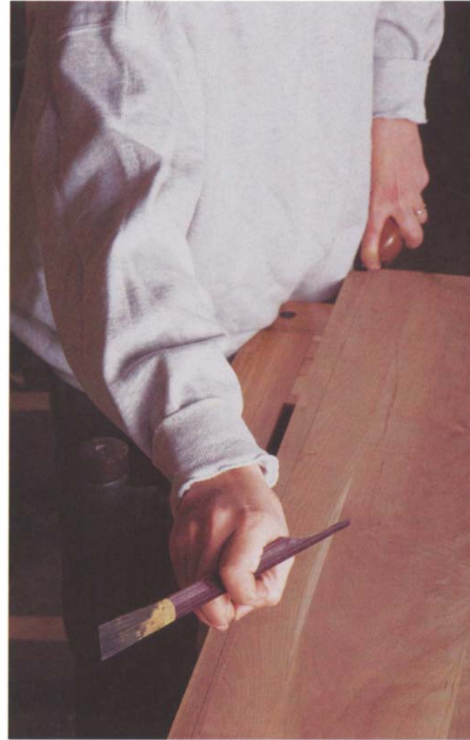
Photo A: I snap a Japanese ink line along the edge of the tabletop to establish a cut line for ripping the edge.
