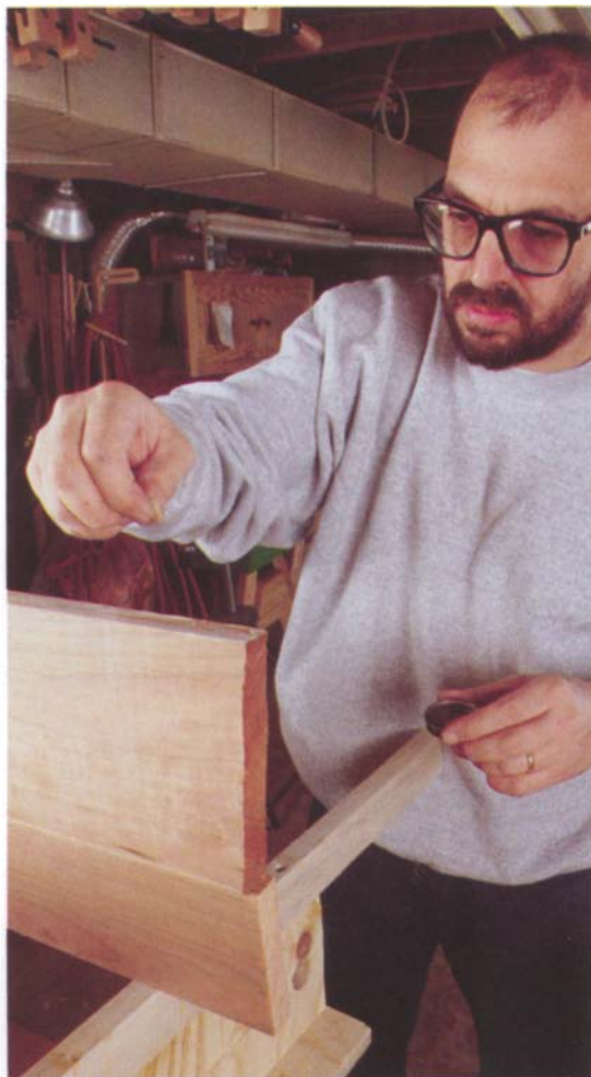
Photo B: A few grains of sand sprinkled into the glue at the ends and center of an edge joint prevent the boards from slipping out of alignment under clamp pressure.
