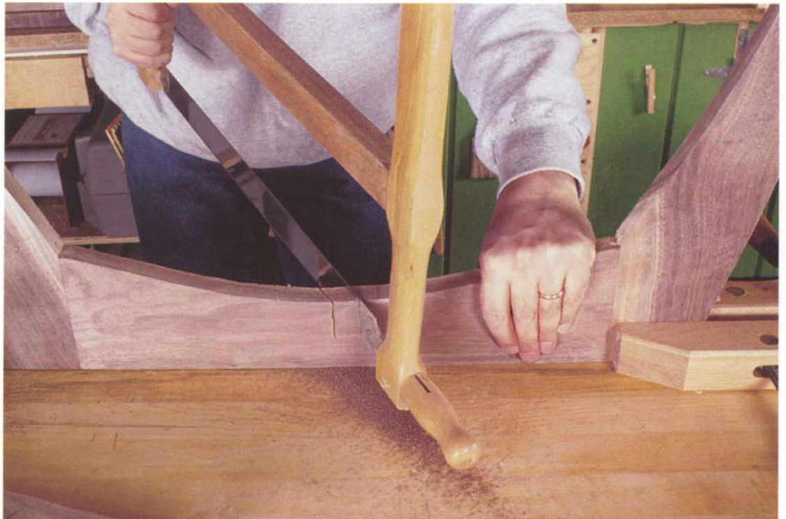
Photo J: To cut the notch, first saw the shoulders, then chisel out the waste to the finished depth of the notch.
