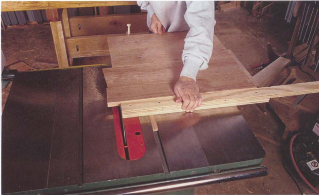
Photo C: A shop-made panel-cutting jig helps you squarely crosscut wide stock, such as the tabletop. The body of the jig is guided by a strip of wood that rides in the table saw's miter gauge slot.
