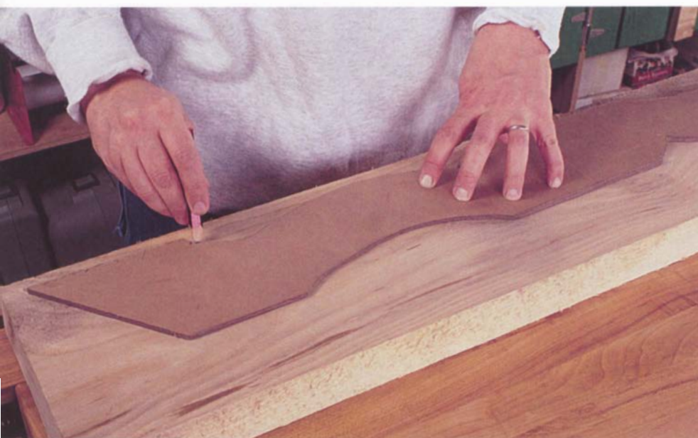
Photo E: Trace the profile of the leg onto its blank using a template.
