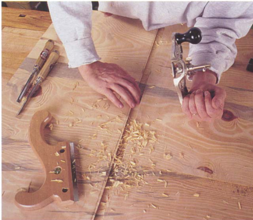
Photo A: After sawing the walls of the tapered dovetail slot, chisel out most of the waste, and then level the bottom of the slot with a router plane.
