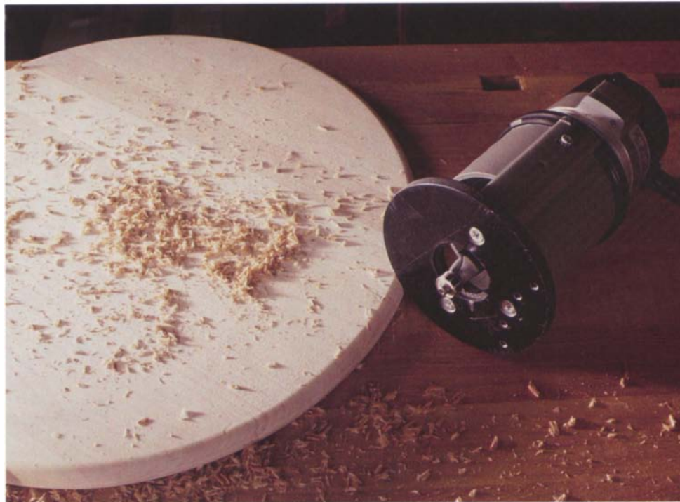
Photo D: Rout both edges of the top using a \frac{1}{4} -in.-radius roundover bit.
