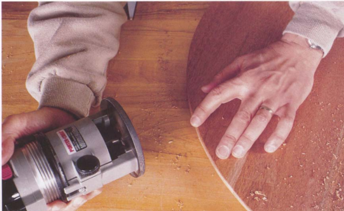
Photo B: After routing the chamfer on the underside of the top, use a \frac{1}{8} -in. roundover bit on the top side.
