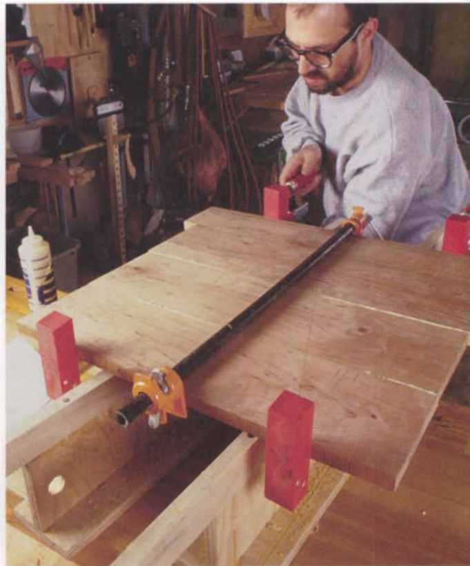
Photo B: Clamping stands allow easy access to the clamps when edge joining boards. The weight of the clamps on the top also helps pull the panel flat.
