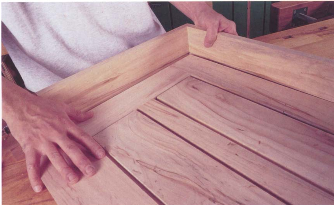
Photo H: Dry-fit the bottom into the grooves in the drawer front, back, and sides to check the fit before gluing up the drawer.
