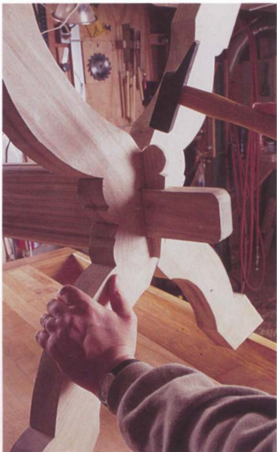
Photo K: Assemble the trestles and the beam by tapping the tusk tenon wedges into place.
