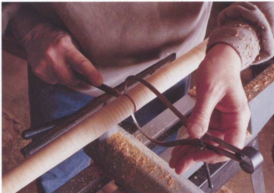
Photo E: Cut a 1-in.-diameter groove 11 in. up from the foot to establish a midpoint reference for turning the leg's taper.
