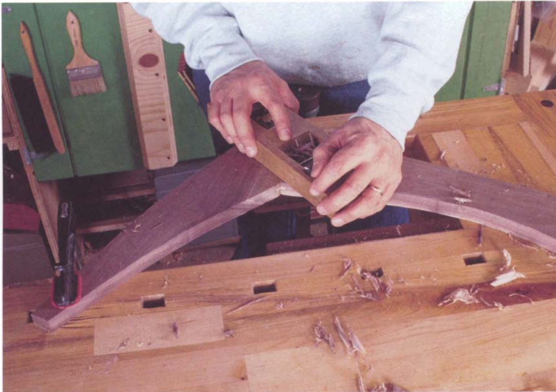
Photo H: Plane or sand the leg-to-rail joint faces smooth.
