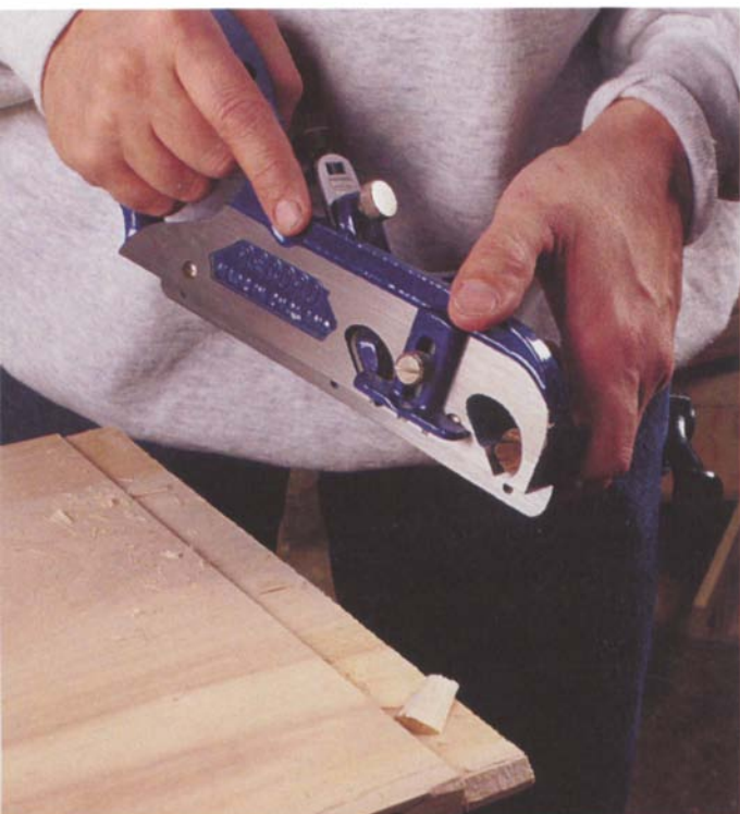
Photo B: After sawing the shoulder at the edge of the plank, cut the tongue with a fillister plane. Planing the tongue, rather than sawing or routing it, allows you to fine-tune its thickness for a perfect fit in its breadboard end groove.
