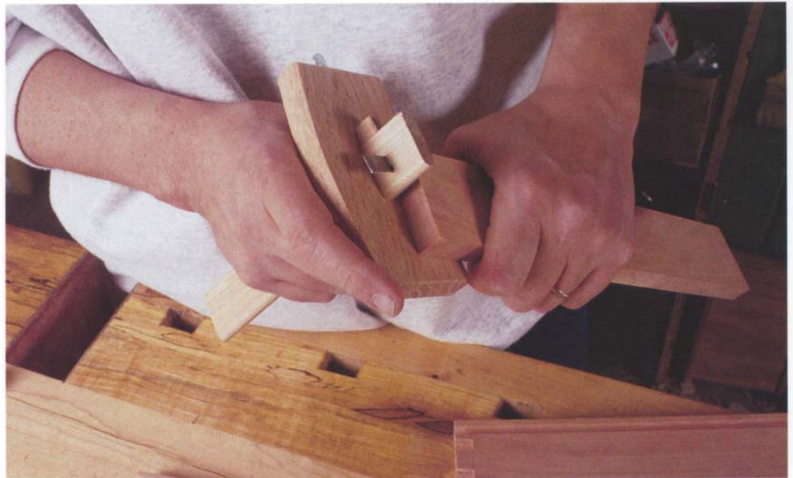
Photo F: Use a marking gauge to scribe a line that defines the length of the half-blind dovetails in the drawer fronts.
