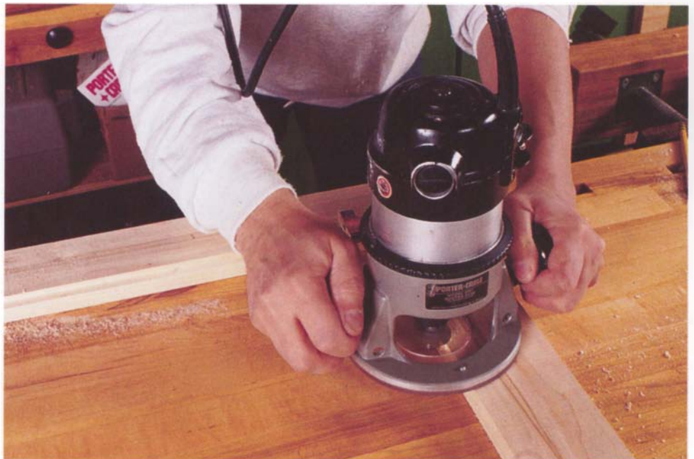
Photo A: Rout the rabbet for the glass top, moving the router clockwise inside the frame.
