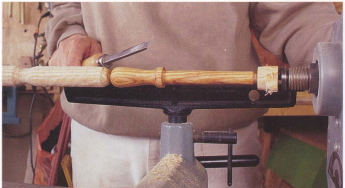
Photo J: Use a skew chisel to turn the slight taper on the batten pins.
