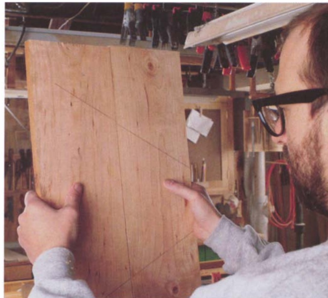
Photo A: I "spring" the joint by handplaning a slight concavity into the edge of each tabletop board. The resulting \frac{1}{4} -in. gap at the center ensures that the joint is first and foremost tight at its ends.
