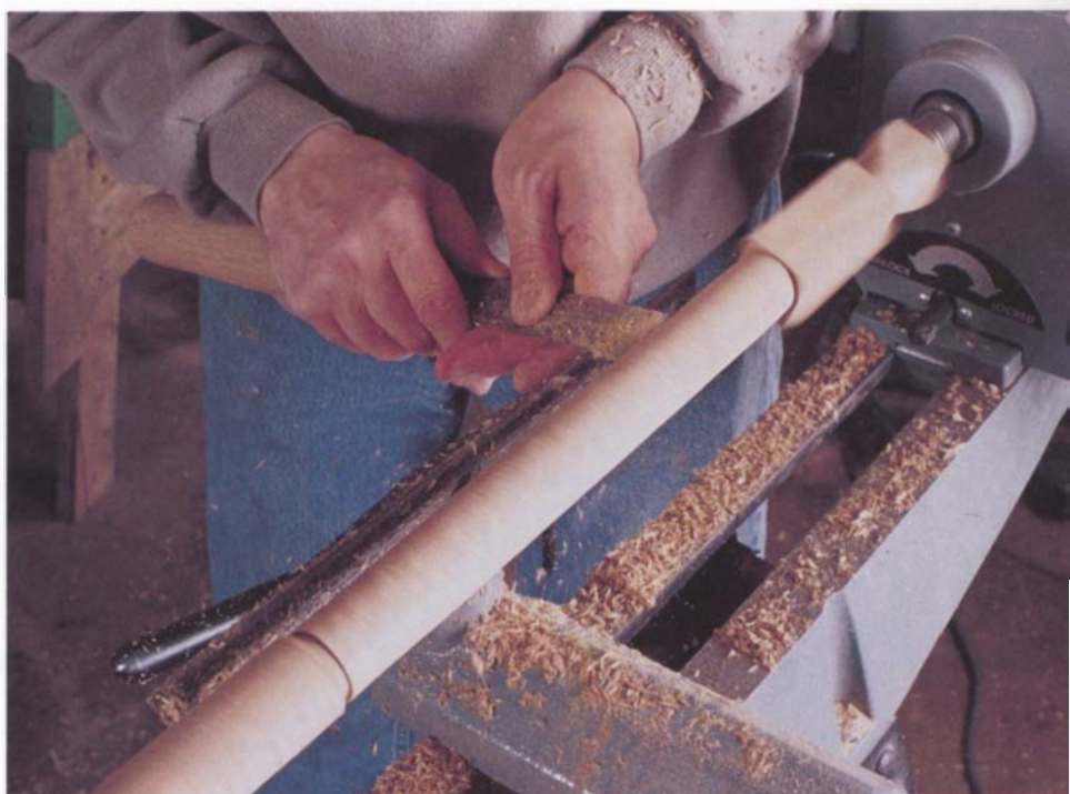
Photo F: Turn the taper with a skew chisel. Use calipers to check the 1\frac{1}{16} -in. diameter at the top of the taper and the \frac{3}{4} -in. diameter at the foot.
