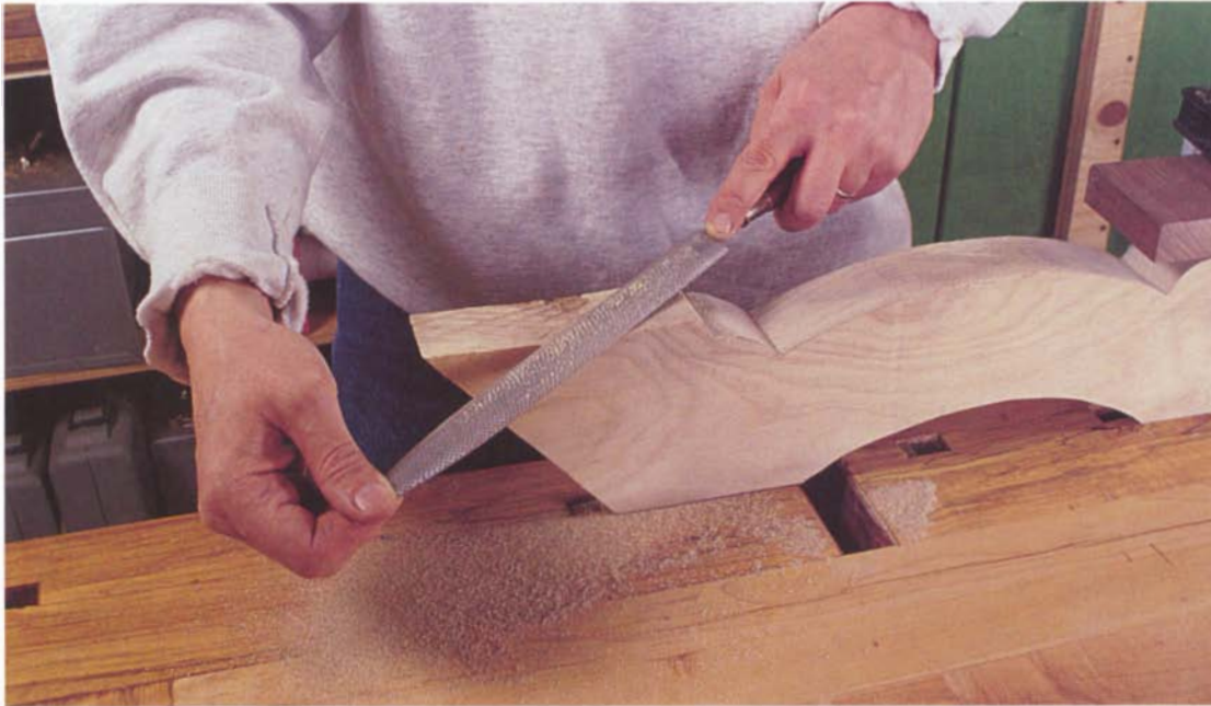
Photo F: Clean up the bandsaw marks on the leg pieces using files, rasps, and spokeshaves.
