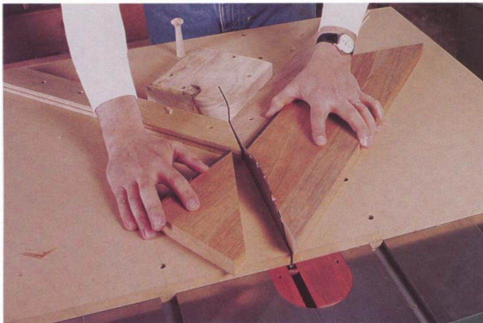
Photo A: A table saw miter sled makes quick, accurate work of sawing the miters for the top and shelf frames.
