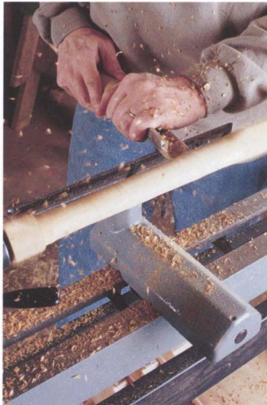
Photo D: Begin shaping the leg by turning it to a cylinder with a roughing gouge.
