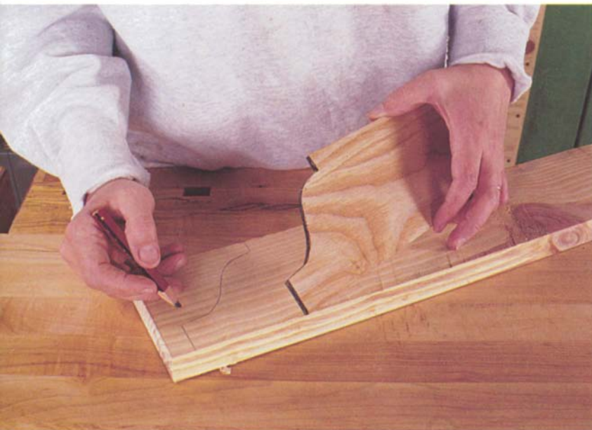
Photo B: Lay out the ogee on the end of each batten using a template made from "Batten Pattern."
