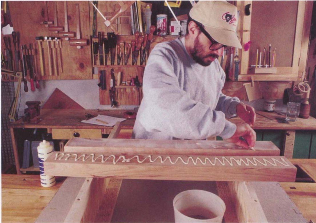
Photo D: If you can't find 3-in.-thick stock to make the legs, laminate two pieces of thinner material together.
