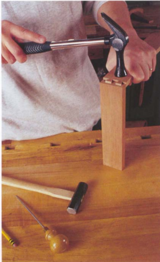
Photo K: Test the fit of the joint by lightly tapping the tails into the sockets.
