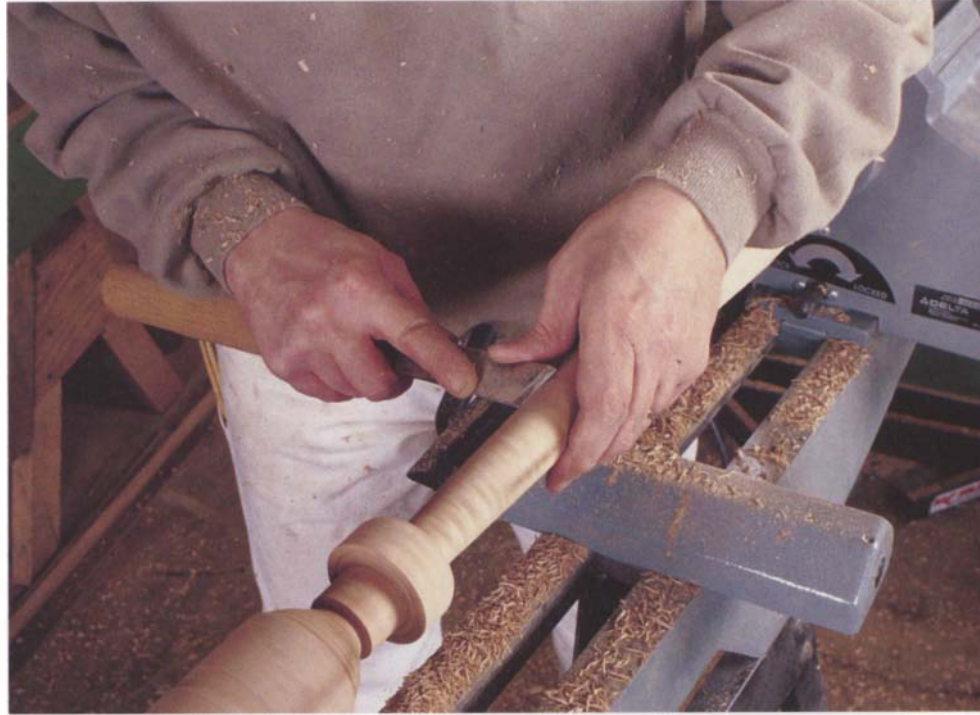
Photo F: After roughing out the taper with a gouge, smooth it with a skew chisel.
