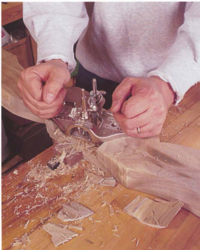
Photo G: After sawing the shoulders of the leg notches and removing most of the waste with a chisel, flatten the bottom of the notch using a router plane.
