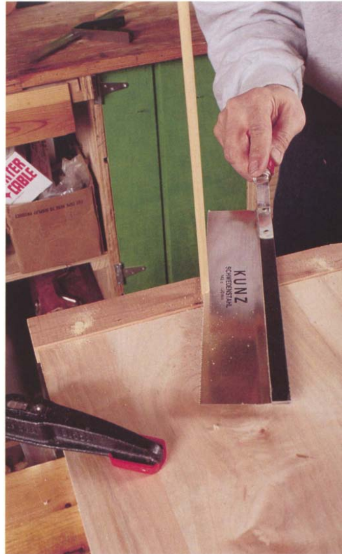
Photo E: Pin the unglued breadboard ends to the plank with dowels sparingly glued into their holes. Trim them flush after the glue dries.
