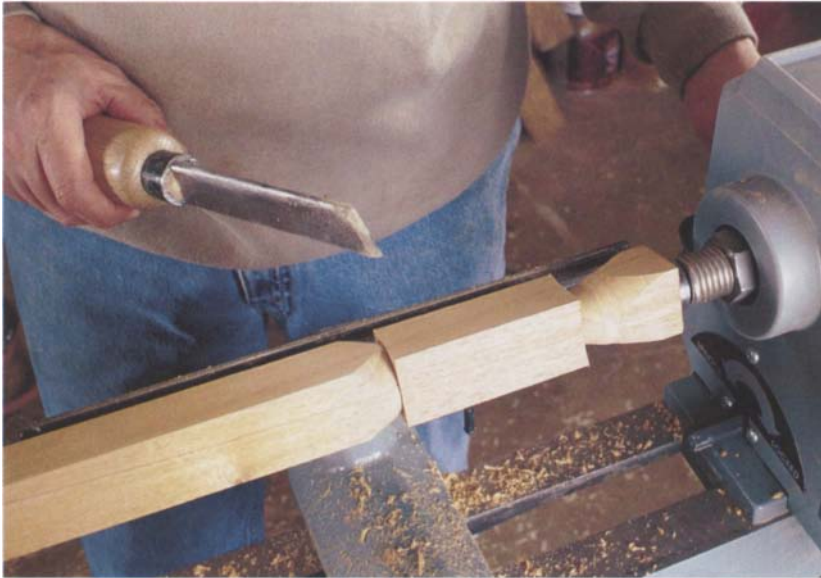
Photo C: Using a skew chisel, make a cut 3\frac{1}{2} in. down from the top of the leg to cleanly define the bottom of the square section.
