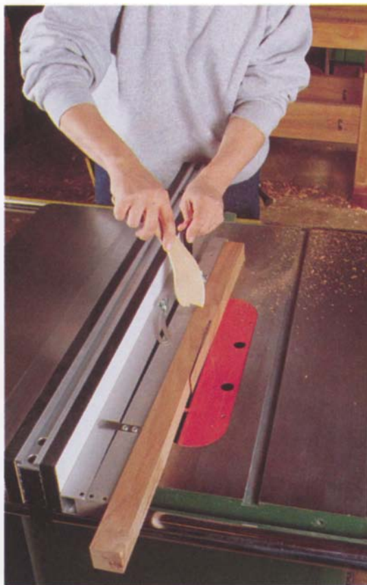
Photo C: I use a commercial tapering jig to saw the taper on the legs.
