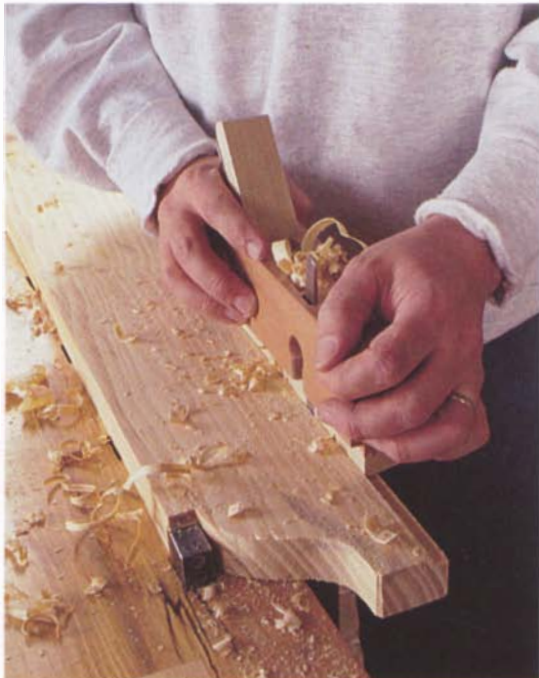
Photo C: Using a dovetail plane, cut the tapered dovetail on each batten. Begin at the narrow end of the taper, taking short strokes and working toward the wider end.
