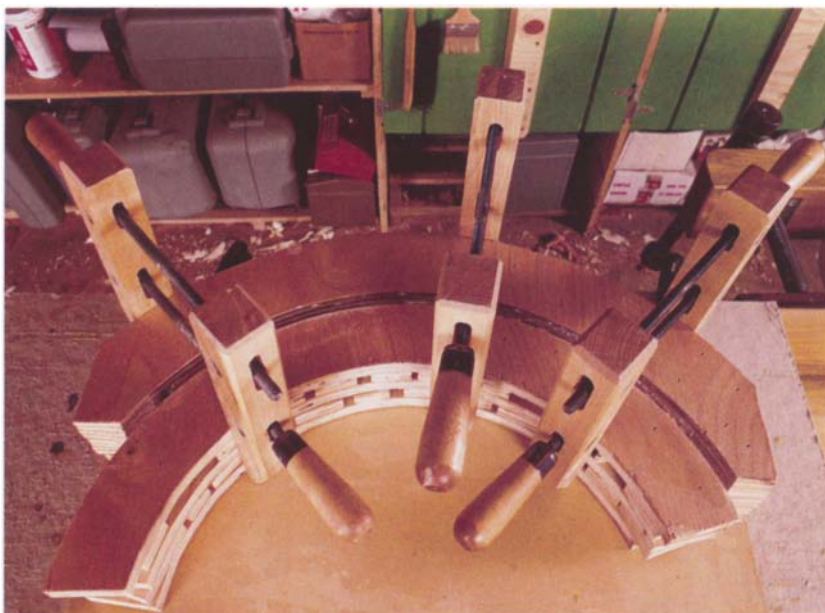
Photo I: Clamp with handscrews alongside the bar clamps because of their wide bearing surface. Then remove the bar clamps.
