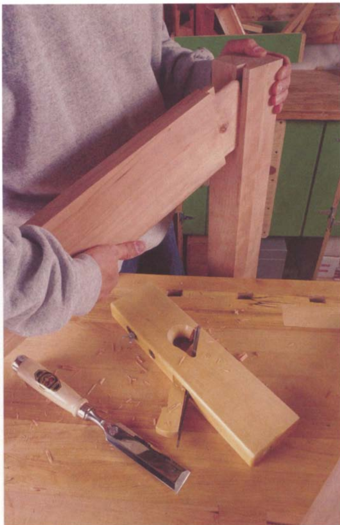
Photo J: In preparation for glue-up, check the fit of the mortise-and-tenon joints, trimming them as necessary to ensure a good fit.
