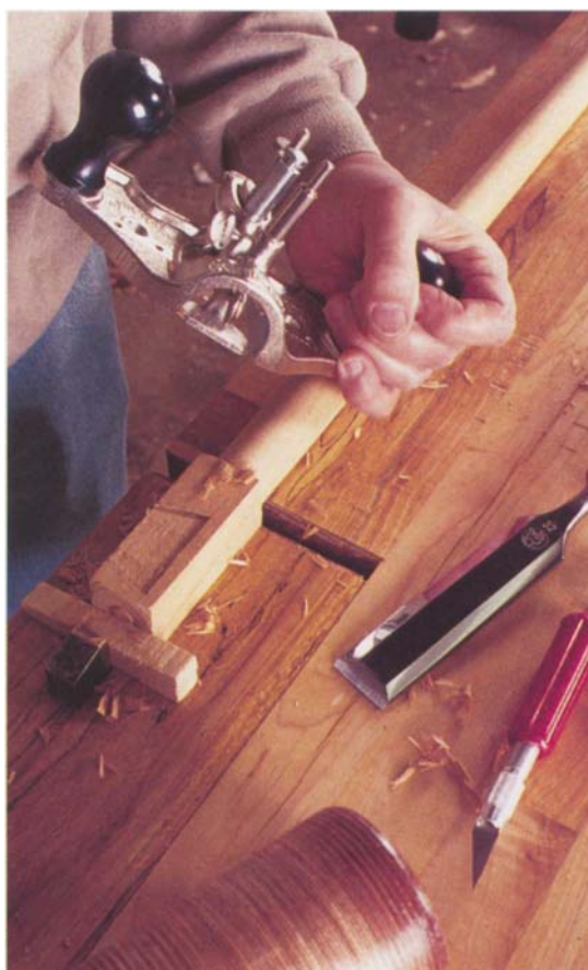
Photo K: I use a chisel and router plane to cut the socket in the rear legs for the half-lap dovetail on the rear rail.
