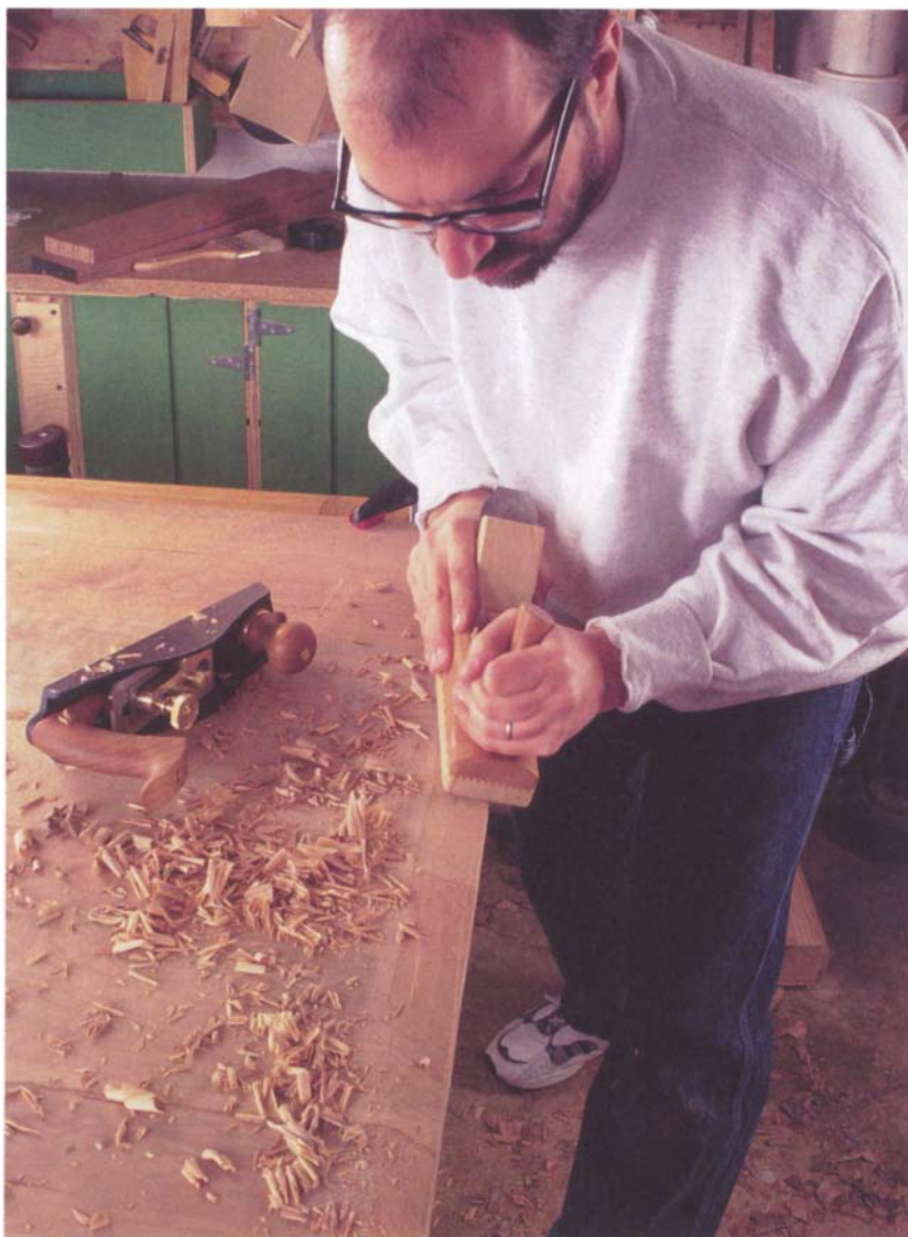
Photo C: Use a smoothing plane to create the bevel on the tabletop. Begin by taking moderately heavy cuts, then adjust the plane iron for a very light cut as you approach the bevel layout lines on the top and sides of the plank.
