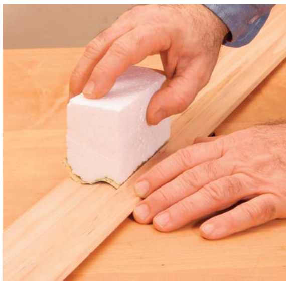
Improvise a curved sanding block to conform to concave shapes. You can easily shape foam packing material to match moldings.
