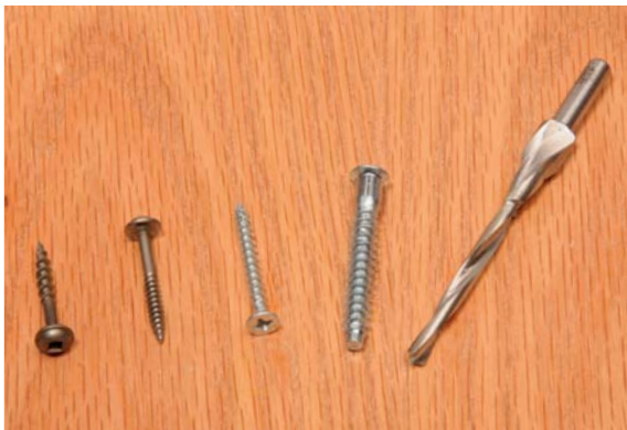
Here's an assortment of special screws you'll find helpful (from left): a pocket hole screw for softwood, one for hardwood, the deep-thread Spax design, a Confirmat screw and its special bit.
