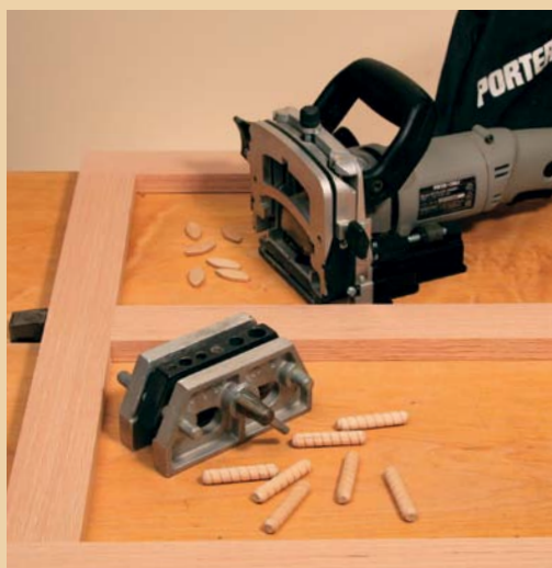
Dowels are an old standby of face-frame construction, and biscuits also make sturdy joints.
