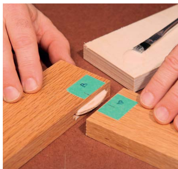
A biscuit joint is strong, invisible, and easy to make.
