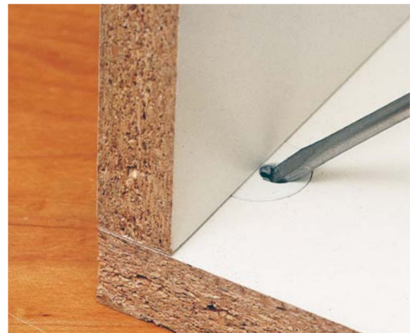
Knockdown corner fittings are easy to install and provide very good joint strength.
