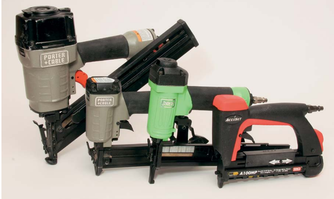
Four pneumatic drivers will speed the assembly and installation of your built-in. From left: a finish nailer with an angled magazine for easy access in tight quarters, a brad driver, a narrow-crown stapler, and a headless pinner.
