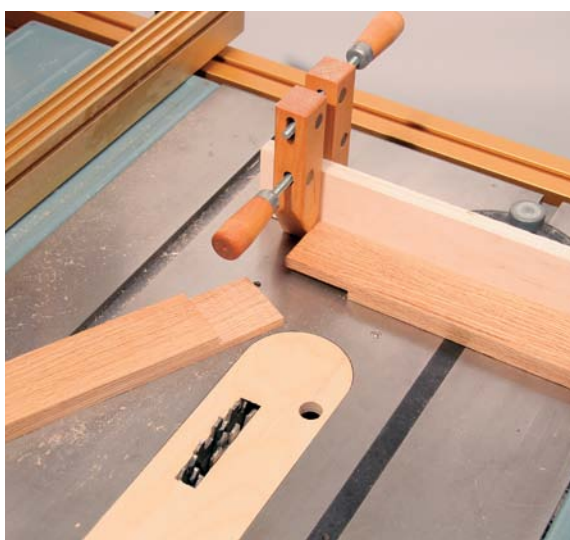
You can machine half-lap joints with a single setup on your tablesaw.
