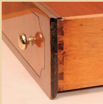
This vintage drawer features a one-piece front joined to the sides with half-blind dovetails.
