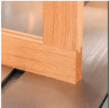
You can machine a stub mortise and tenon joint with a dado head in your tablesaw or with a table-mounted router.
