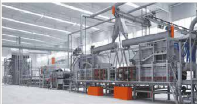
Particleboard Production Line
