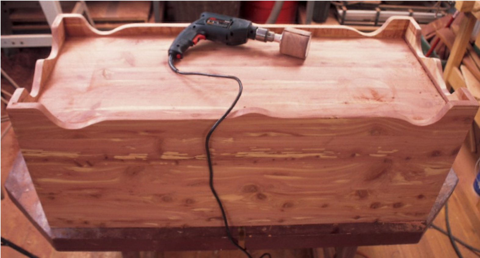
STEP 16 Use a sanding drum attached to a hand drill to smooth the curved edges of the box.
