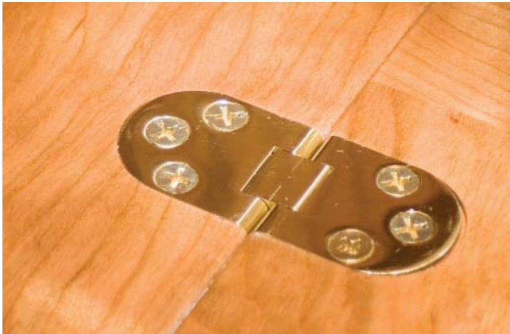
STEP 34 When the desk is opened, your eye is immediately drawn to the bright brass hinges, so make them a good fit. The drop-front desktop and the shelf it's hinged to need to be flush when the desktop is open. The butler tray hinges look good and work perfectly. The installation of the hinges is just like the butt hinge installation. Install the hinges on the desktop first, then attach them to the shelf.
