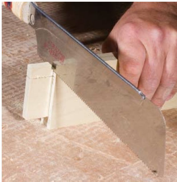
STEP 4 The band saw is great for cutting the tenon offset. Complete the offset by cutting the scrap away with a hand saw.
