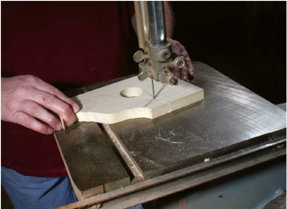
STEP 24 Cut the profiles using a band saw, then sand the edges smooth.
