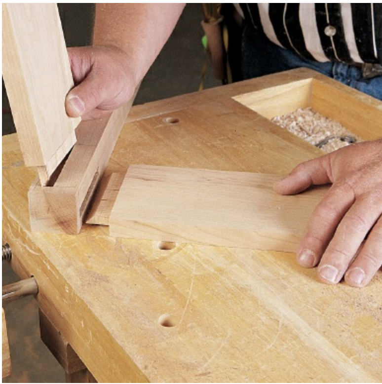
When you have to use mitered mortise-and-tenon joinery, don't get too worked up about the fit of the miter. You don't want the miter too tight.
