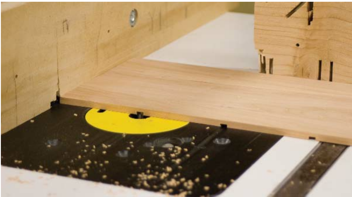
STEP 37 I cut the dados for the vertical cubby hole dividers using a router table. The table saw will work equally as well.
