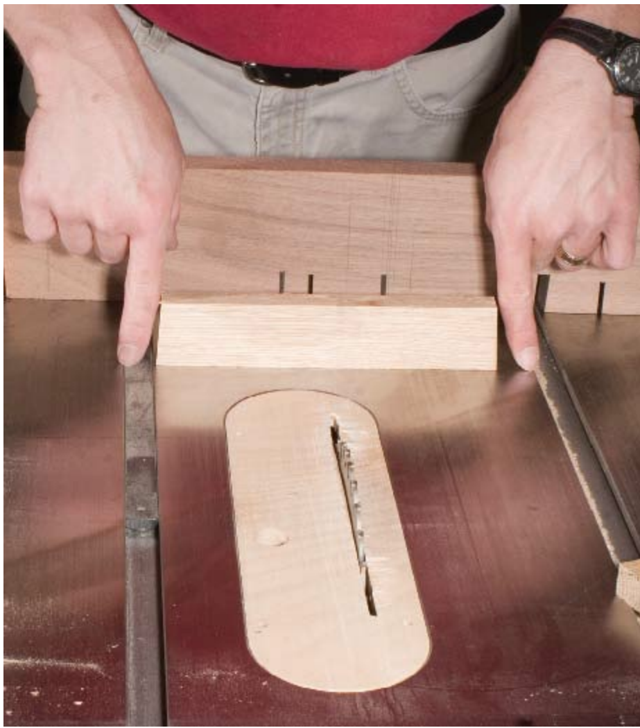
STEP 4 The rails will have opposite angles and the stiles will have parallel angles. I'm showing exaggerated opposite angles on the rails using my fingers.
