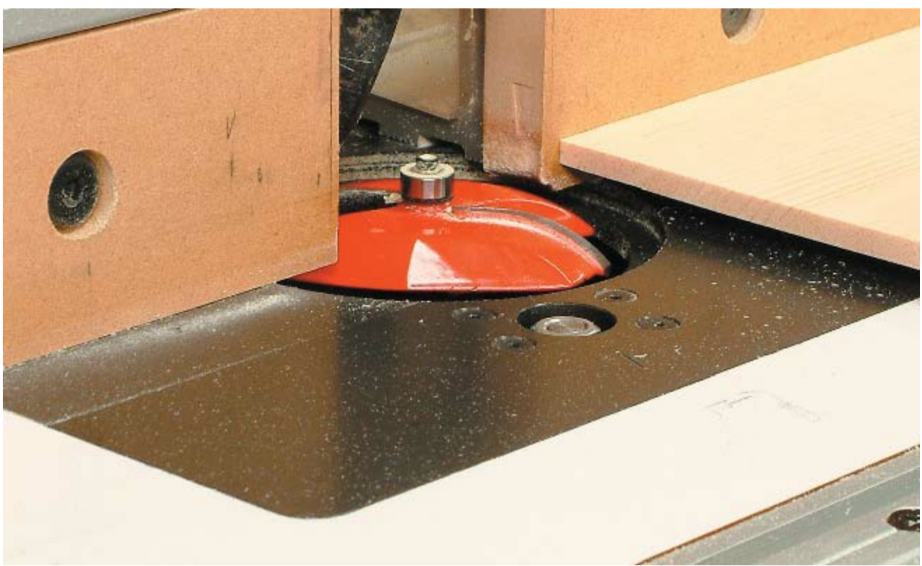
STEP 10 Use the router to cut the cove on the door panels. You could also raise the panels by cutting a 12° bevel on the panel edges.
