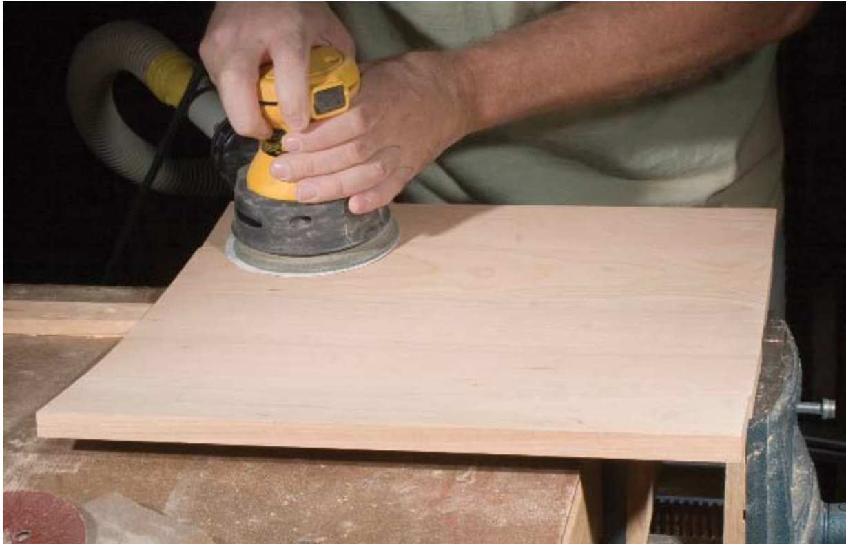
STEP 24 Use a curved scraper to roughout the curve on the inside of the panel. Finish up with the random orbital sander.
