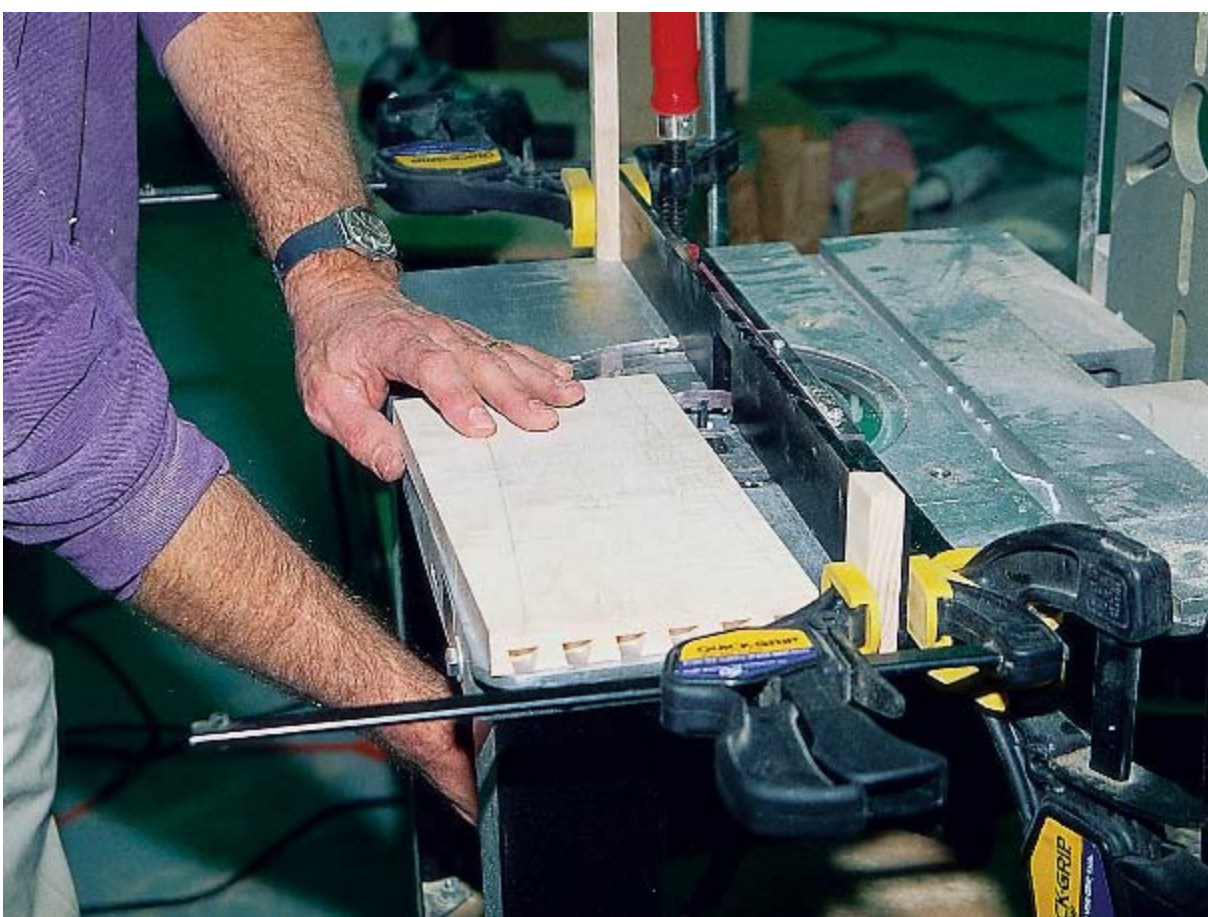
A stopped groove was required on the inside of the drawer front to receive the bottom. It was cut with a router.
