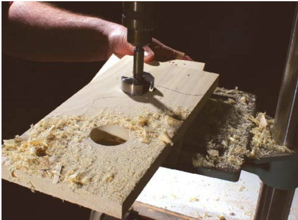
STEP 23 Use a 1 3/4" Forstner bit to cut holes in the feet. These holes will form the spur of the foot.
