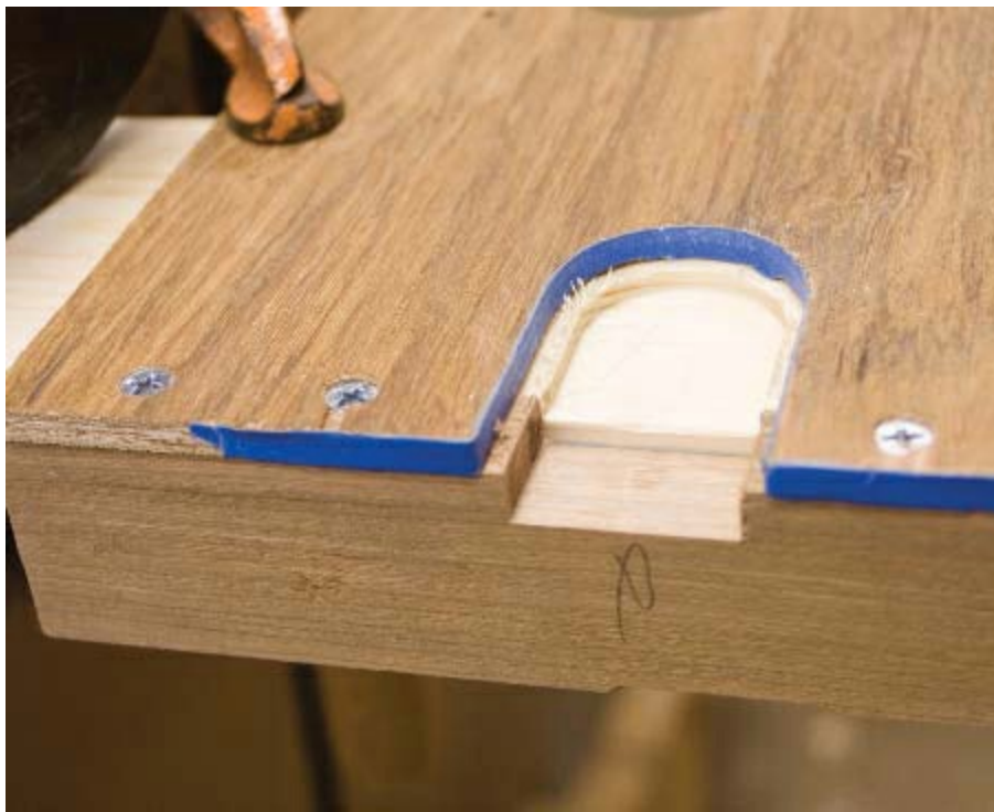
STEP 33 I made a jig for cutting the mortises for the drop-leaf desktop. Note the blue tape used to fine tune the fit of the mortise to the hinge plate exactly.
