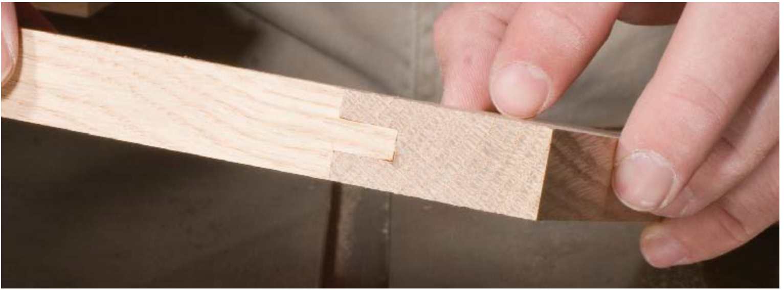
STEP 12 The tops of the stiles will be visible when the wastebasket is finished. Fit the end of the tenons so they bottom out in the grooves. It's not necessary to leave a space for glue.
