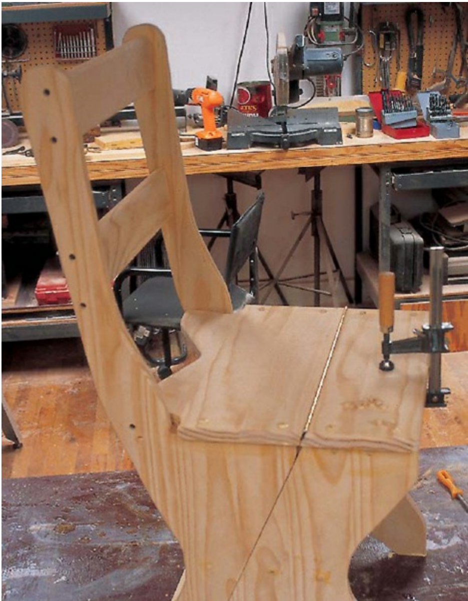
STEP 12 After cutting the seat to shape, separate the front and back parts. Then attach the continuous hinge to the parts. The bevels on the hinged edges of the seat should match the
