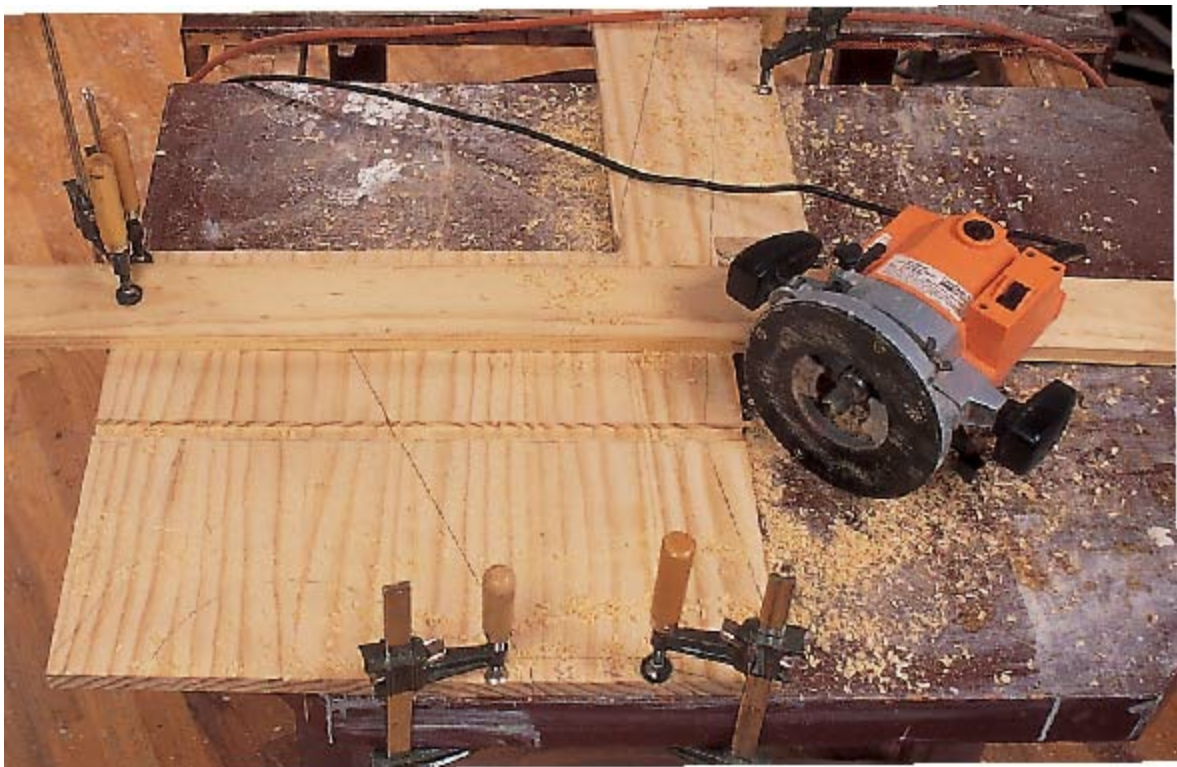
STEP 4 Glue the final wing piece on the long back edges of the sides. Then, using a straightedge and a router, cut a \frac{1}{4} "-deep by \frac{3}{4} "-wide dado in the sides for the front and back steps. Be sure to make right and left sides.
