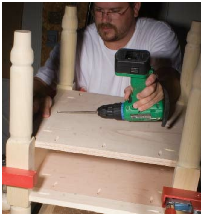
STEP 10 Attach the bottom of the drawer box and two edging rails to the table base using the same method shown in steps 8 and 9.
