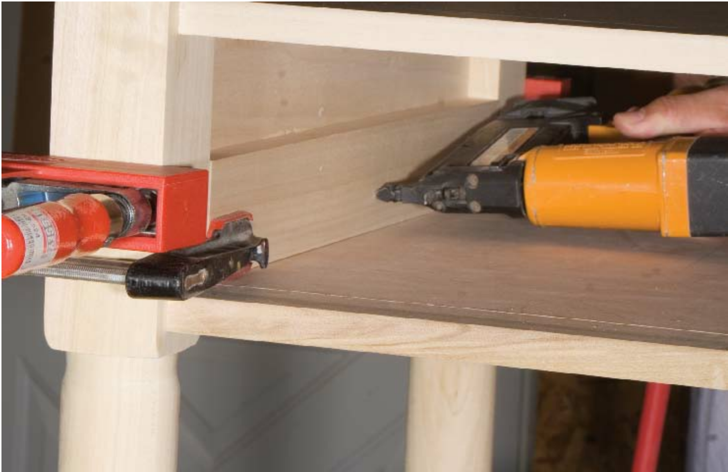
STEP 11 Attach the drawer guides using glue and nails. Note that the guide is about \frac{1}{16} " proud of the inside faces of the legs. This will keep the drawer fronts from hitting the legs.
