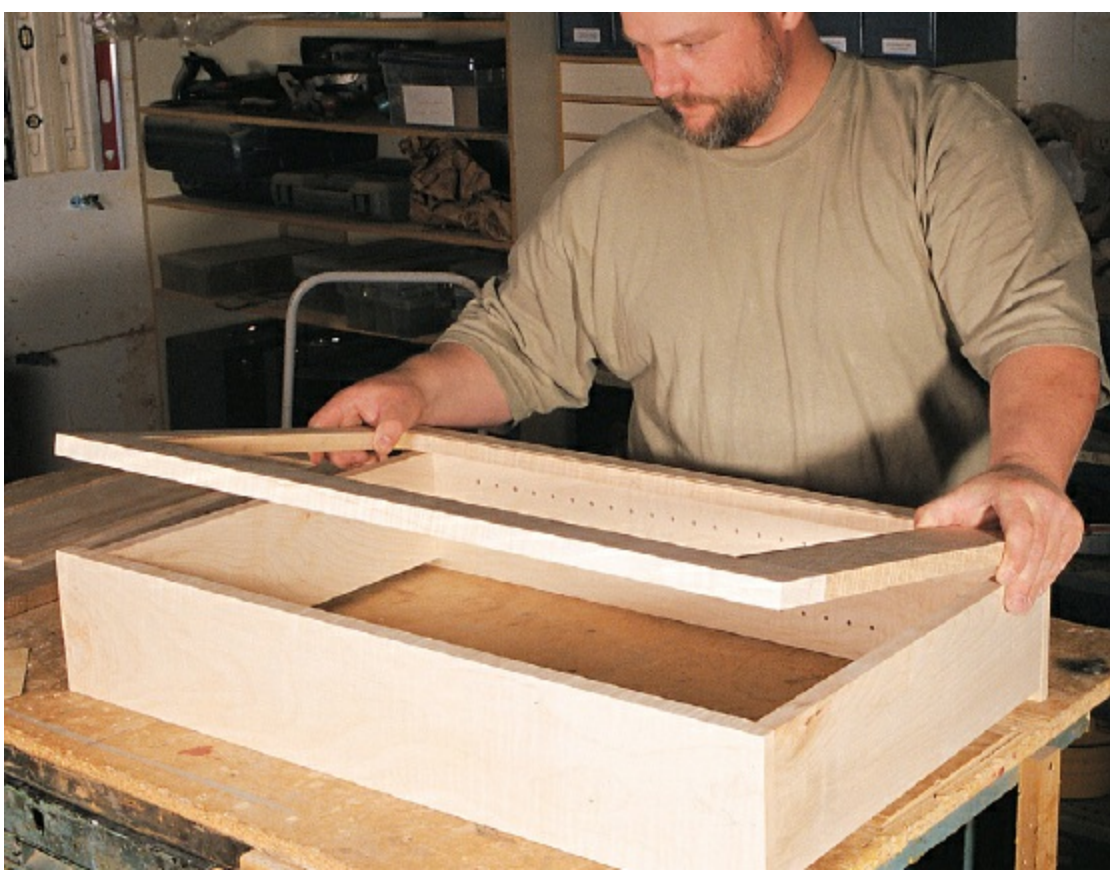
Fit the face frame on the case. The stiles should hang \frac{1}{8} " over the edge of the case so you can rout (or plane) them flush later.
