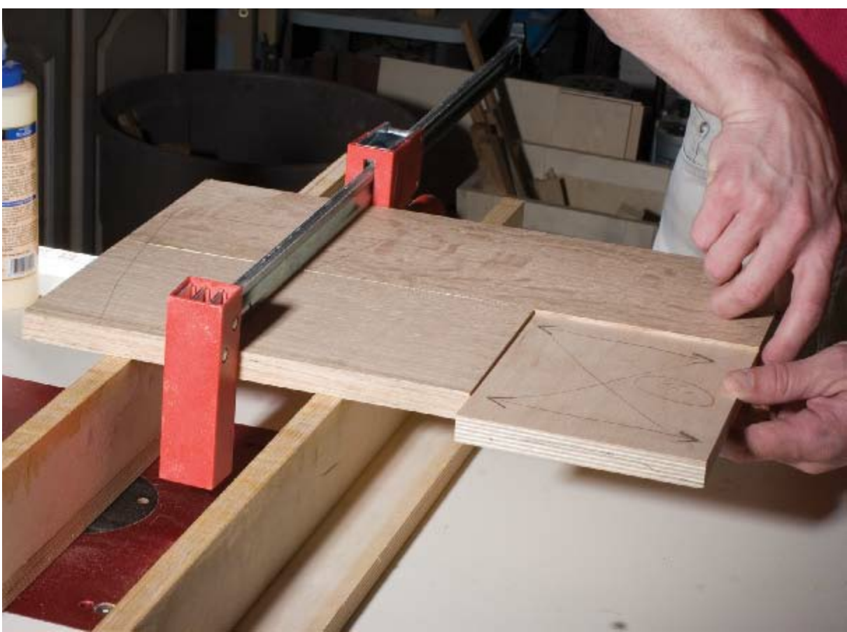
STEP 4 I found it easiest to glue up the sides two boards at a time using a spacer cut to step height.
