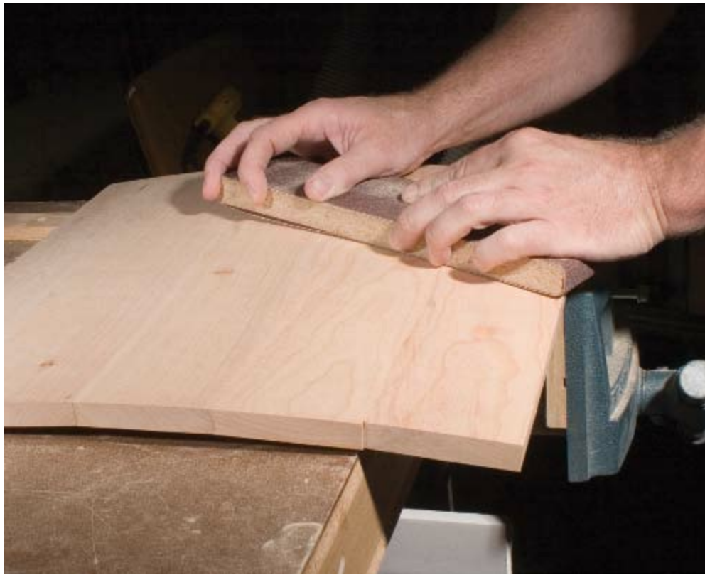
STEP 23 This is the best way to true the curve: use an 80-grit sanding belt wrapped around a wood block and sand across the wood grain. Then use a random orbital sander to clean it up.
