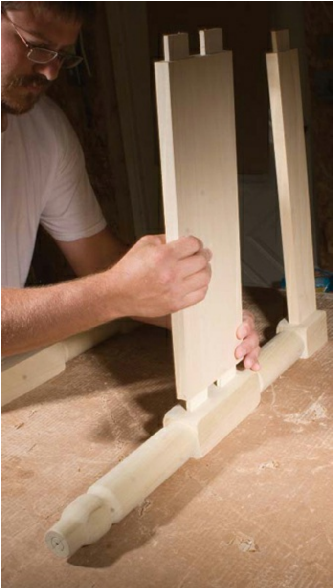
STEP 5 When the mortises and tenons have been cut and dry fitted, assemble the two sides of the base.
