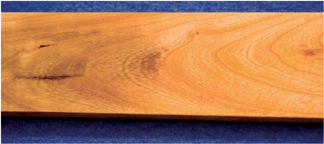
STEP 39 After finish-sanding the entire project, I used a paintbrush to apply ammonia to the raw wood. (The left side of the wood sample in the photo shows how the ammonia affects the cherry.) After the ammonia dried, I sanded the raised grain and applied a coat of catalyzed lacquer. When the lacquer was dry, I sanded the finish using 220-grit sandpaper. I applied two additional coats of lacquer and allowed them to cure for one week, then used No.0000 steel wool to rub the finish. To make the finish a little shinier, I applied a coat of wax.
