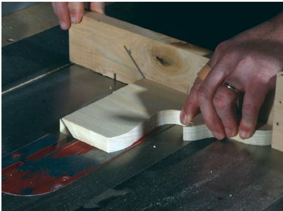
STEP 25 Cut the miters on the two right-handed feet.
