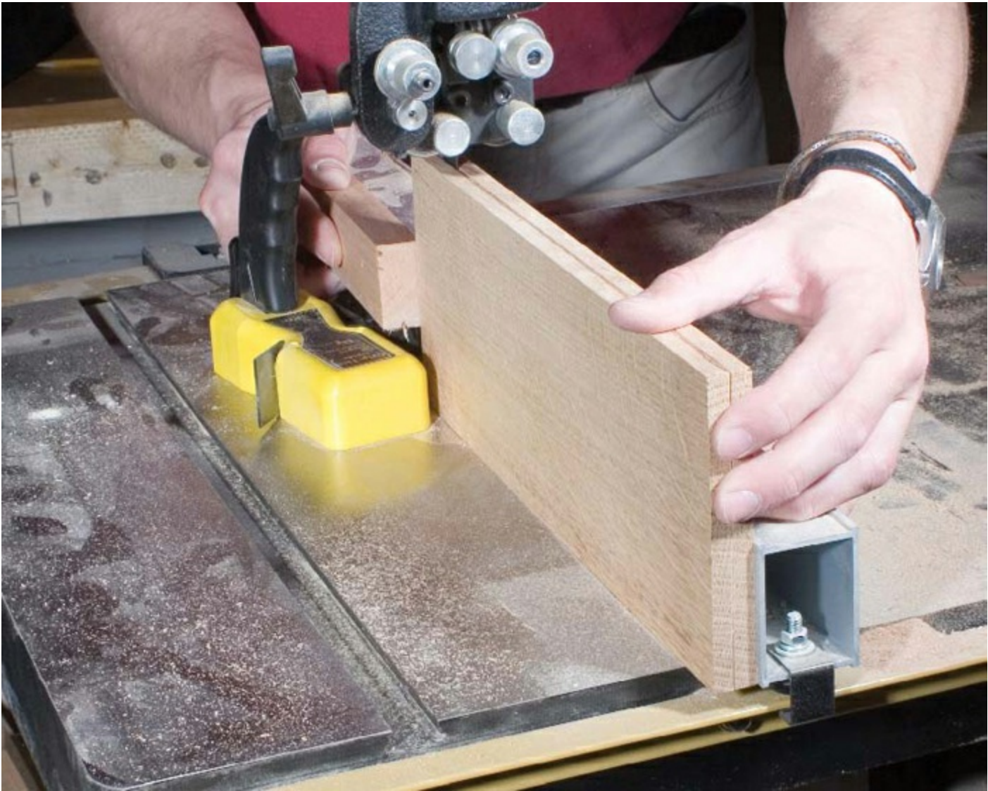
STEP 13 I chose to resaw and bookmatch the quartersawn white oak to make the floating panels. (This technique requires you to slice a board in half, opening the two pieces like a book. When glued together, one piece is a mirror image of the other.) The graining in the bookmatched panels for this particular piece looks very similar to the stems of a large leaf. You can also make the panel with multiple hardwood boards glued together or a piece of 1/4"-thick plywood. If you choose to use plywood, find a piece that is veneered on both sides because both sides will be visible.
