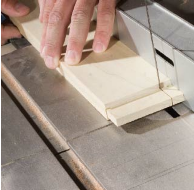
STEP 3 One of the easiest ways to cut the tenon faces is to use a tenoning fixture at the table saw. The tenons can also be cut using the same setup shown in step 2. Incrementally move the apron away from the fence and nibble the material away. Do this on both faces.
