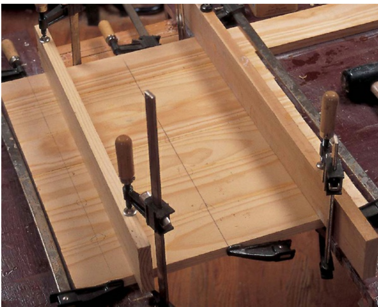
STEP 3 Use battens to help keep the glued-up sides flat.
