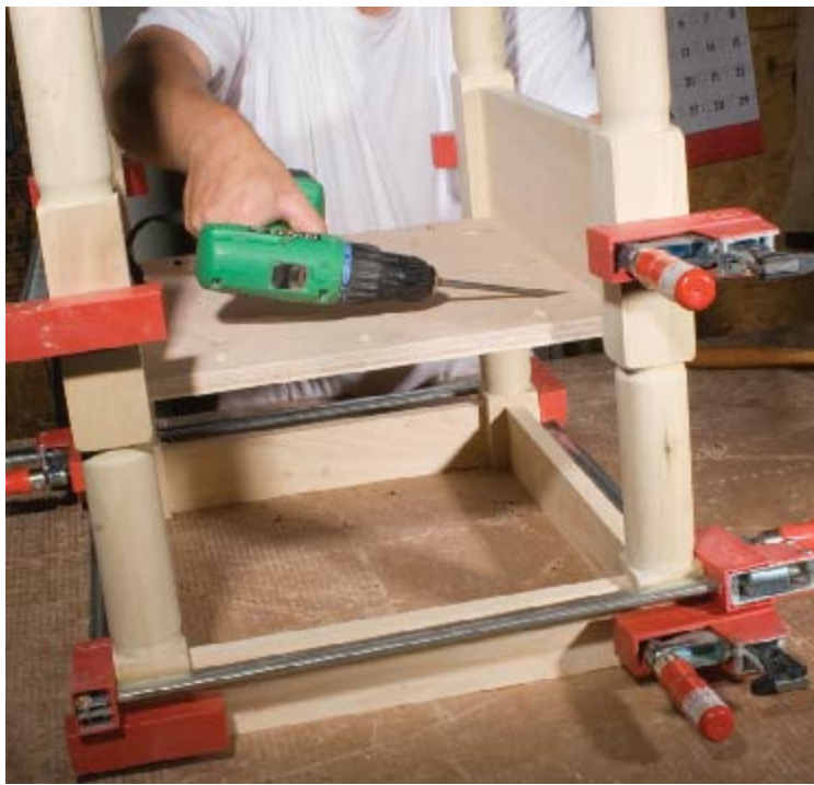
STEP 8 Using glue, pocket holes and screws, attach the top of the drawer box.
