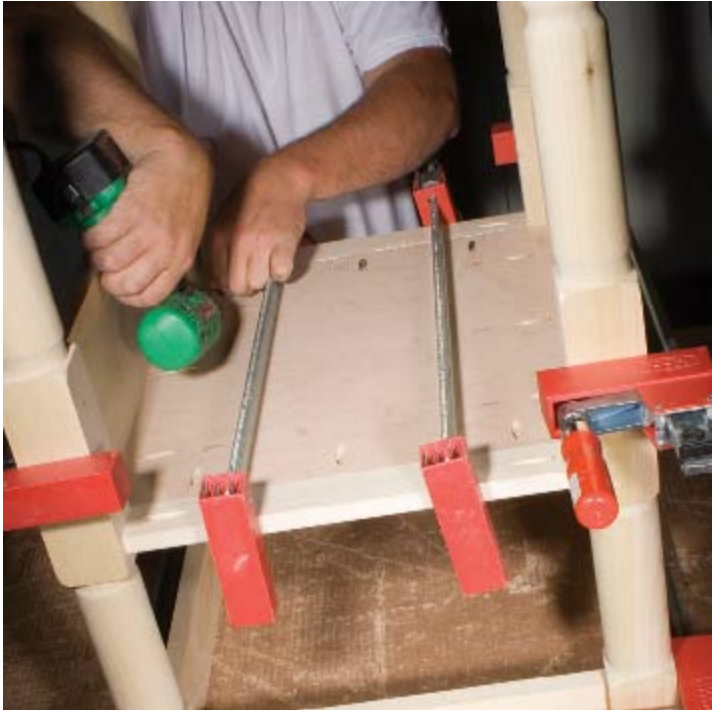
STEP 9 Using glue and pocket screws, attach two edging rails to each end of the top of the drawer box.
