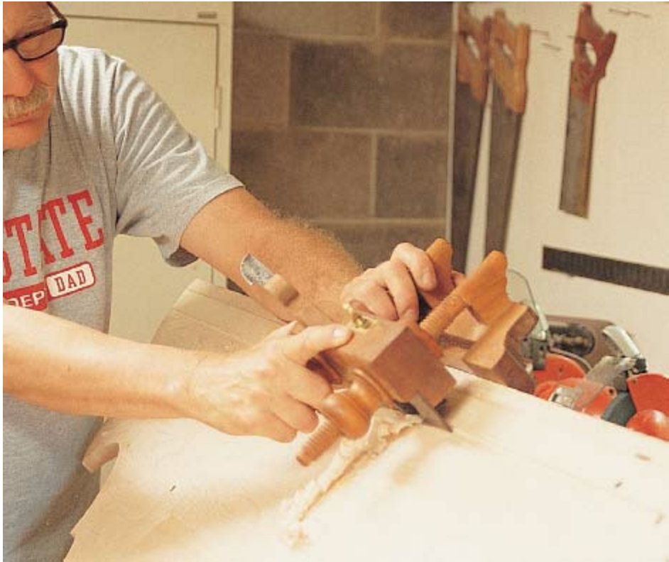
STEP 24 In order to hide the light cord, drill a hole in the cabinet top and another hole in the cabinet back. Then, on the back side of the cabinet back, plow a groove that intersects the drilled hole in the cabinet back. I cut this groove with a plow plane, but you might choose to cut it with a router and a straight bit. After the cabinet is finished, mount the light, cut the plug from the light cord, feed the cord through the hole in the cabinet top, the hole in the cabinet back, and lay the cord in the plowed groove. The groove allows the cord to exit the cabinet at the very bottom. Then put a new plug on the cord
