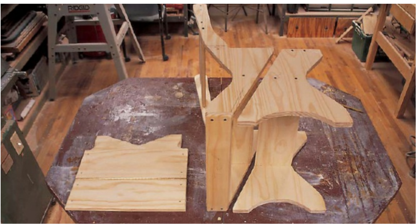
STEP 11 Assemble the chair using glue and screw s.
