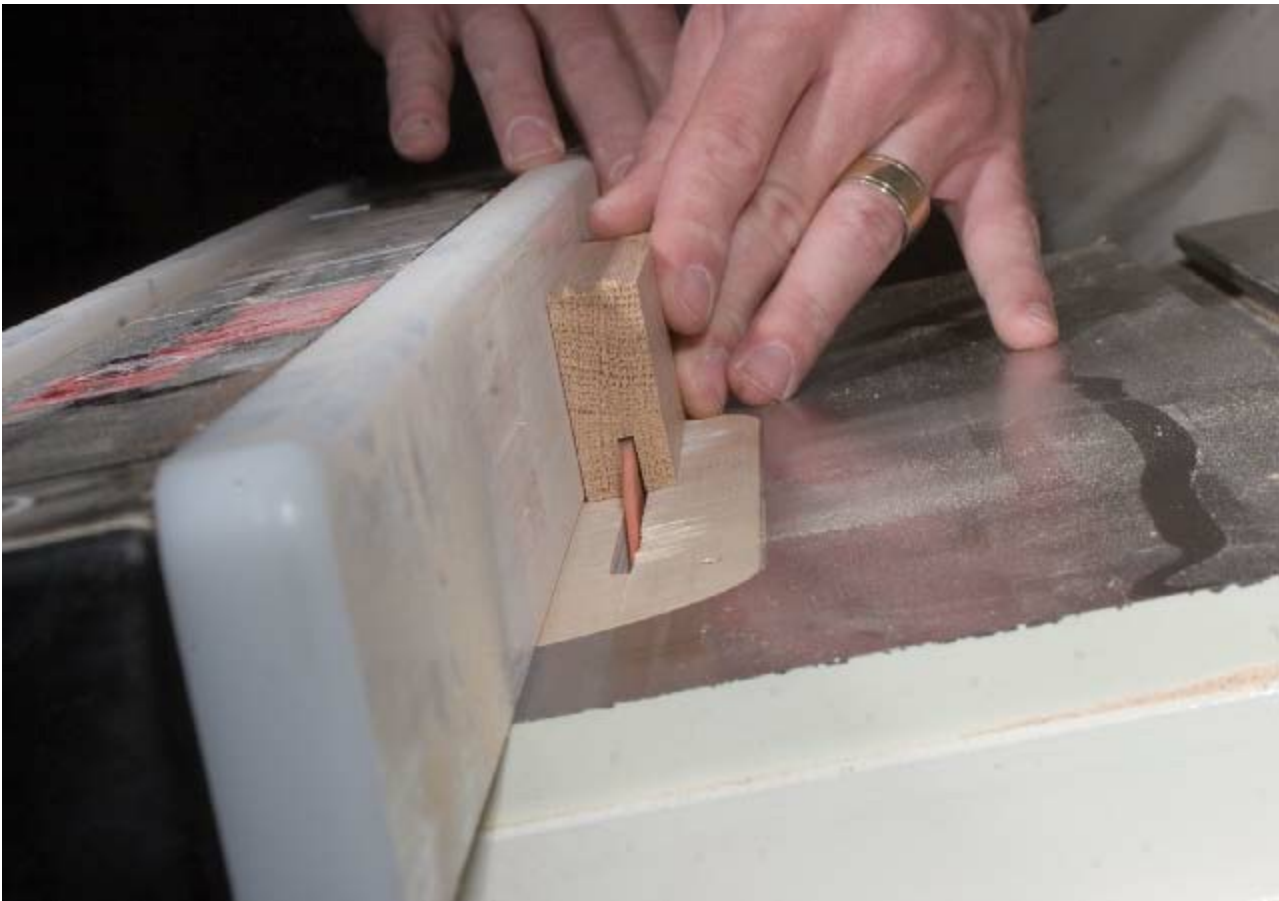
STEP 5 Mark the center of one of the rails. Using a square tooth blade, position the force on the blade will cut to one side of the centerline. Raise the blade to 1/8" high and cut a through
