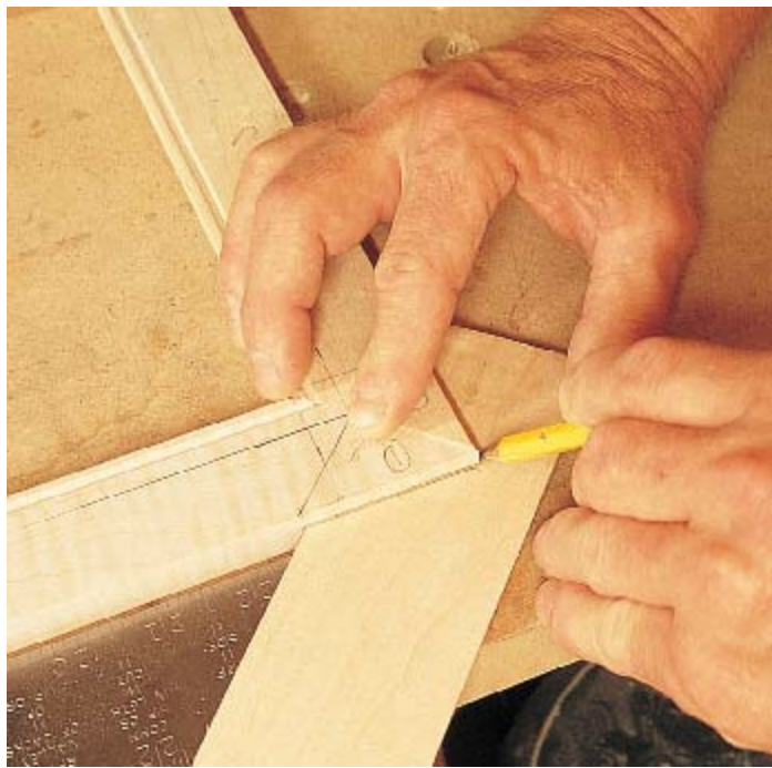
STEP 16 The grain in the feather must run perpendicular to the miter joint it is crossing. If the grain runs parallel to the miter, the feather won't have any strength.
