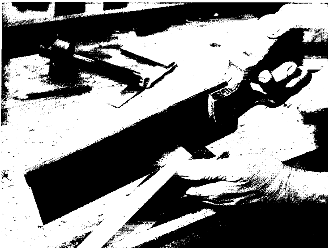
144 Sawing in tenon (second cut)
