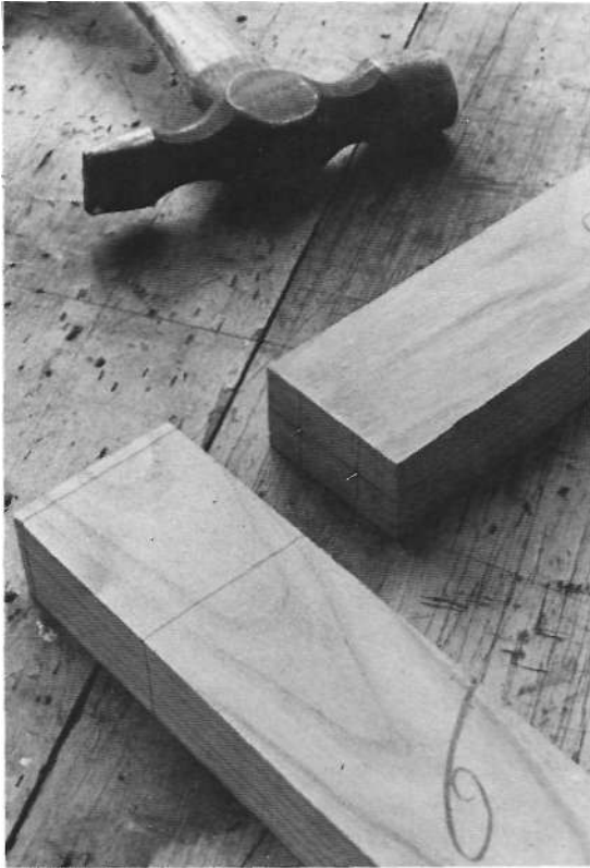
152 Setting/laying out dowel positions
