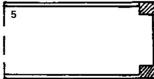
5 veneer edging or spline with cock or corner beads
