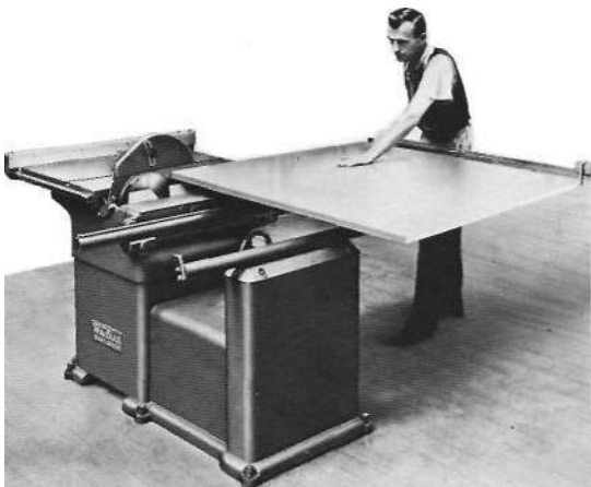
99 12 in (304 mm) sliding-table panel-saw (dimension saw)
