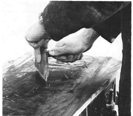
282b Holding the veneering hammer with both hands
