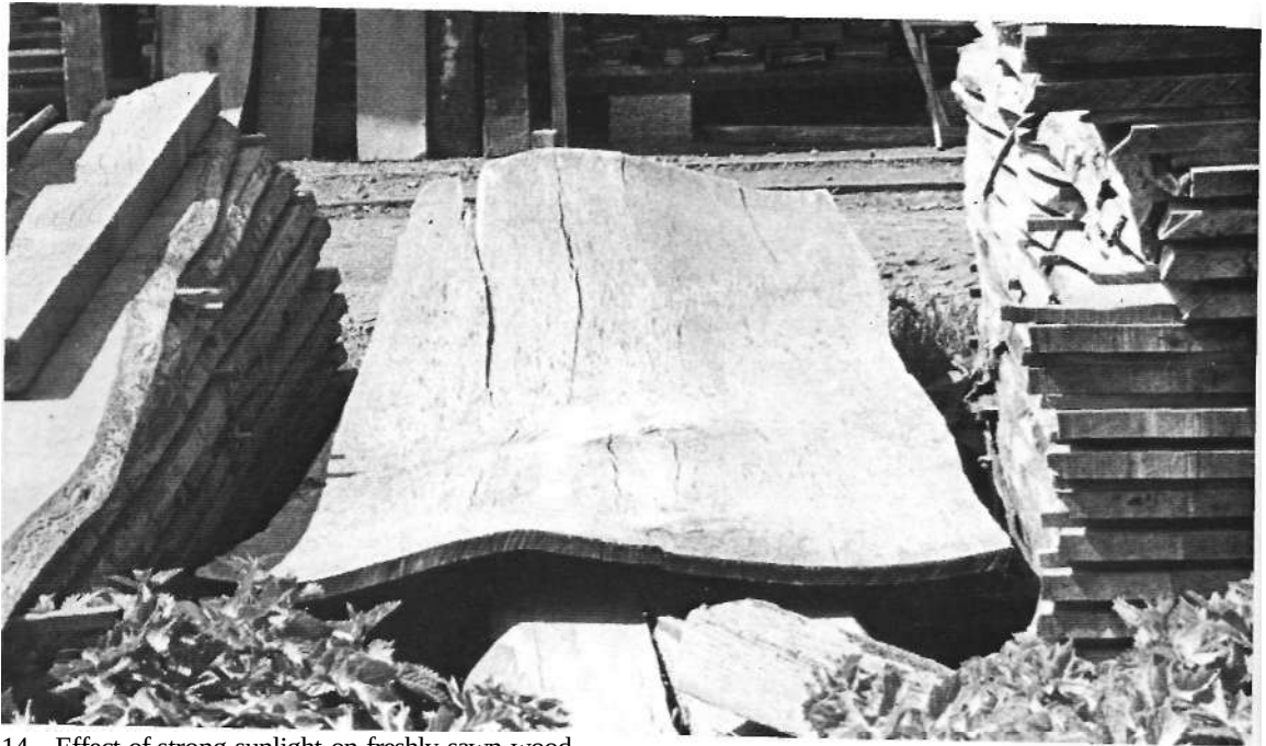
14 Effect of strong sunlight on freshly sawn wood
