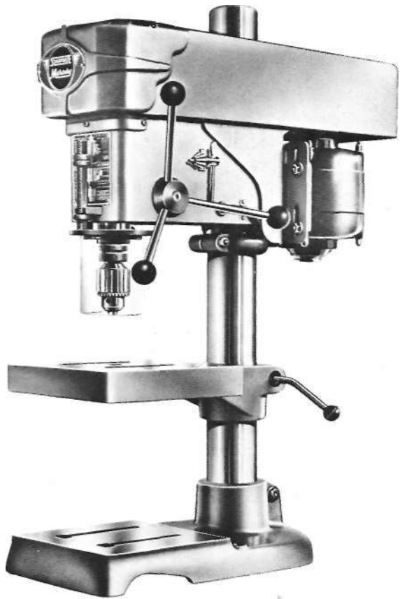
115 1 1/2 in (12.5 mm) capacity five-speed table drill or drill press
