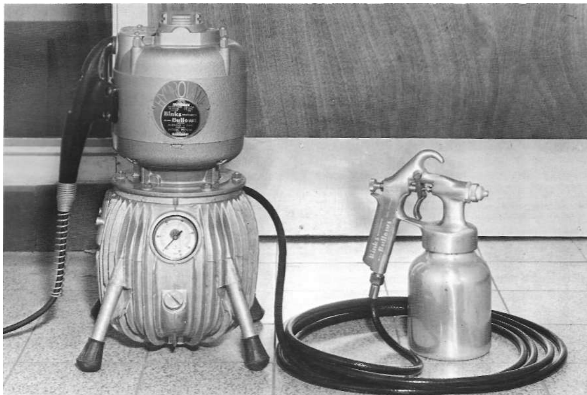
547 Portable rotary vane air compressor. (By courtesy of A. Bullows and Co. Ltd)
