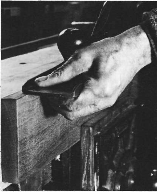
130 Correcting bevelled edge
