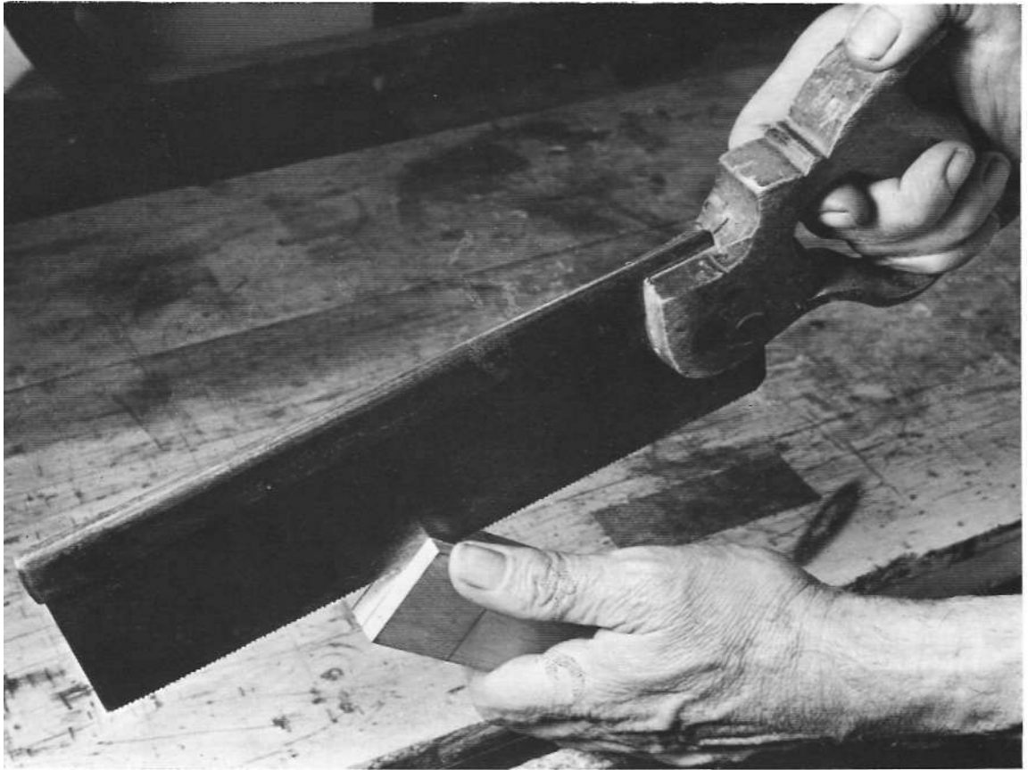
143 Sawing in tenon (first cut)
