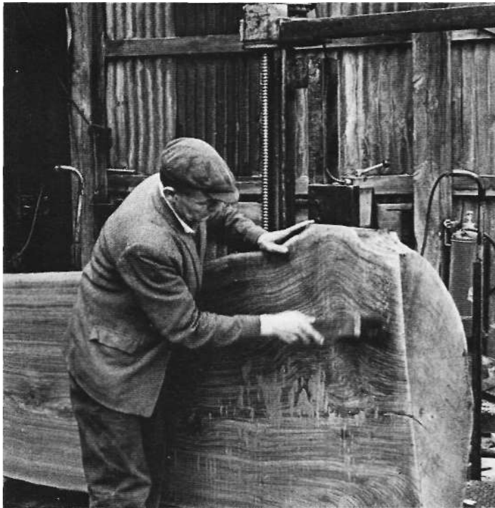
8 Brushing sawdust from log prior to next cut
