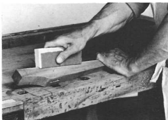
311 Sanding edge with shaped rubbing block
