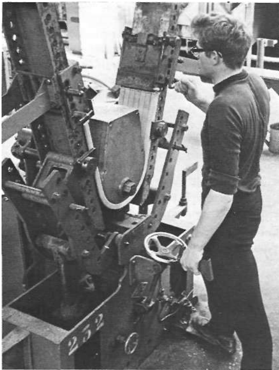
323 Finishing laminated shapes at the factory of Alesbury Brothers Limited. (By courtesy of CIBA [ARL] Ltd)
