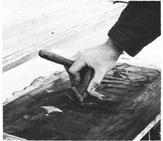
282a Holding the veneering hammer with one hand
