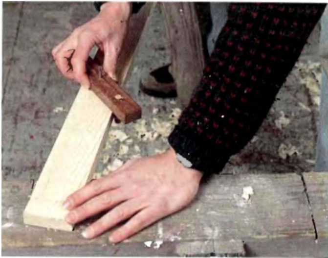
AN EFFECTIVE AND CHEAP centering scribe can be made from a piece of scrapwood, two dowels, and a drywall screw, as the author demonstrates above.
