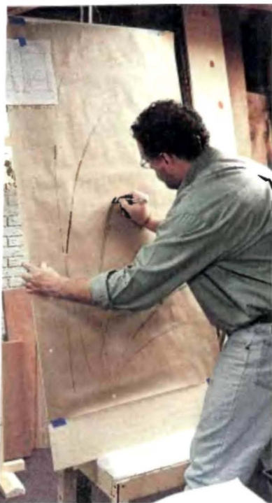
TO THE BIG BOARD. A piece of plywood propped on a chair (another old mock-up) serves as an easel for sketching the carving design. The author uses a fat pencil to produce a flowing line.
