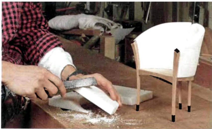
A CUSHION THAT'S REALLY FOAM. High-density, white polyurethane foam shapes easily and is perfect to mimic upholstery in scale models.
