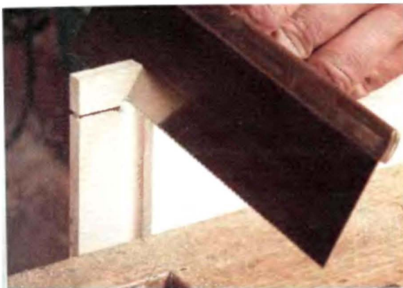
THIS HANDWORK IS FAST and accurate enough. A dovetail saw makes quick work of trimming the angled haunch and mitering the ends of the tenons.
