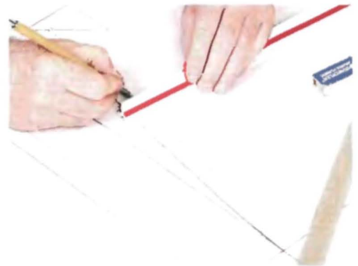
DRAW THE RAILS IN THE TOP VIEW. Use the overhang dimension to offset the curved rail evenly from the curved tabletop. Lowe is using a triangular scale, but any ruler will do.
