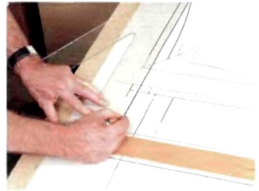
TRANSFER LINES FROM THE PLAN view to the front view. Use a long triangle to carry down the tabletop and leg edges.
