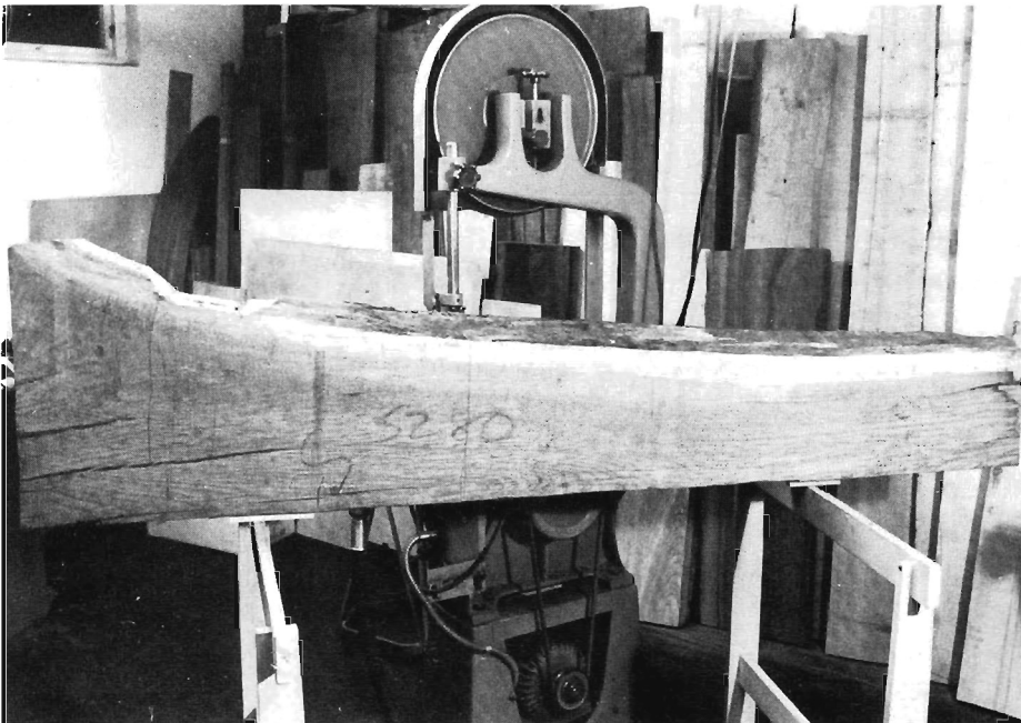
Oak plank to be thought about, laid out with an intention, sawn, and then re-sawn. Note the cracks: one of them is sixteen inches long.
