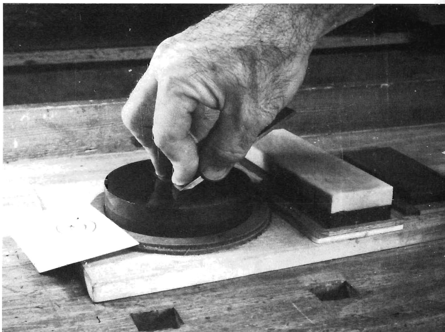
Whetting. India or Washita oilstone can be used directly after grinding with fine-grit wheel.
