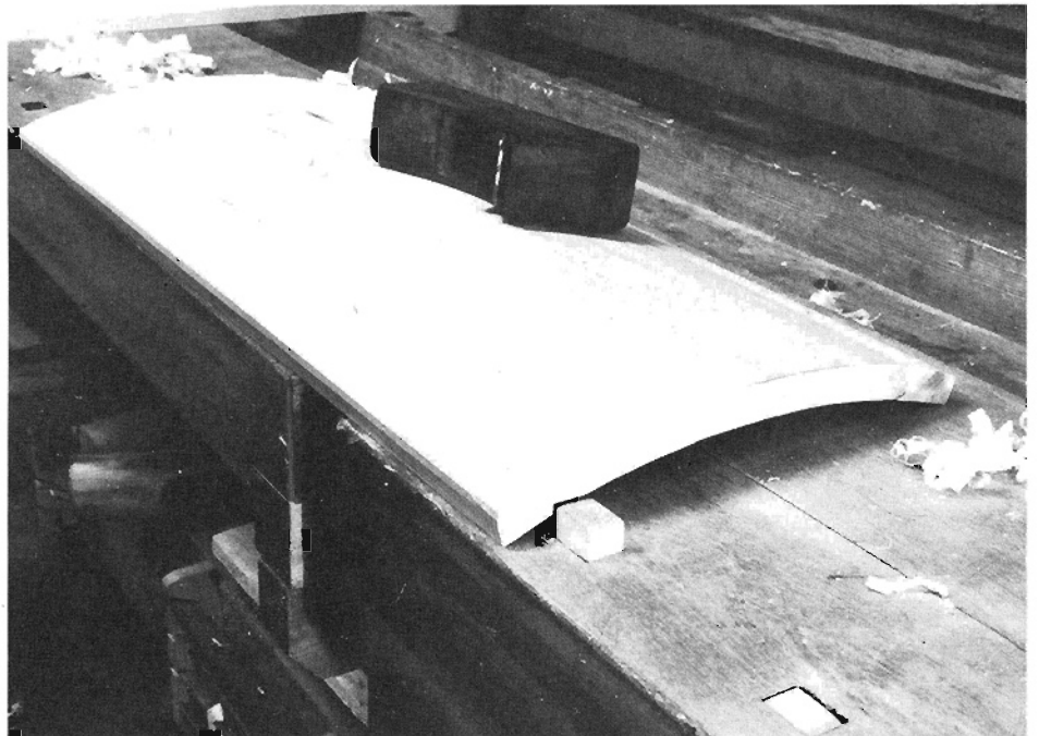
Rough-shaping two glued pieces at a time is handy—and will reveal any slight fault in the wood or the glue joint.
