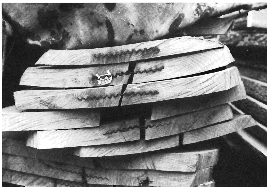
Flitch-cut log of beechwood. The tendency to warp during the initial drying is towards the outside of the tree and its longer rings.
