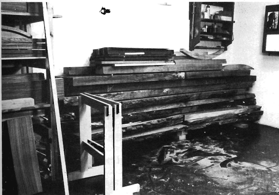
Wood sawn with portable mill pinned and stacked to air-dry. It should be protected from rain, etc. but given free circulation of air.
