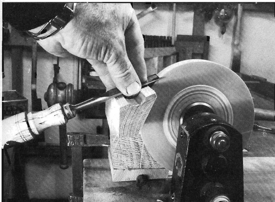
Grinding chisel with help of narrower toolrest of wood.
