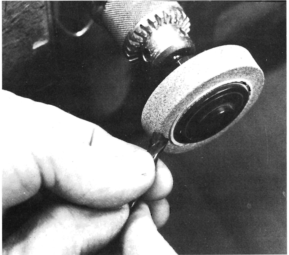
Regrounding drill-tip. Edge of wheel should be slightly rounded.
