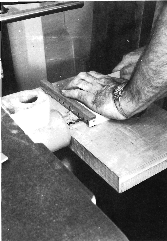
Drilling for dowels in end-grain of cabinet sides.
