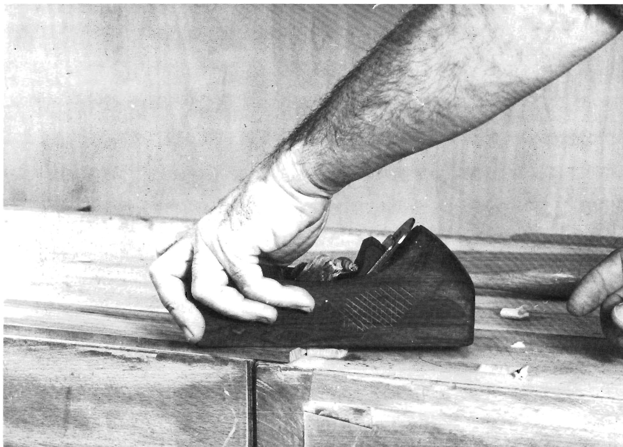
Three principal stages of a natural and effective stroke with a wood plane.
