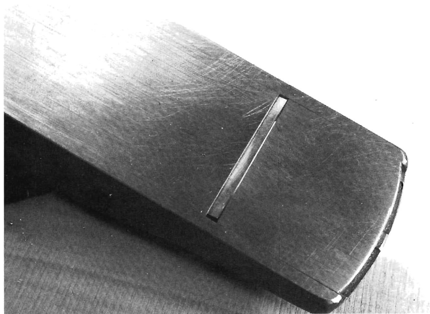
The opening of such a plane should be set as thin as possible for the work to be done.
