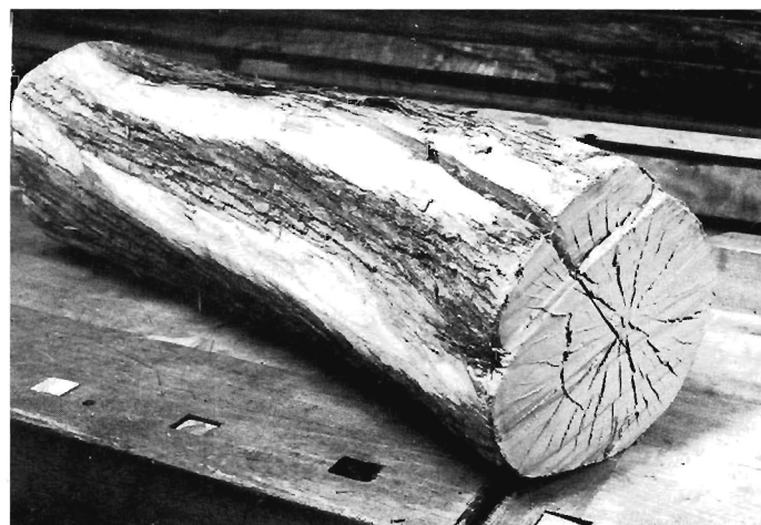
Applewood left unopened and stored in unheated garage. Note twist in split: this adds to waste of otherwise fine wood.
