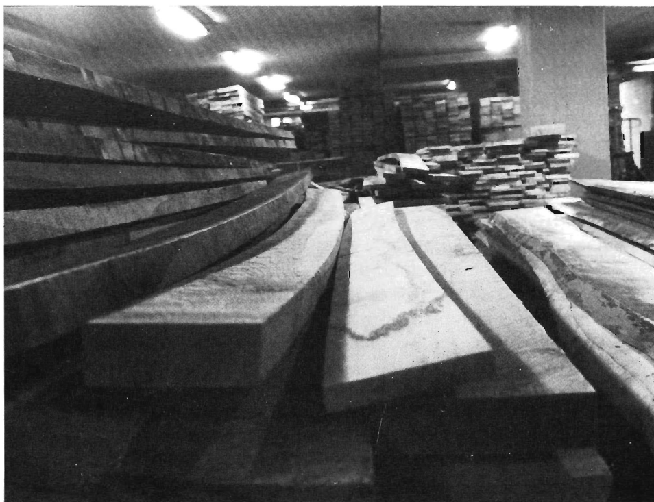
Oak pieces sawn slash-grain at outside of log. Note spring, or bend, which is result of pent-up tensions in the tree itself. However dried, such wood is apt to misbehave.
