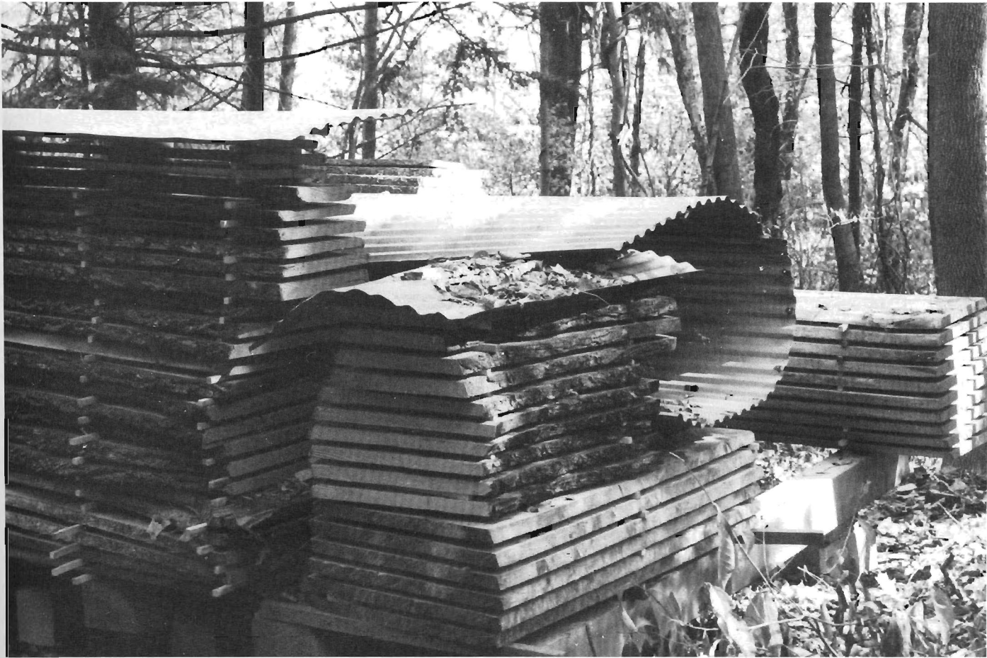
Wood sawn with portable mill pinned and stacked to air-dry. It should be protected from rain, etc. but given free circulation of air.
