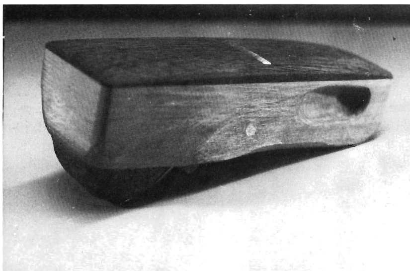
Planes with bottoms shaped to various curves.
