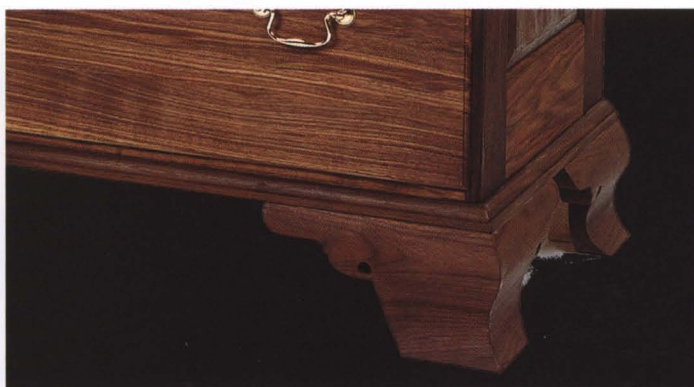
The ogee bracket foot is a versatile element used to create bases for case pieces. Often used in high style pieces, it is more elegant and sinuous than a flat base.
