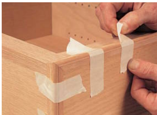
Wrap small moldings with masking tape until the glue sets.
