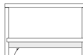
Glue rail under bottom near front of case.
