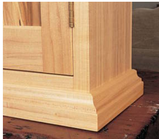
A built-up base provides a classic touch to a small cabinet.
