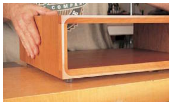
When the case is turned right side up, a slight rise creates an attractive shadow line.
