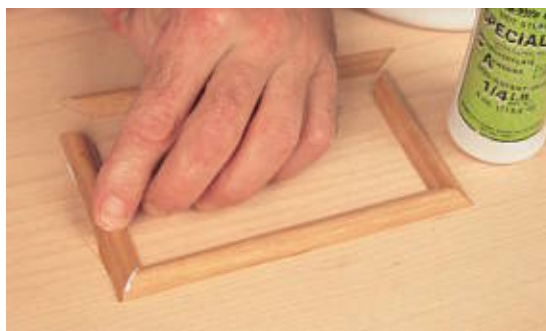
Immediately press the white glue and CA mixture to the work surface. In seconds, the molding is secure.
