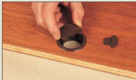
Tap the barbed grommet into the hole. A plastic cap reduces the opening for smaller runs of wire.
