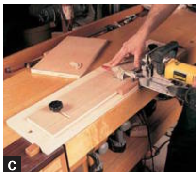
This hold-down jig lets you safely cut biscuit slots in short or narrow stock without having your hands near the cutting action.
