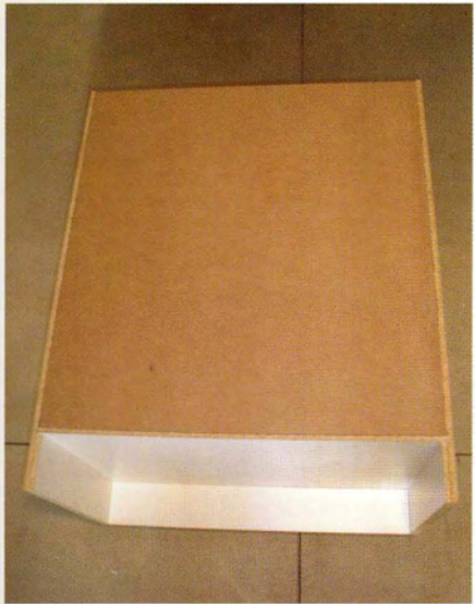
15 Lay the cabinet face down. The back should fit snugly into the rabbets. The back will help square the cabinet, so a good fit is important. You can use a framing square or measure diagonally from top to bottom. Repeat with the opposite corners. If the cabinet is square, both measurements will be the same. If the measurements are not the same, adjust the longest dimension by pulling the corners diagonally together until the cabinet is square.
