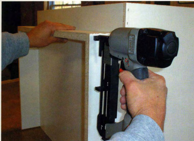
8 Attach the toe kick between the sides.
