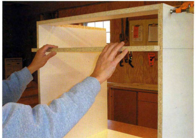
9 Stand the cabinet up, then install the rails using glue and staples or screws. Use a bar clamp to hold the sides tight to the rails.
