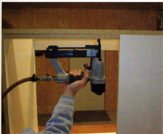
12 Attach the sub rail to the top front rail.
