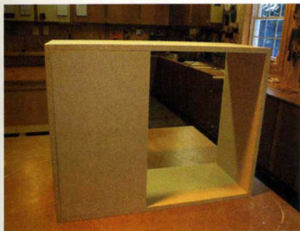
9 Install the filler panel between the top and bottom panels and next to one side.
