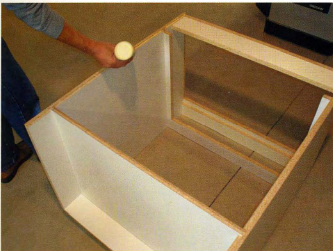
13 Lay the cabinet face down. The back should fit snugly into the rabbets. The back will help square the cabinet, so a good fit is important. You can use a framing square or measure diagonally from top to bottom. Repeat with the opposite corners. If the cabinet is square, both measurements will be the same. If the measurements are not the same, adjust the longest dimension by pulling the corners diagonally together until the cabinet is square.
