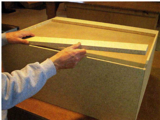
15 Glue and staple or screw the nailers in place on the back of the cabinet.
