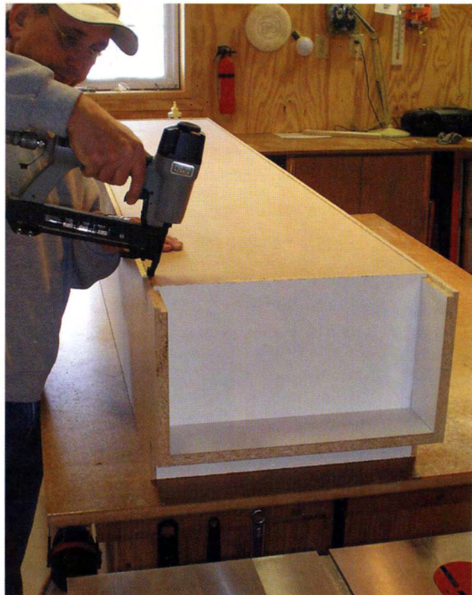
17 Finally, attach the back with glue and staples or nails.
