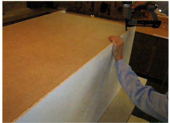
16 Finally, attach the back with glue and staples or nails.
