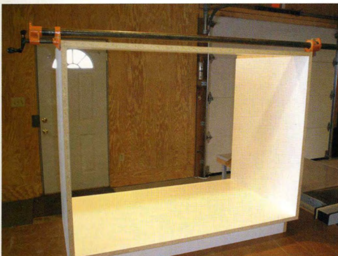
9 Install the front and back rails. Use a clamp to hold the rails in place.
