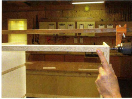
10 Stand the cabinet up, then install the rails using glue and staples or screws. Use a bar clamp to hold the sides tight to the rails.
