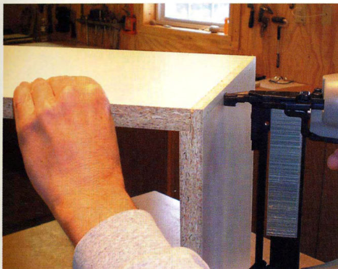
7 Use staples or screws to attach the bottom panel.
