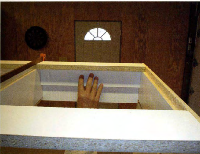
14 Install the drawer support. At the back of the cabinet, use the sub rail as a spacer to locate the drawer support. Attach the support to the nailer in the back.
