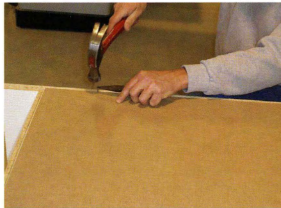
16 Add glue to the rabbets and set the back panel in place. Be sure to check for squareness of the cabinet, then attach the back.
