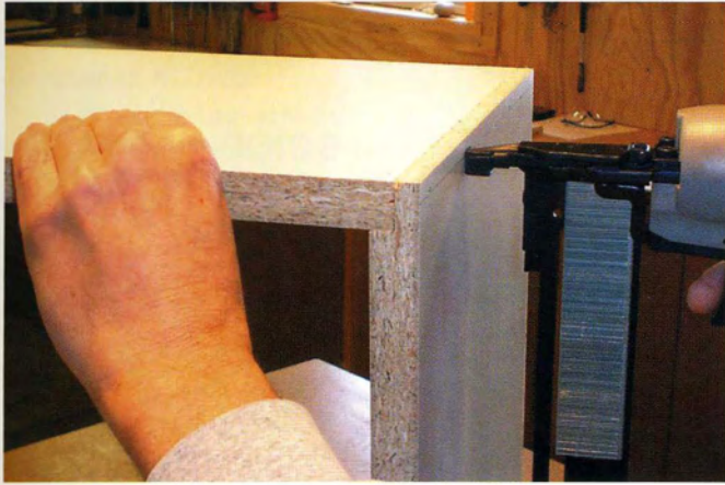
7 Use staples or screws to attach the bottom panel.
