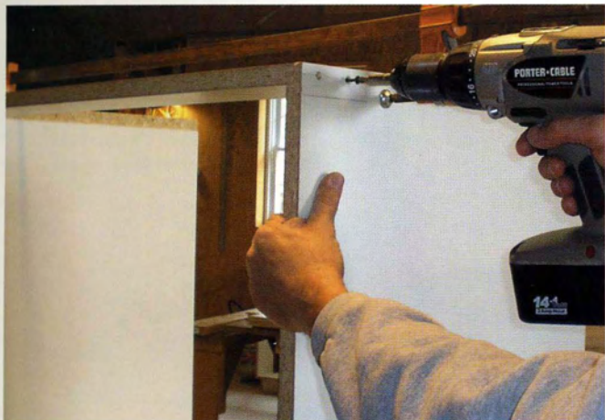
8 Install the front and back rails. Use a clamp to hold the rails in place.
