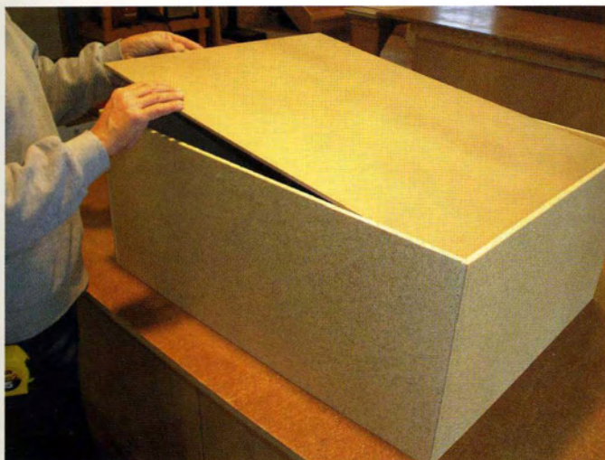
12 Lay the cabinet face down. The back should fit snugly into the rabbets. The back will help square the cabinet, so a good fit is important. You can use a framing square or measure diagonally from top to bottom. Repeat with the opposite corners. If the cabinet is square, both measurements will be the same. If the measurements are not the same, adjust the longest dimension by pulling the corners diagonally together until the cabinet is square.
