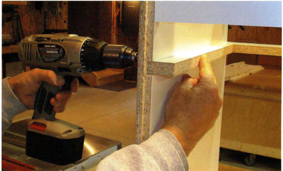
14 Glue and staple or screw the drawer glide supports in place.
