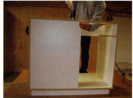
13 Install the filler by attaching to the side, top rail and bottom panel.
