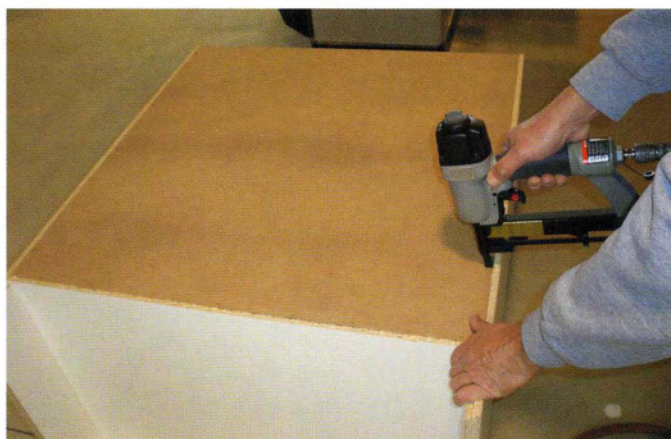
12 Add glue to the rabbets, check for squareness and attach the back.
