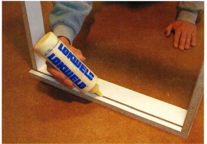
9 Apply glue in the groove that accepts the bottom panel.
