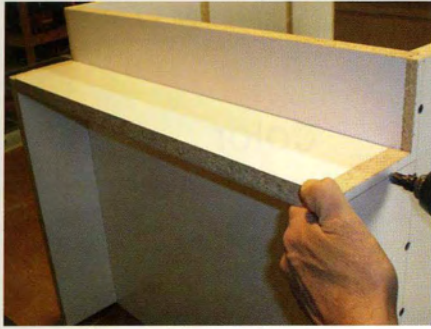
9 Attach the toe kick between the sides.
