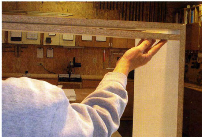
9 Attach the sub rail under the top rail.
