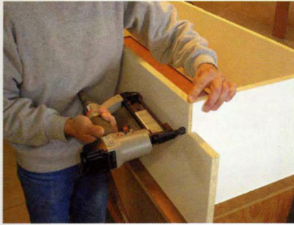
10 Starting at the bottom, attach the other side.
