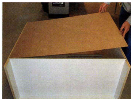
14 Lay the cabinet face down. The back should fit snugly into the rabbets. The back will help square the cabinet, so a good fit is important. You can use a framing square or measure diagonally from top to bottom. Repeat with the opposite corners. If the cabinet is square, both measurements will be the same. If the measurements are not the same, adjust the longest dimension by pulling the corners diagonally together until the cabinet is square.
