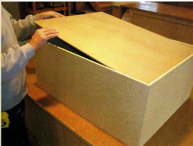
12 Lay the cabinet face down. The back should fit snugly into the rabbets. The back will help square the cabinet, so a good fit is important. You can use a framing square or measure diagonally from top to bottom. Repeat with the opposite corners. If the cabinet is square, both measurements will be the same. If the measurements are not the same, adjust the longest dimension by pulling the corners diagonally together until the cabinet is square.
