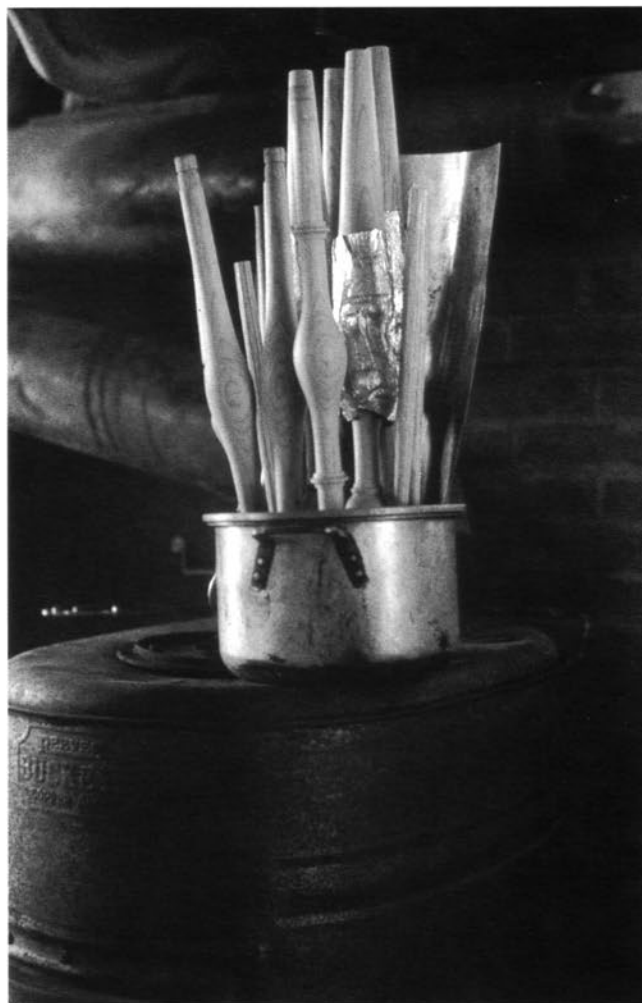
Drying legs and stretcher tenons in warm sand (120 to 140 degrees). Check the temperature at the bottom of the sand. The sand pot is on a wood stove; an electric hot plate also works fine.
