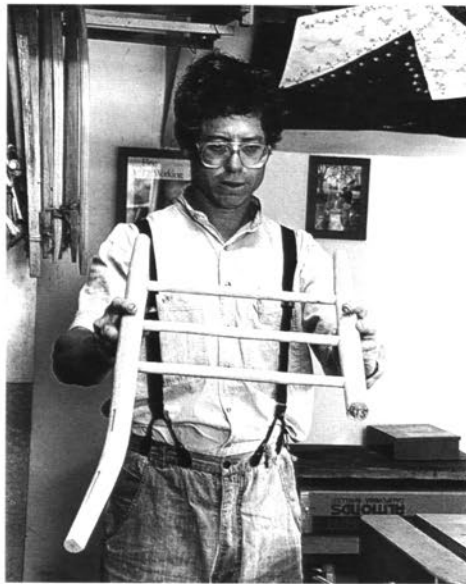
Checking across the side rungs to see if the panel is flat. You can try to correct warp by twisting in the opposite direction.
