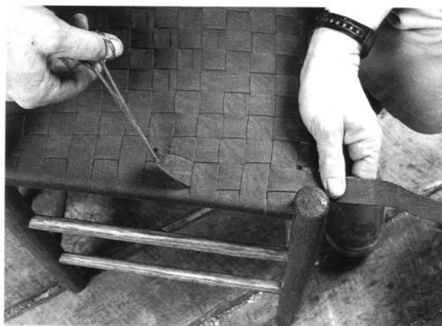
Weaving the ears (the side triangles). A surgeon's hemostat (a locking pliers) is useful here—hospitals throw them away.
