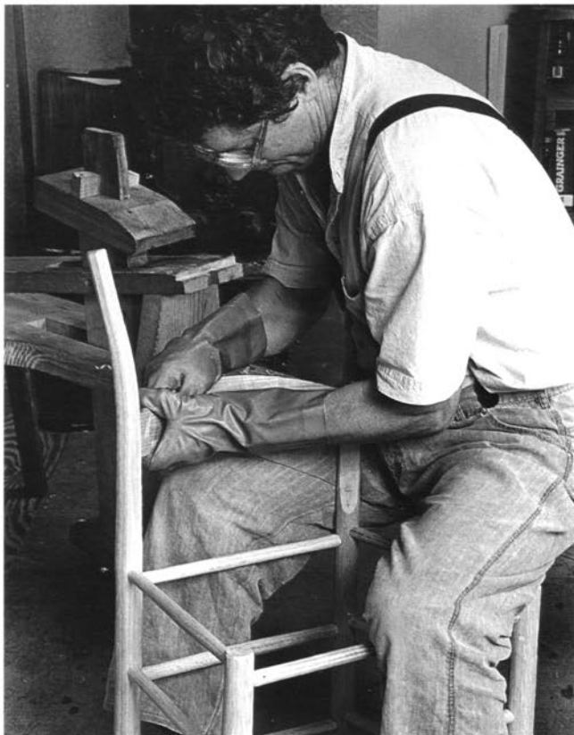
Fitting the lower slat into the mortises—something of a wrestling match.
