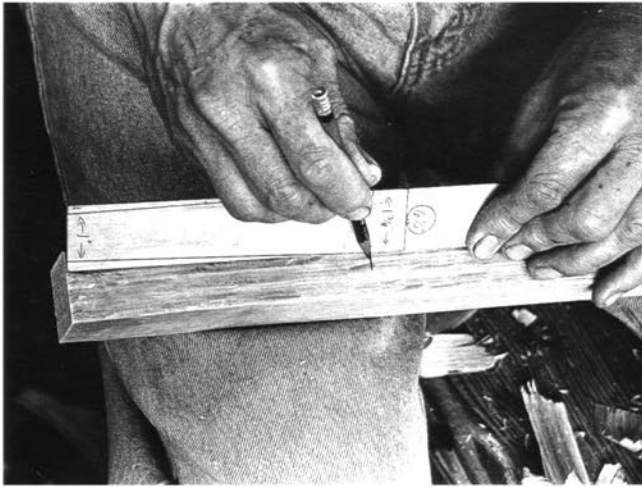
Penciling a line around the post's four sides—the tapers begin about 3/4 inch below the tangent line for the lower rungs.
