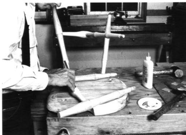
Gluing up the Windsor stool by disassembling, gluing, and reassembling one joint at a time cuts your chances of accidentally getting a component in the wrong place or position.
