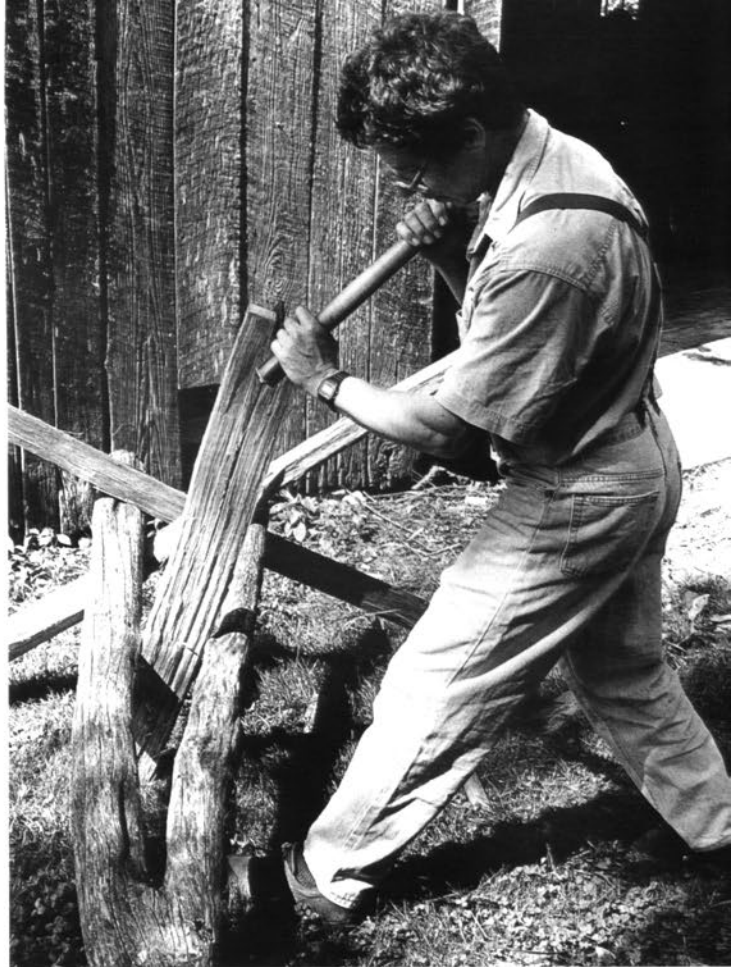
Using a splitting brake, a forked tree trunk supported by opposing poles. The brake steadies the bolt, making precise riving easier.
