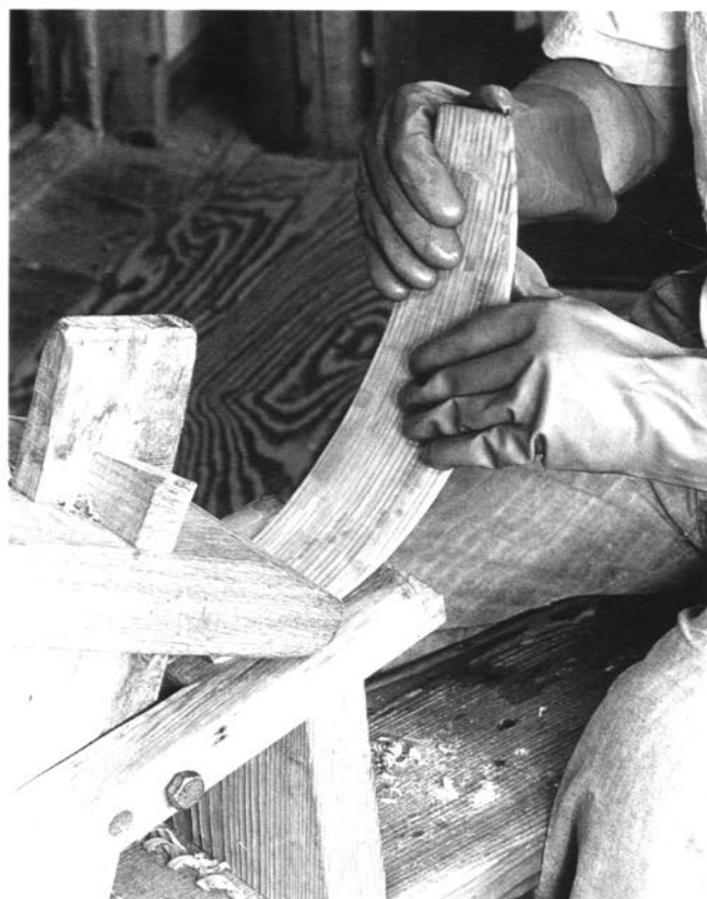
Limbering a slat at a shaving horse. Limber the entire slat, but only in the bending direction.
