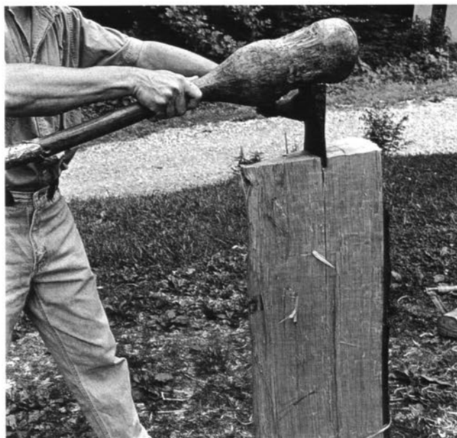
Splitting the rear posts
