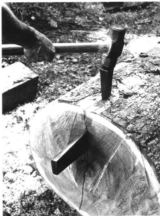
Driving a standard splitting wedge into the bark side of the log. (The starting wedge could have been driven further into the log.)
