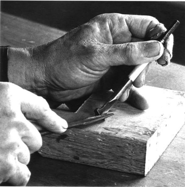
Sharpening a 5/8-inch powerbore bit with an auger bit file. Use the file only on the underside of the cutter and the inside of the side nicker.
