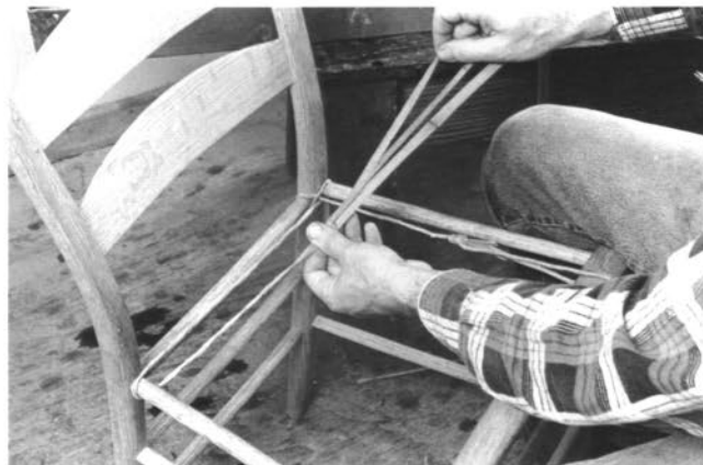
Holding the cord in tension and simultaneously weaving the seat and twisting the leaves
