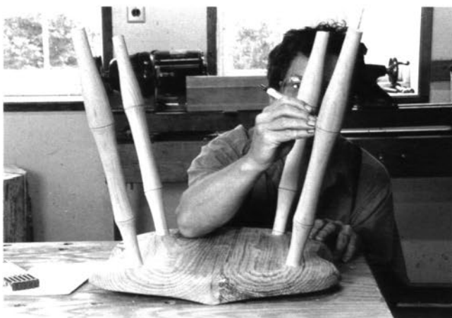
View straight across the legs to mark the center points on the bamboo nodes.
