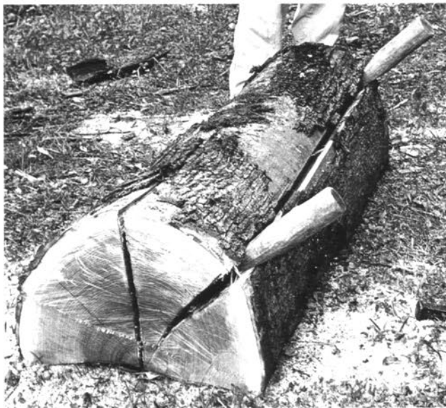
Locate gluts where cross fibers in the crack won't intercept their leading edge. Scattered cross fibers in the inner heartwood hold the split bolts together. I don't pull the bolts apart until all splits are complete. The heavy half-log is more stable than lighter split out bolts.
