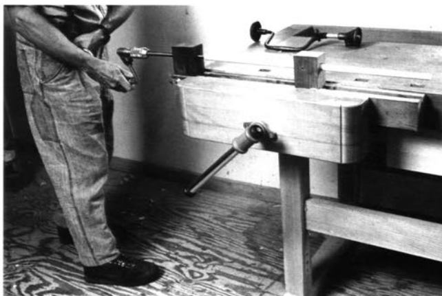
Cutting the intermediate 5/8-inch-diameter tenons on the long sticks with Brian Boggs's tenon former. The extended end will taper to a 1/2-inch-diameter tenon, which will be made with a plug cutter.
