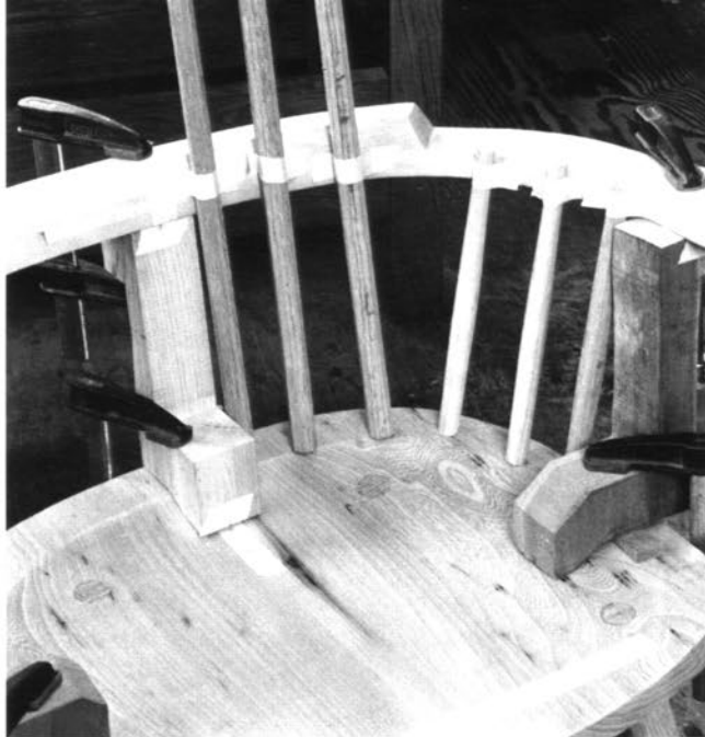
Taping sticks against the bow to check their placement before boring mortises. Make corresponding center marks in the bow and seat deck.
