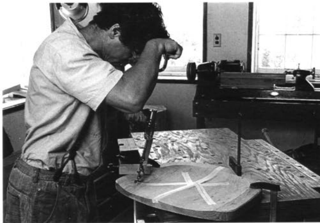
Boring a compound-angle leg mortise using the sighting line and resultant angle method. The brace is aligned with a bevel gauge set parallel to the sighting line and a try square set perpendicular to the sighting line. Masking tape on seat areas allows lines or other notations to be penciled in.
