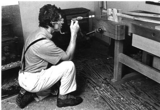
Centering the boring bit. This body position puts your sighting eye in line with the level bit shaft.
