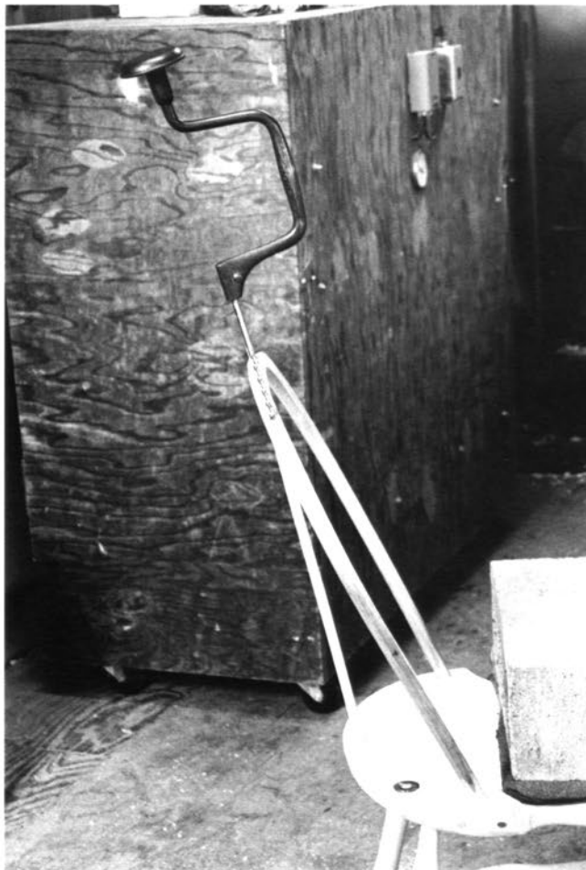
Using a standard auger bit, you can let go of the brace to check alignment from a side view. Placing a flat washer over the target mortise eliminates the possibility of aiming at the wrong point.
