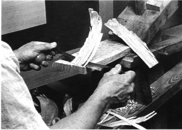
Lightly dressing one face of each riving, the first step in shaving slats. A drawknife with a slightly bowed blade makes slat shaving easier.
