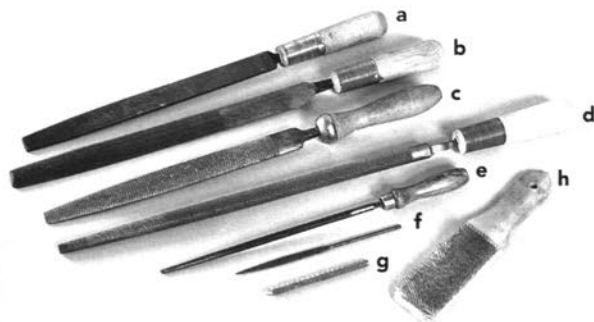
Rasps and files: a, 10-inch flat bastard file; b, 12-inch half-round file; c, 10-inch hand-cut pattern-maker's rasp; d, 5/8-by-14-inch rat-tail file; e, 5/16-by-8-inch rat-tail file; f, riffler; g, broken rat-tail file for use with electric drill; h, file card.
