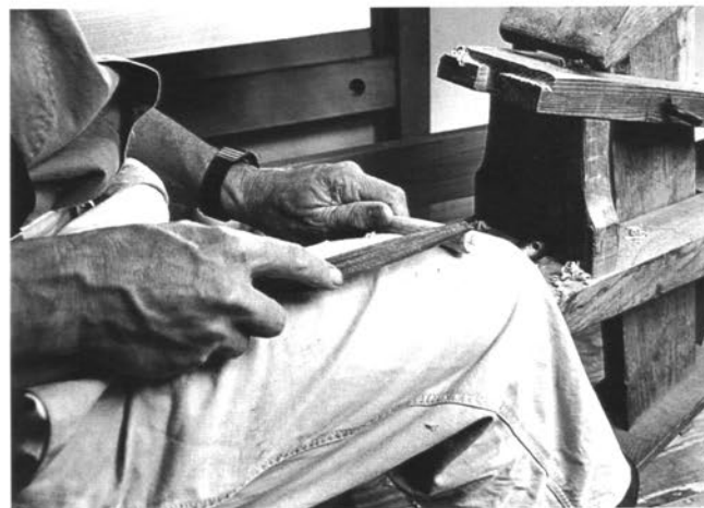
Filing a narrow chamfer around the ends of the rung. Roll the rung on your knee toward the file as you simultaneously move the file forward.
