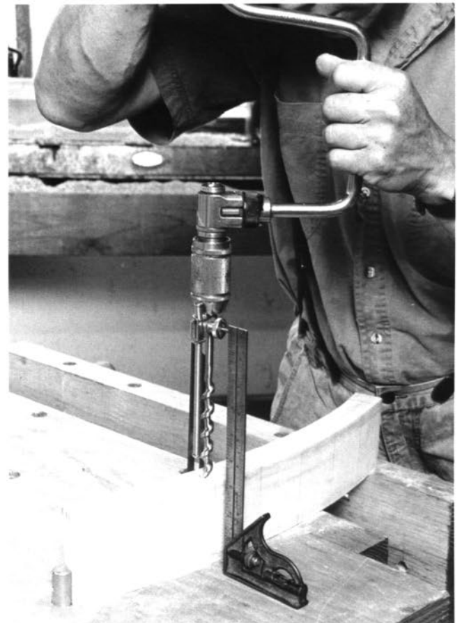
Boring 1/2-inch-diameter mortises in the comb
