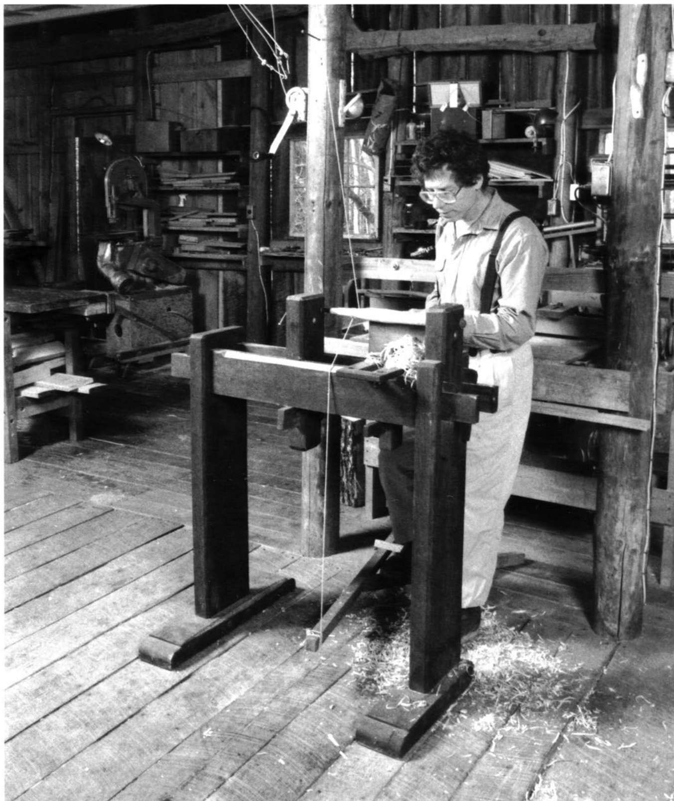
A shop-made pole lathe can be used to turn ladder-back tenons, or for complete turnings of Windsors.
