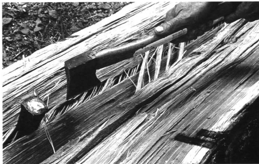
Severing connecting fibers in the split half-log with a hatchet. Note that the arc of the swung hatchet cuts away from the iron wedge.
