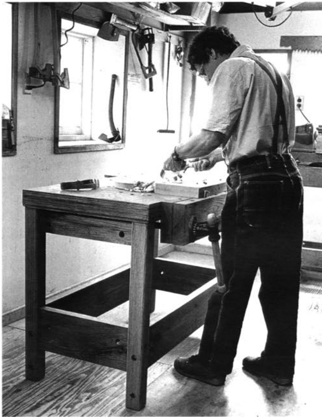
A small, sturdy workbench designed to be located several feet from a wall. It is bolted to the floor and will not move when you're doing vigorous work, such as saddling a Windsor seat with an inshave.
