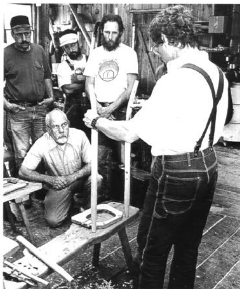
Holding the rear posts over the potty seat before boring, to mentally picture the boring angles
