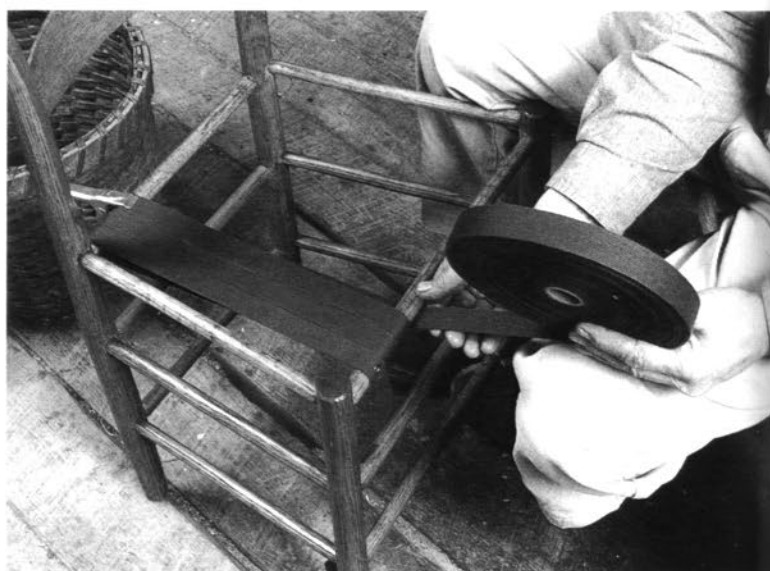
Beginning a Shaker-tape seat by winding the warp around the front and rear rungs. Hanging from the front rung is the foot-long tail, to be woven into the weft toward the end of the process.
