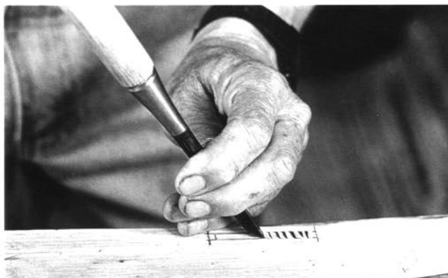
Chopping a series of cuts into the outlined surface with the mortise chisel, bevel down. Hammer lightly.
