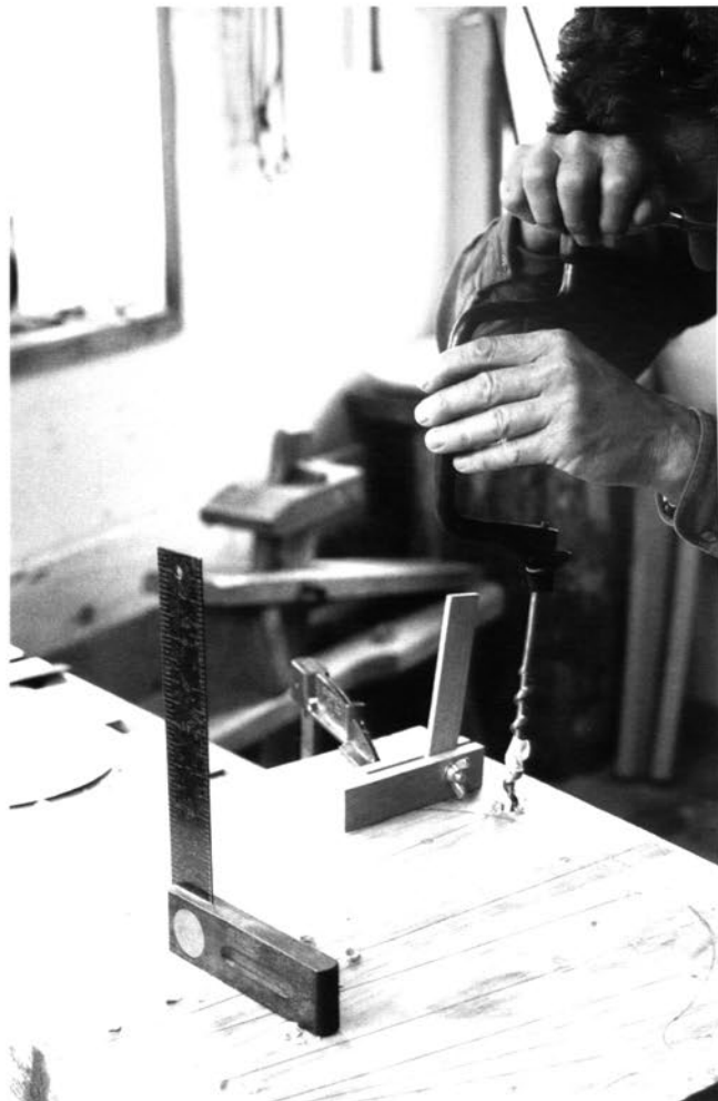
Preboring the spindle mortises in the deck—one option. You can also bore these mortises after the bow is fitted to the seat.
