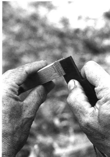
Using the notch gauge to check the dimensions of the shaved square rung. The growth-ring plane is still about 1/16 inch proud (oversized).
