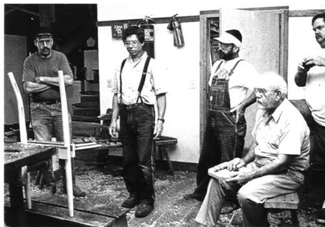
Visually checking the rear posts for flare and symmetry before boring the mortises
