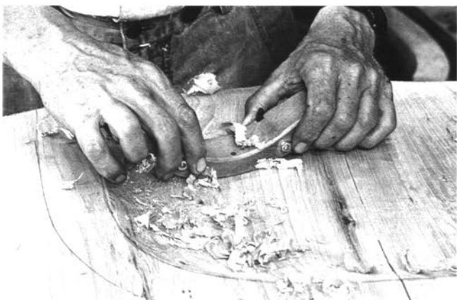
Finishing the center area of the seat with a travisher made by the author
