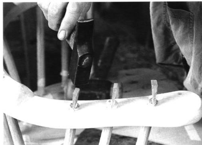
Driving wedges into the kerfs of protruding tenons
