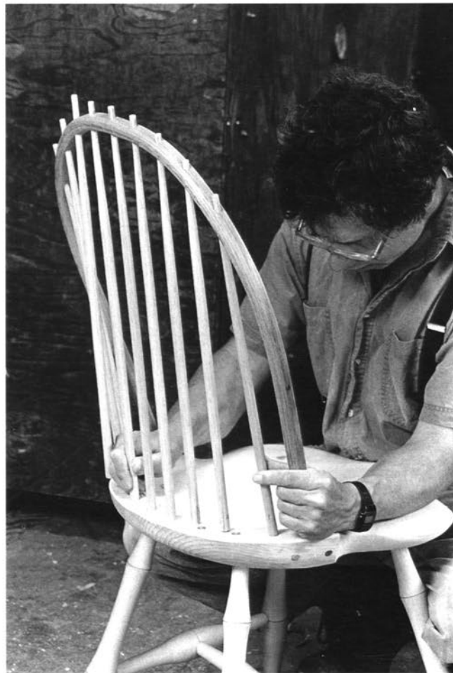
Fitting the bow and spindle assembly to the seat often requires some fiddling and wrestling.
