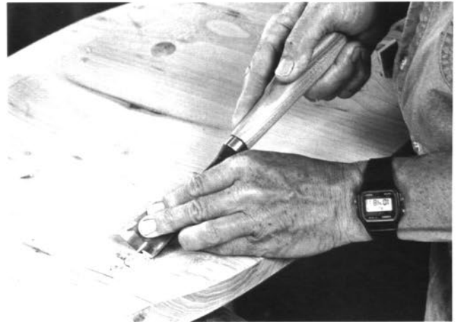
Paring the protruding tenon flush to the saddled seat
