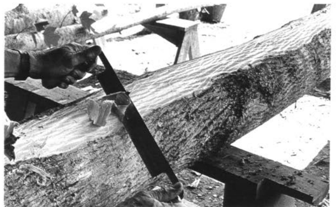
Shaving off the coarse outer bark and most of the heavily netted section of the bast
