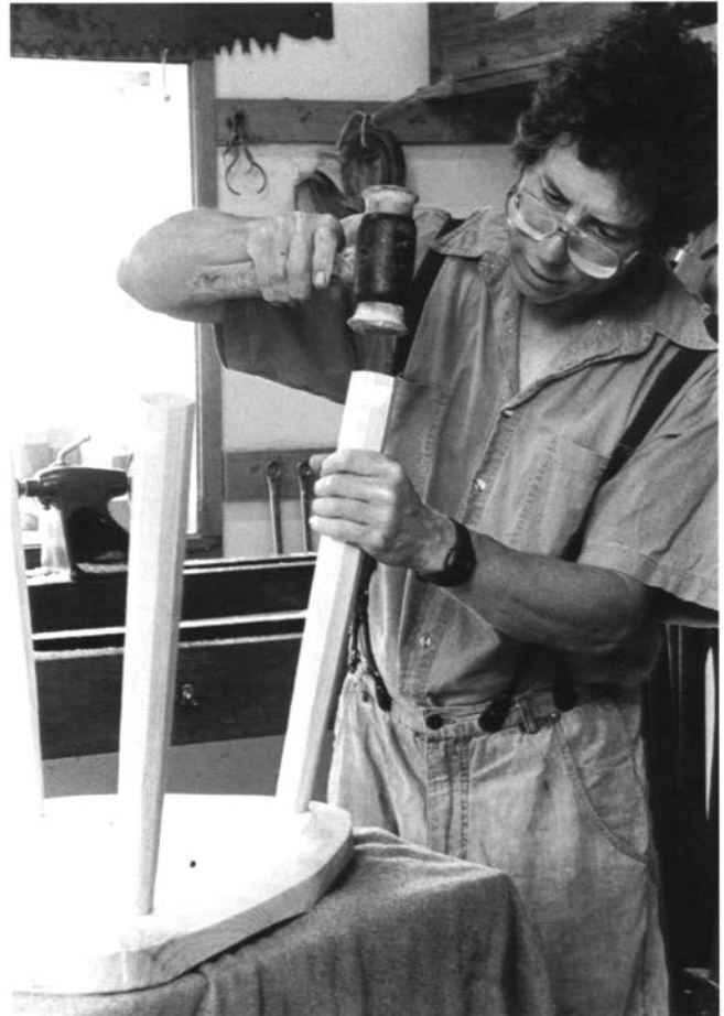
Pounding the legs home during glue up of the stool
