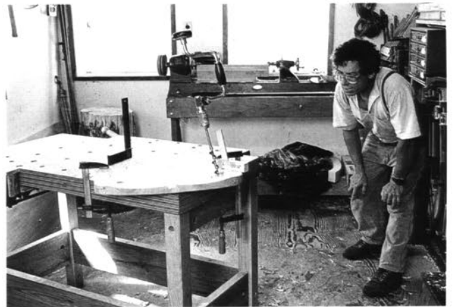
Stepping back to check the brace alignment with the angled bevel gauge and the try square (if you're using a standard auger bit, you can let go of the brace after taking a few turns into the wood).
