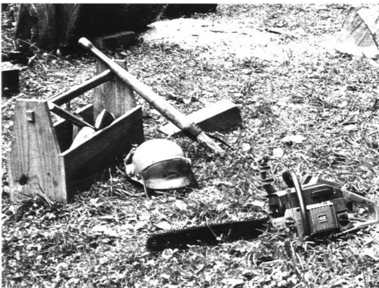
A chain saw and a hard hat that combines eye and ear protection. A cant hook leans against the tote box, used to haul wedges, gluts, and a hatchet.
