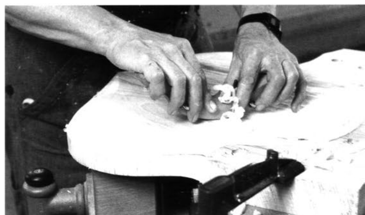
Smoothing the pond area with a travisher, a tool you can also use in the steep concave area below the deck. Take extreme slicing cuts; this tightens the effective sweep of the blade.
