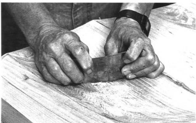
Scraping the difficult concave slope area is also useful.
