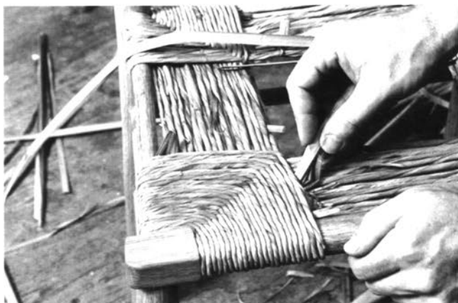
Filling the pockets at the corners with short lengths of scrap rush to begin the stuffing. Tom Donahey stuffs the top and bottom layers; other chair "bottomers" stuff only the bottom.
