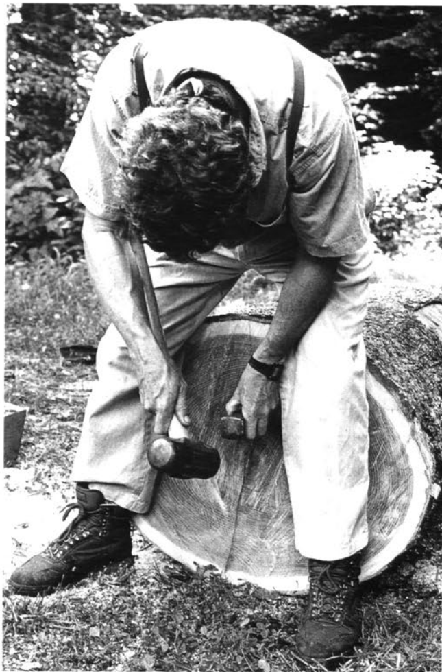
Using a standard wedge to score along the penciled line. This small indentation will influence how the split develops.
