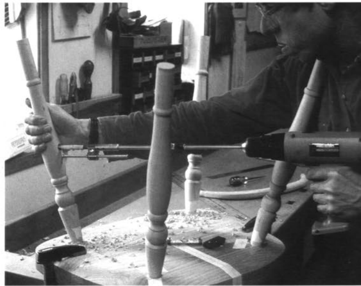
Boring mortises for the crinoline stretcher tenons with the legs fitted to the chair seat
