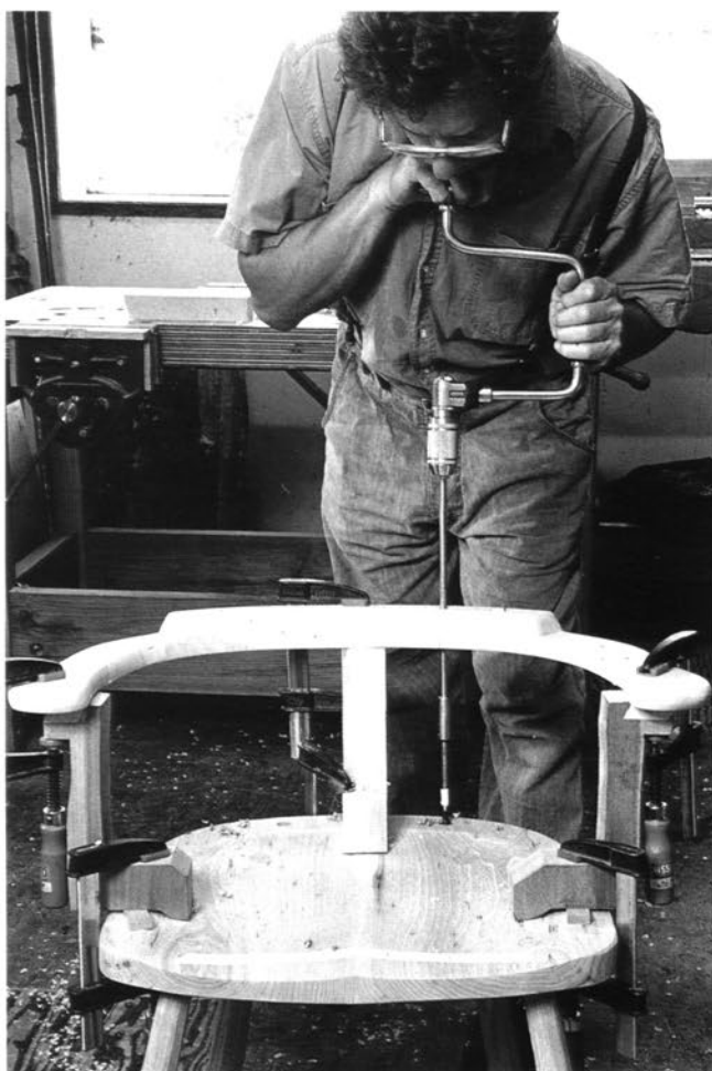
Using an extension that passes through the bow mortise for boring the seat, which eliminates any fussing with stick angles
