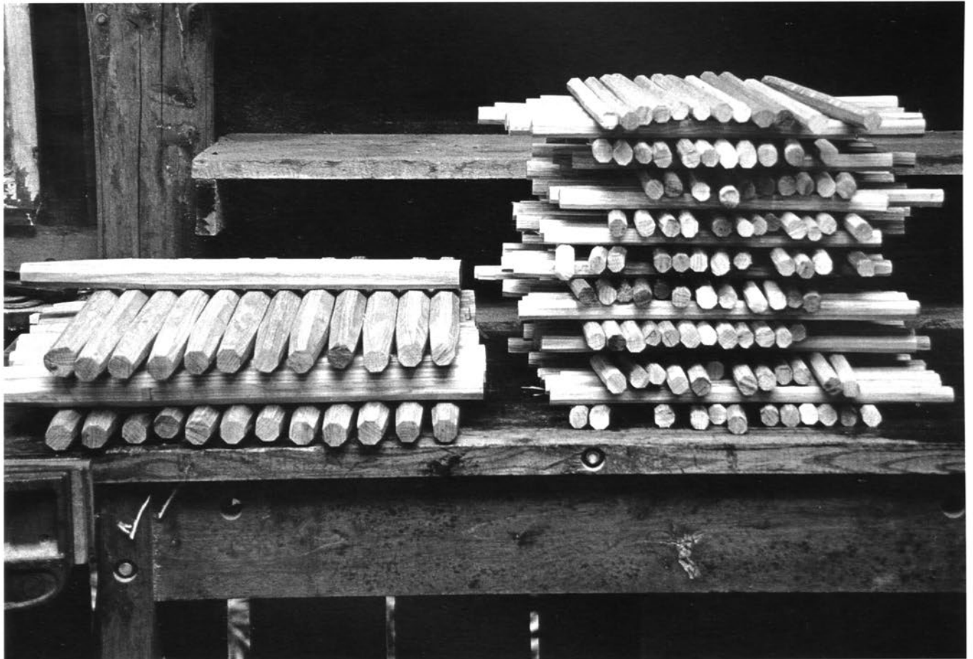
Air drying “chairmaker’s gold.” Shaved front posts and rungs for seven or eight ladder-back chairs. The front posts are tapered at the foot end. All are octagonal in section.
