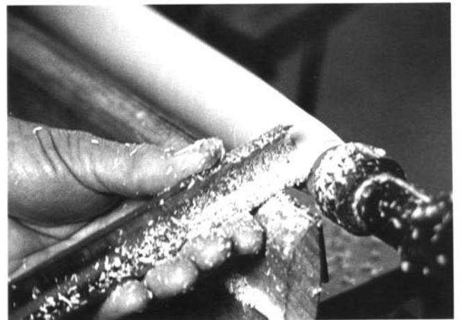
Shaping the taper with a 1-inch roughing gouge, a safe, easy tool to use
