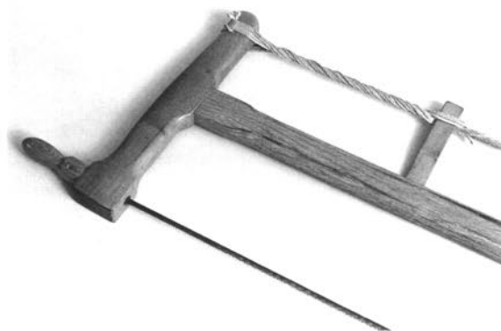
Shop-made bow saw, with knobs for rotating the blade
