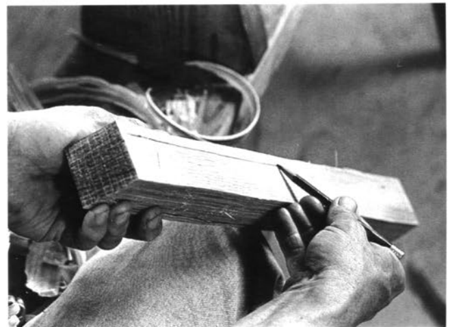
Penciling lines 3/4 inch from the common arris of a dressed plane—use your hand as a marking gauge.
