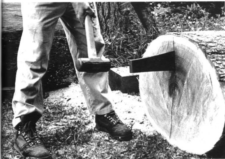
Using a flat, narrow-angle starting wedge to start the split. The handle of the 8-pound sledge hammer has been cut down to 24 inches.
