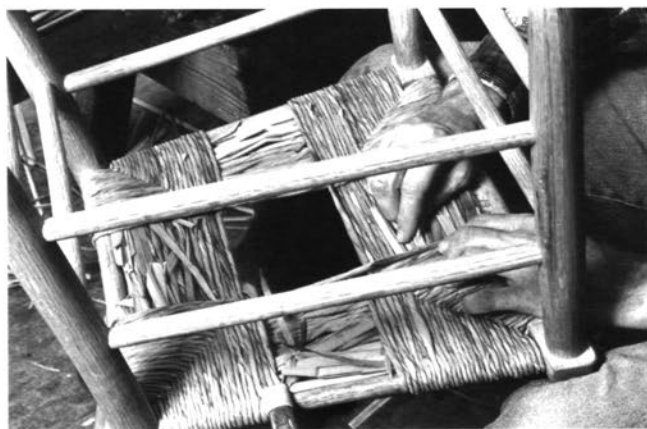
Spreading larger scraps of stuffing across pairs of corner pockets as the gap closes in
