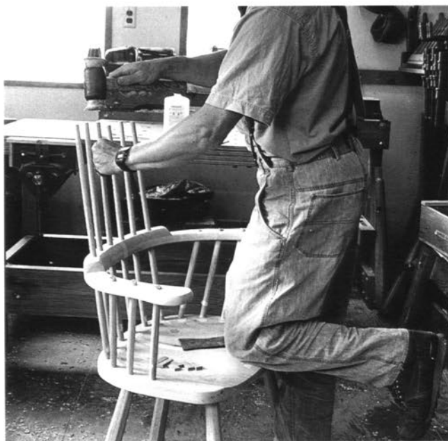
Seating the sticks into their mortises with a mallet
