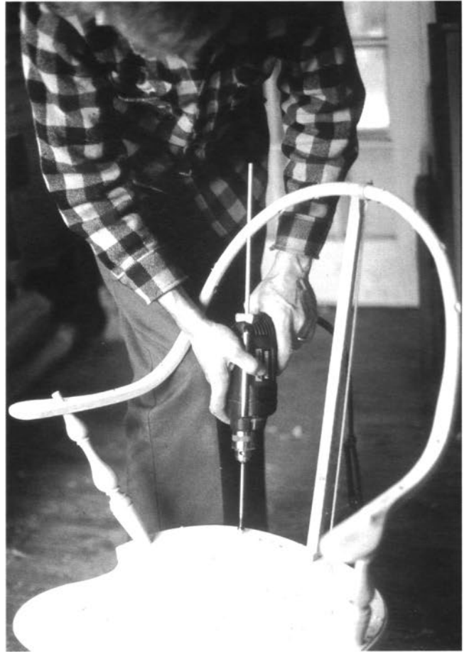
Dave Saucyer boring spindle mortises in the seat deck with the back box in place
