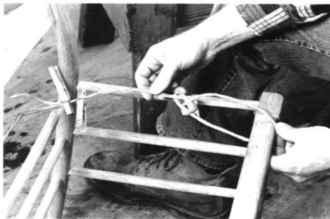
Chairmaker Tom Donahey's rush technique begins by wrapping a loop of twisted cord around the left end of the front rung. The knot is a bowline.
