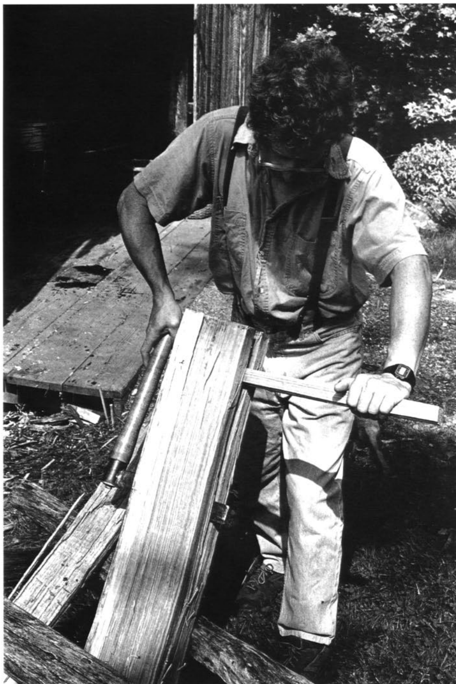
Placing a piece of scrap behind the split, so that the froe can be moved forward into the riving
