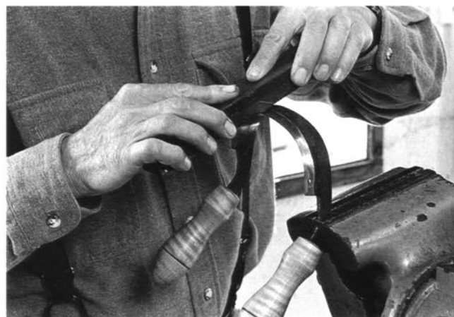
Polishing an inshave with a 4,000-mesh water stone. Rub the stone lengthwise along the bevel.
