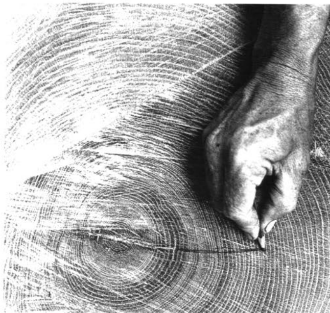
Before splitting a log, pencil a radial splitting line that extends from any pre-existing split.
