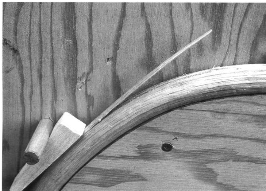
Example of a tension failure on a Windsor bow. The strip can be glued back.
