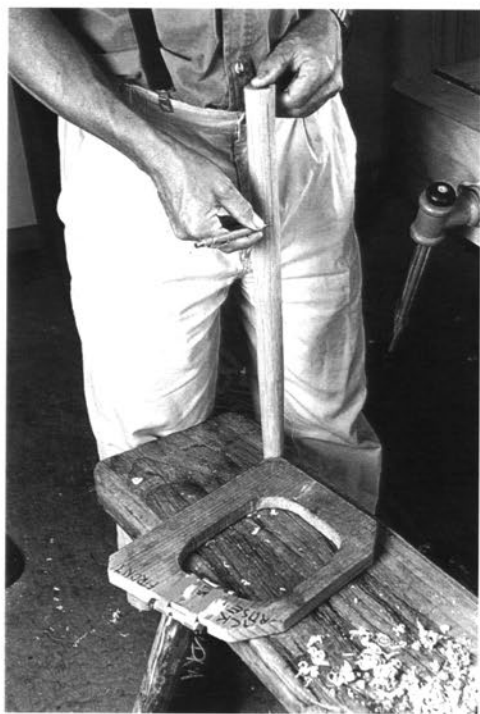
Locating the right front leg at its corresponding position on the potty seat, lining up the penciled line with the potty seat's right side
