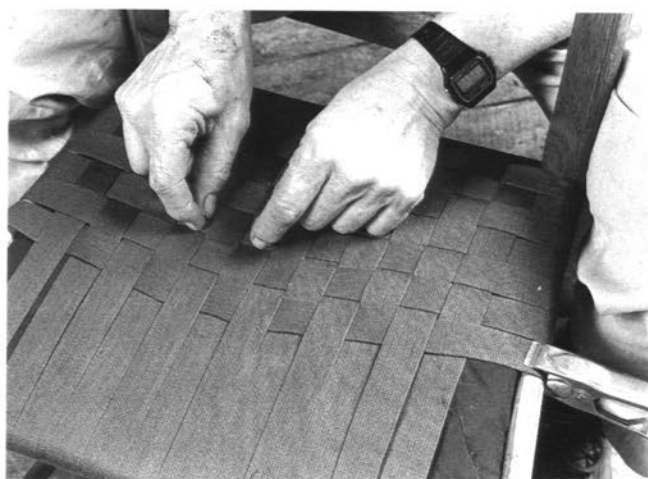
Pulling the middle section of the weft toward the back rung to keep the weave straight
