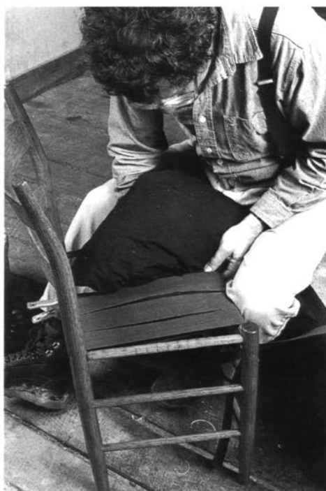
Inserting the stuffed envelope when the warp is about half complete
