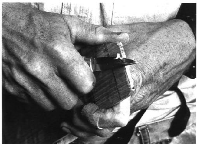
Cutting a chamfer around the ends of the slats with a sharp knife to help prevent jamming when the hot slats are fitted into their mortises. The lower slat corner has been cut off.
