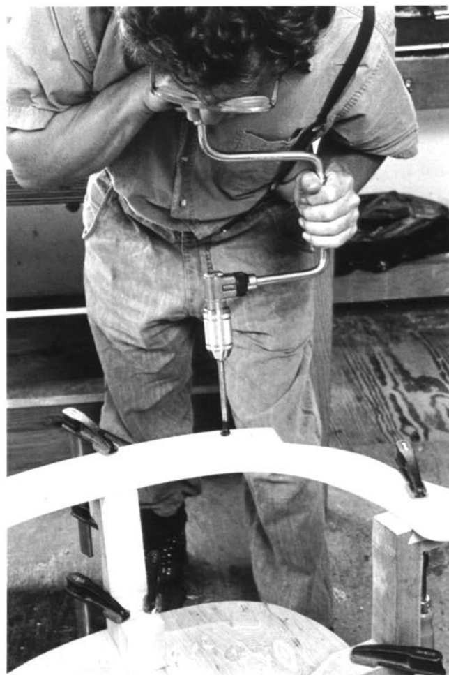
Boring stick mortises with the bow secured in place on the boring fixtures
