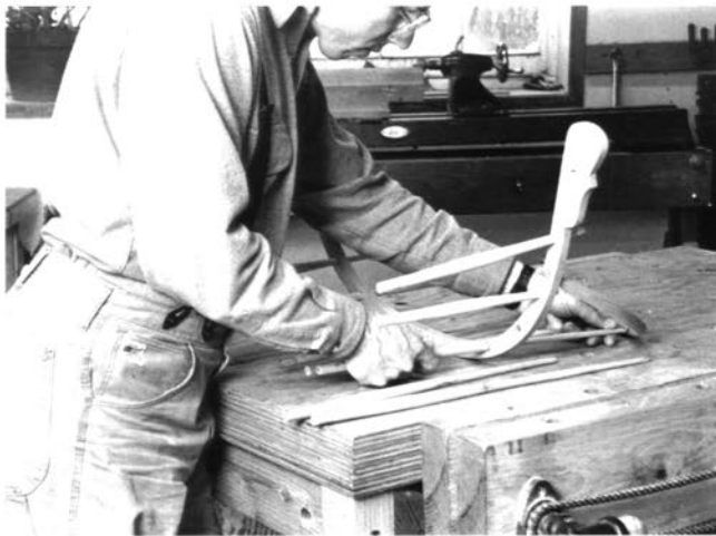
Fitting the long spindles into slightly tapered mortises in the arm bow
