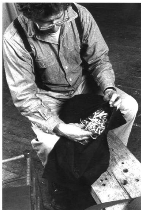
Packing spokeshave shavings into a simple cloth envelope to stuff into a Shaker-tape seat
