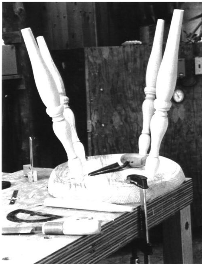
Comparing sets of leg angles as the seat mortises are reamed. The plank runs side to side on this wide, oval-shaped seat.
