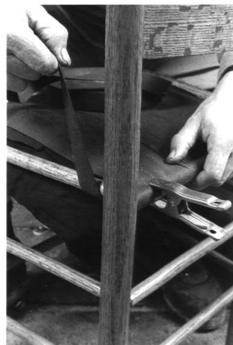
Wrapping the tape under the post and over the adjacent side rung when the warp is filled in, before weaving the weft
