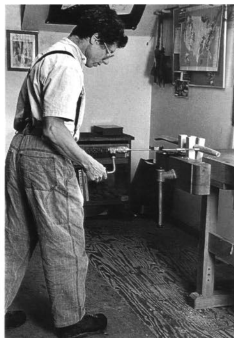
Boring a mortise. Keep the boring rig level while boring all three mortises.
