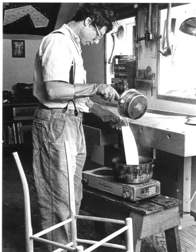
Slowly ladling boiling water over the slats. Rotate and end-for-end the slat to distribute the heat evenly.
