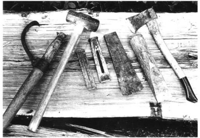
Log splitting tools, left to right: cant hook, 8-pound sledge hammer, two conventional steel wedges, narrow-angle starting wedge, glut, hatchet
