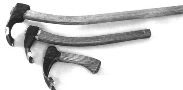
Hollowing adzes, from top: chairmaker's saddling adze with 30-inch handle, designed by the author; Swedish hollowing adzes with 20-inch handle and with short handle
