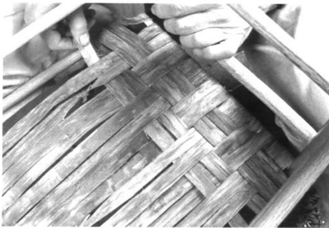
A double-row checker pattern on the underside of the seat. The splice on the next warp row will be hidden by the weft passing over the knot.
