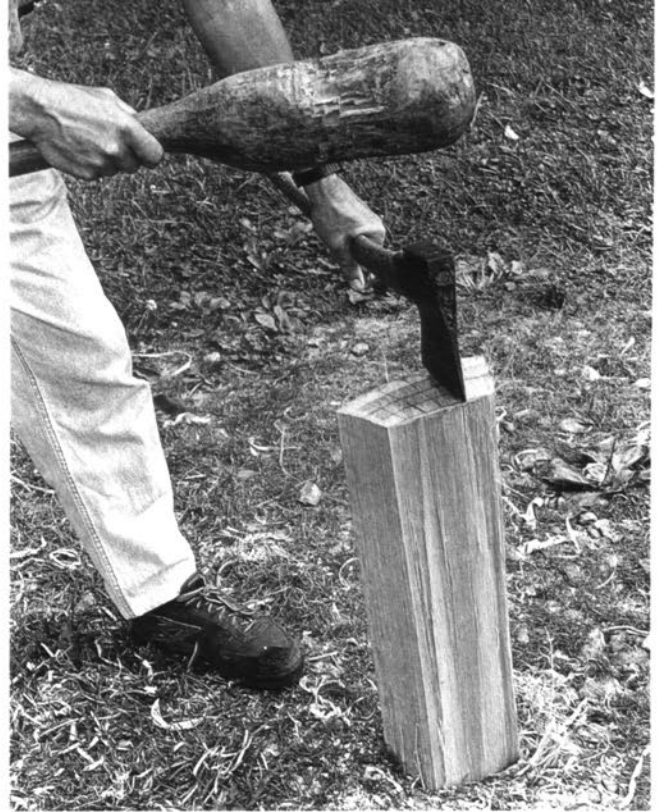
Striking the head of a polled axe with a dogwood-root maul, an excellent method for riving medium-sized pieces
