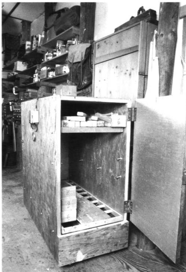
A plywood kiln for drying Windsor boxes, turnings, and spindles
