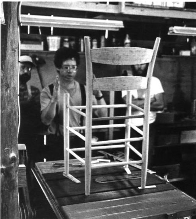
Double-checking the measurements with a visual survey. Variations in the bend of the back posts may suggest tilting the chair slightly.
