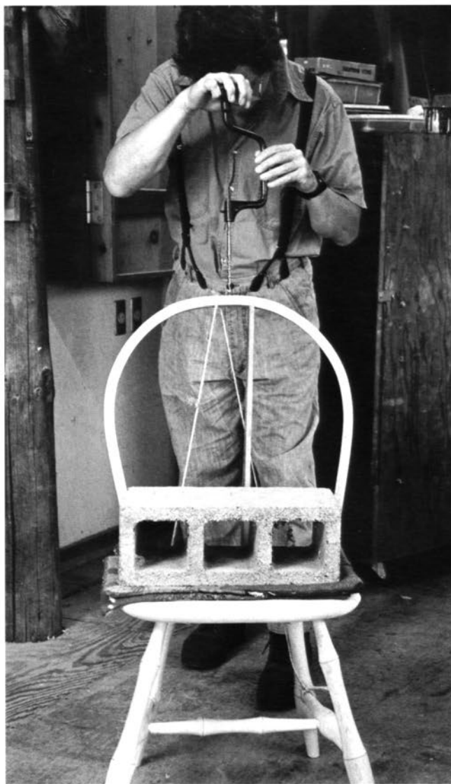
Boring the 5/16-inch mortise for the center spindle. Hold the bow steady by wedging a stick between the seat and bow and by twine that pulls the bow downward against the stick. The cinder block prevents the chair from moving.
