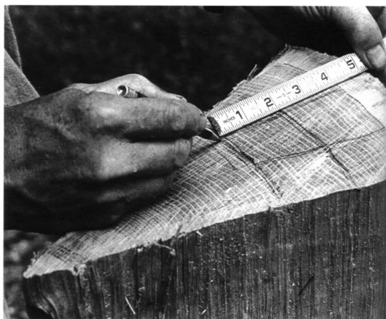
Pencil layout for the posts. I also hope to squeeze a bonus post or two from the inner heartwood.
