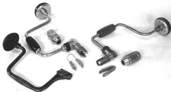
Braces, from left: late nineteenth-century Spofford brace; bit brace with a universal chuck; bit brace with alligator chuck
