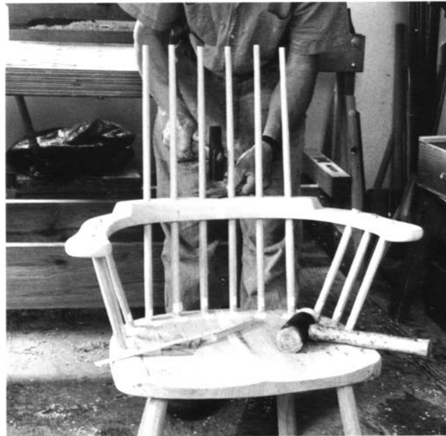
Making sure the arm bow is properly positioned, after the sticks are in place. Check from front and side views.
