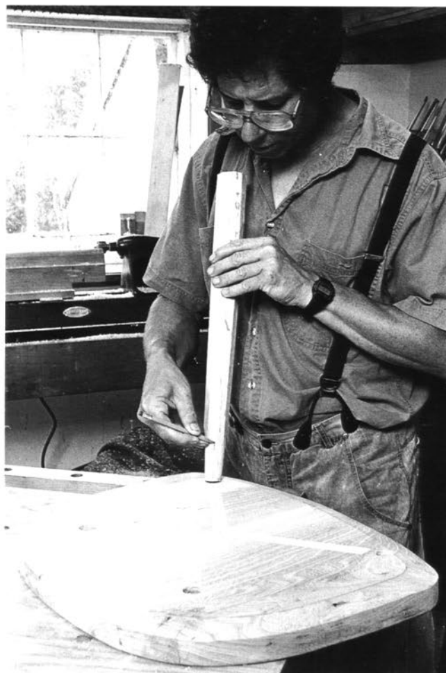
Identifying each leg and its mortise by penciling tick marks on matching parts so that alignment will be consistent during trial fitting and final glue up
