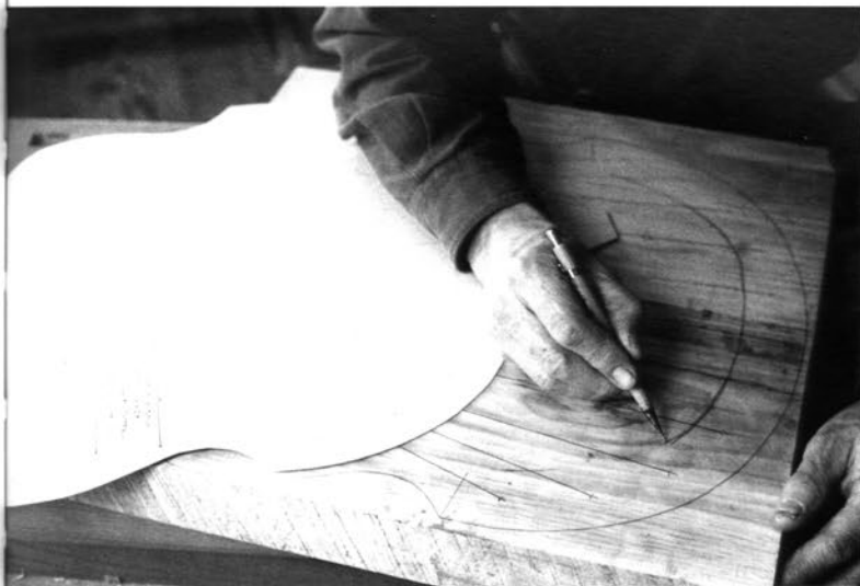
Transferring the outline from the seat plan in figure 9.4, then drawing the spindle deck on the seat plank
