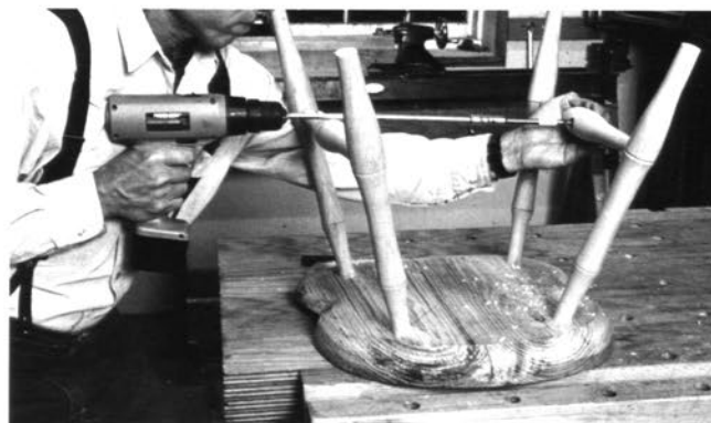
The direct method for boring the medial stretcher mortises in the side stretchers. Rotate the target stretcher slightly, so that the center mark aligns with the upper tangent of the sighting stretcher.
