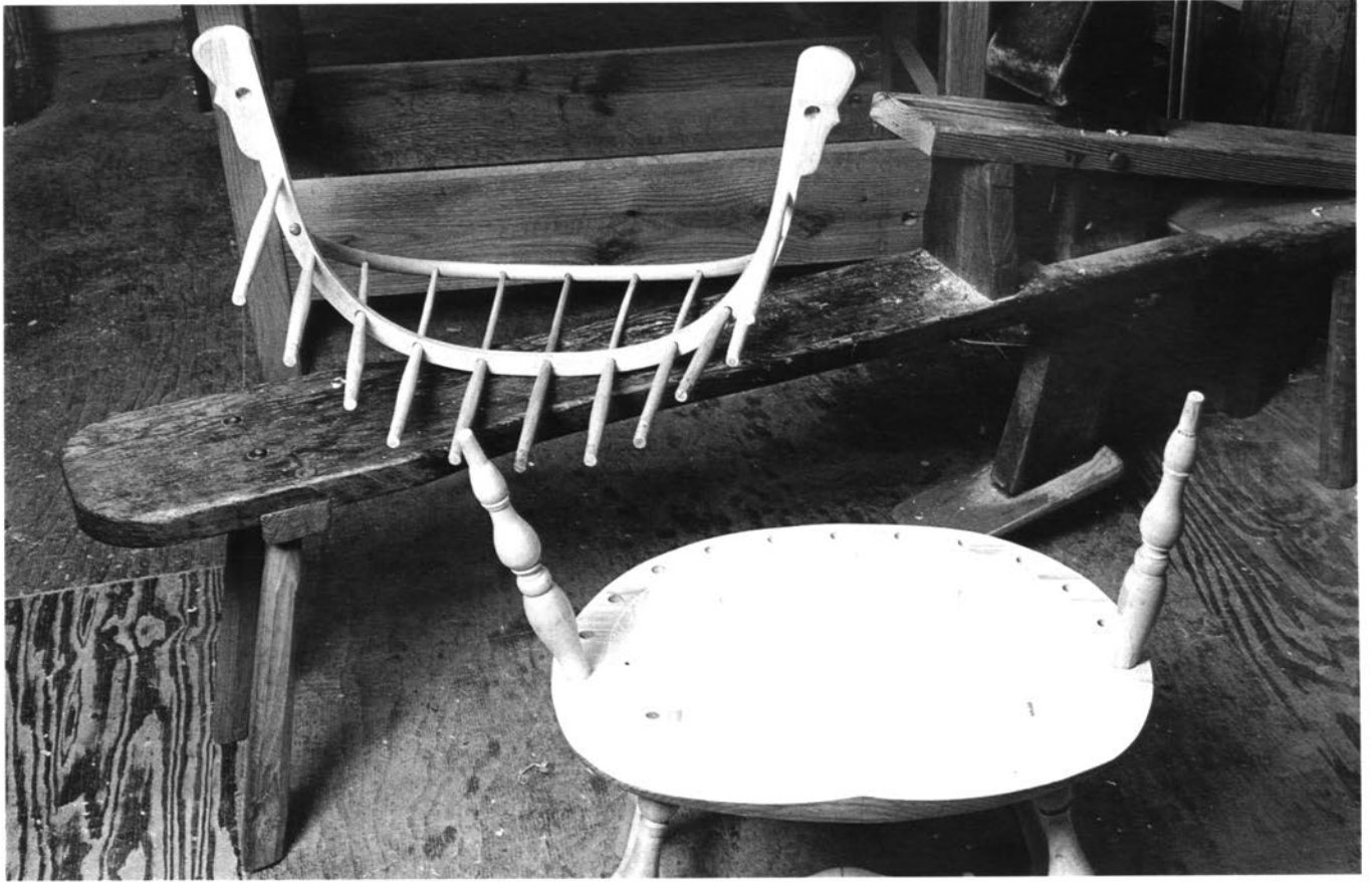
The final test assembly. Put the spindle/bow unit together; then fit the base of the spindles into the seat mortises.
