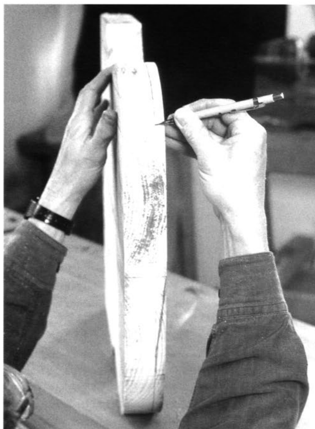
Drawing saddle line #1 a half inch below the arris around the front flanks of the seat
