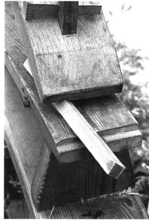
Angling the billet onto an arris, to shave the square into an octagon. Note the small V-notch cut into the bottom of the shaving-horse jaw.
