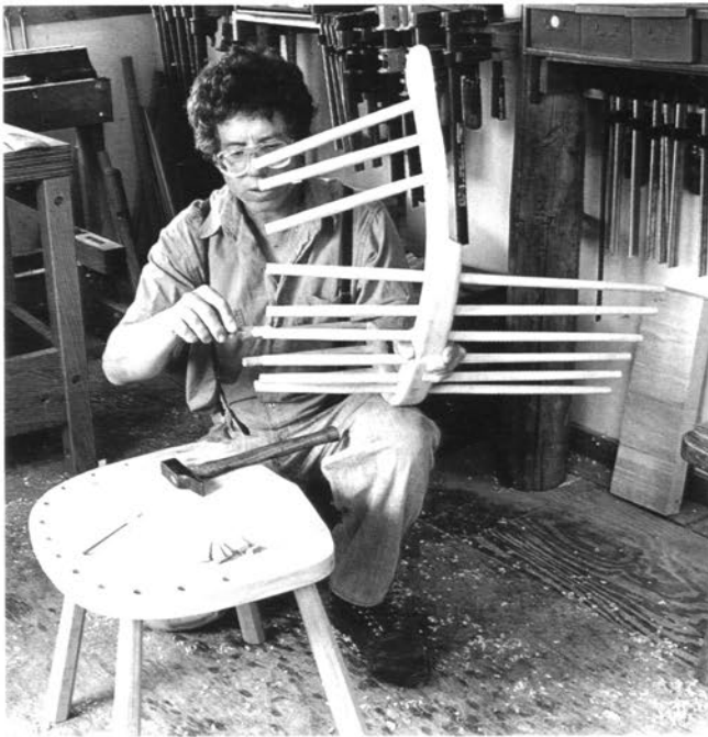
Gluing all the sticks to the bow, the first step in assembling the chair
