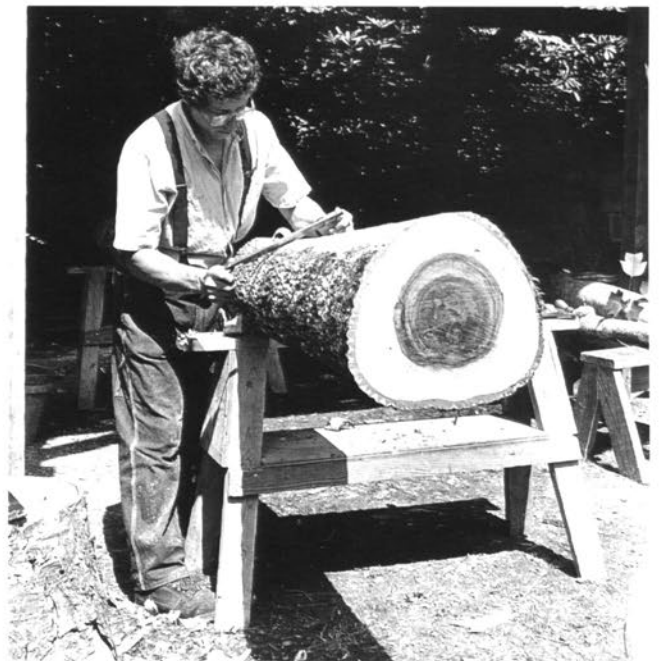
Shaving hickory bark with the log at comfortable work height
