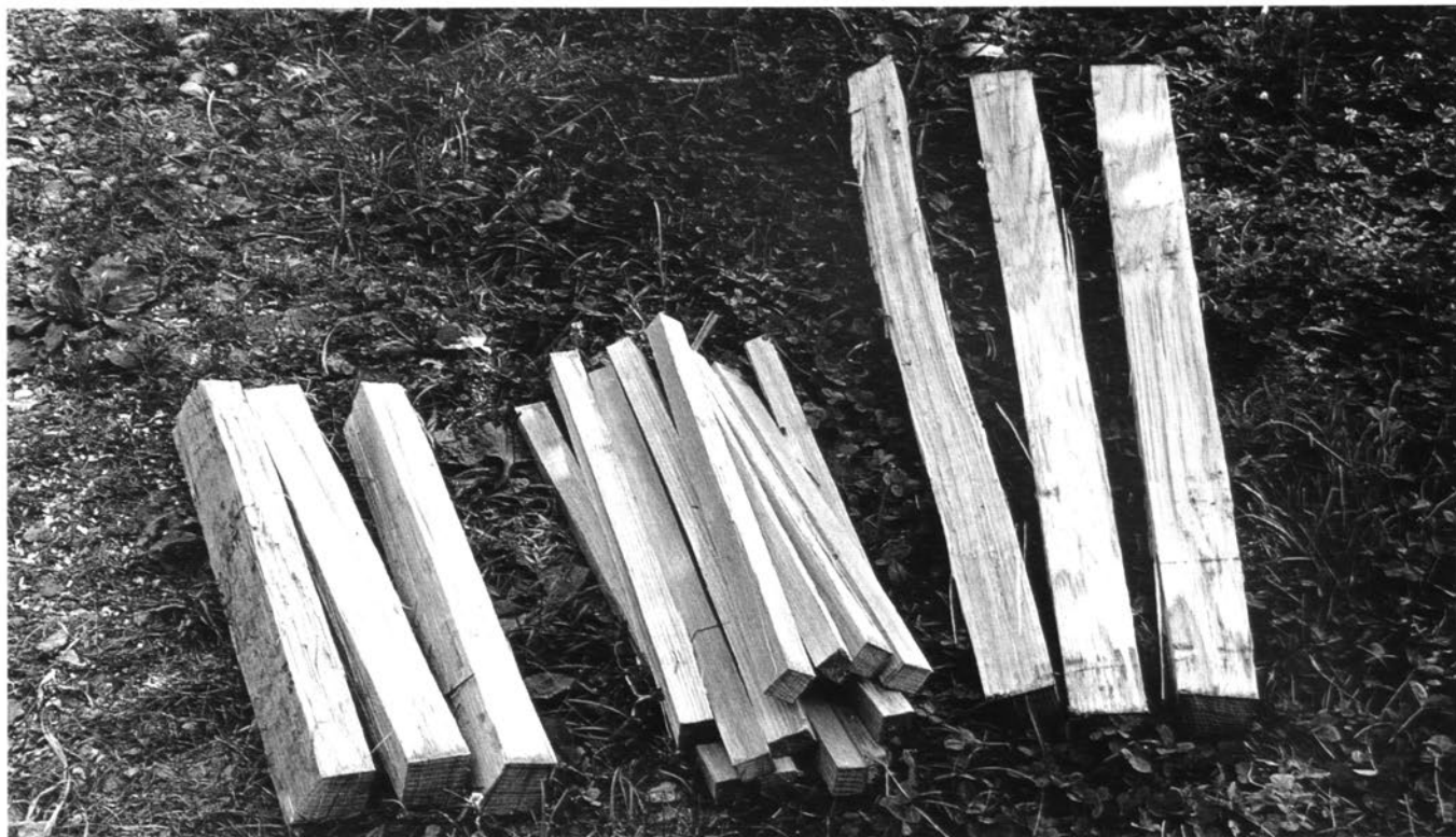
Rived billets for one chair, left to right: three front posts, sixteen rung blanks (all overlength), three rear posts
