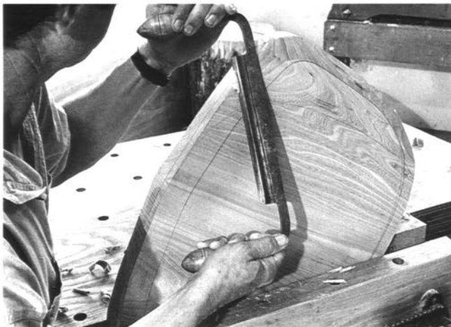
Working with the drawknife on the seat bottom, using extreme slicing and skewing action cutting into the endgrain at the front of the seat
