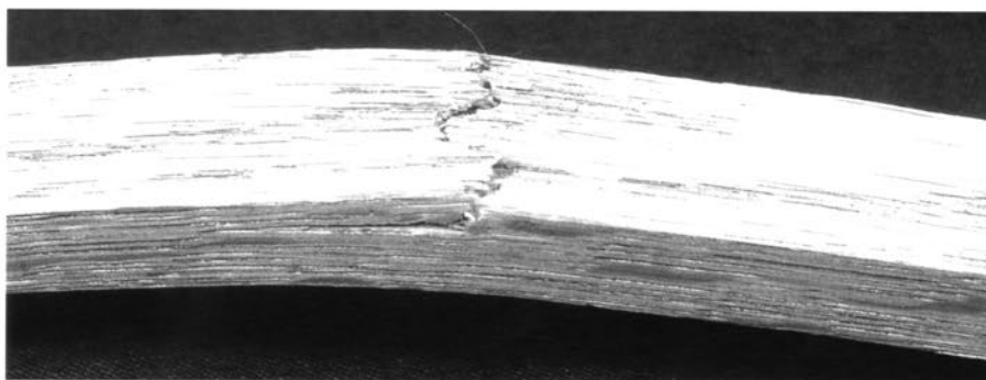
A ragged fissure failure such as this is usually caused by incipient decay. Discard the piece.
