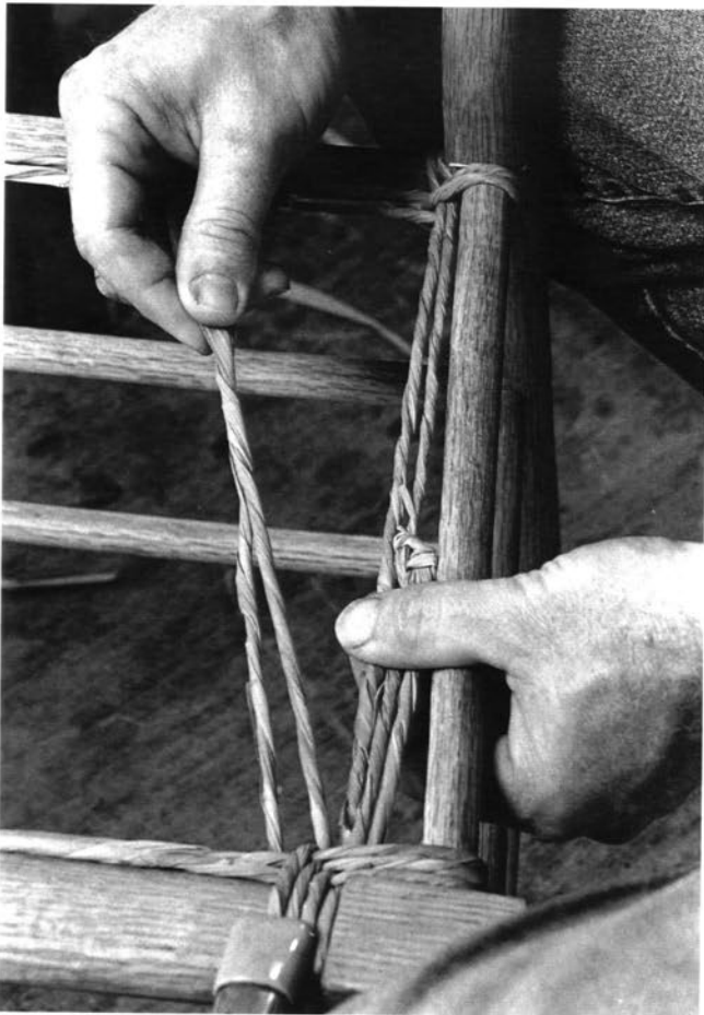
After crossing the front of the seat, the two cords are reunited along the opposite side rung.
