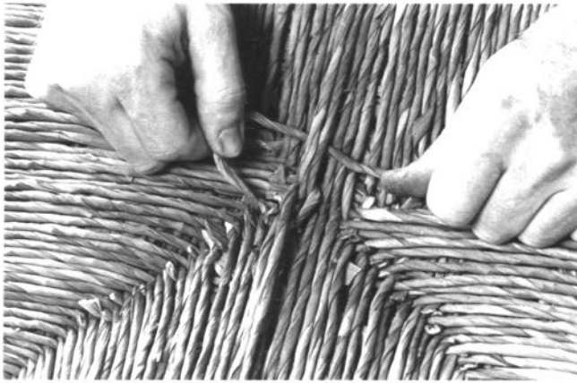
Wrapping a loop or two of cord around the center of the seat bottom to finish. This photo shows the butts of new leaves added into the rope at the diagonal lines.
