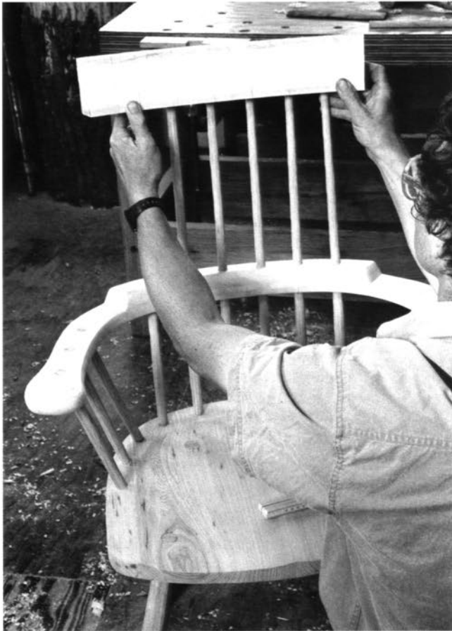
Positioning the comb. Experiment with different heights and spreads for the sticks.
