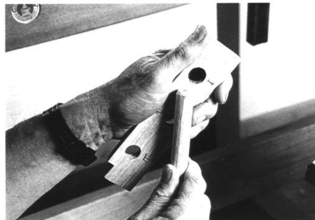
Using hole #1 on the tenon-sizing gauge. Note small smears of pencil graphite on the rung high points.
