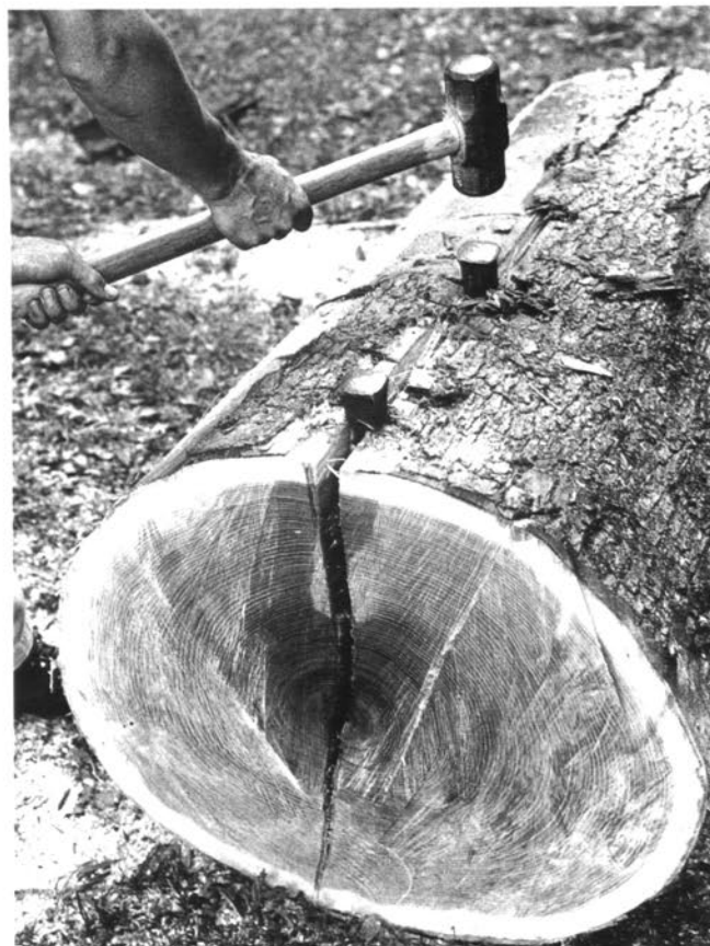
Leapfrogging a pair of wedges into the developing crack. Always leave 1 inch of wedge head above the bark.
