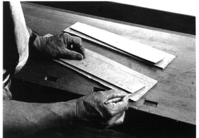
Using slat dummies as patterns to determine the length and end angle of both slats
