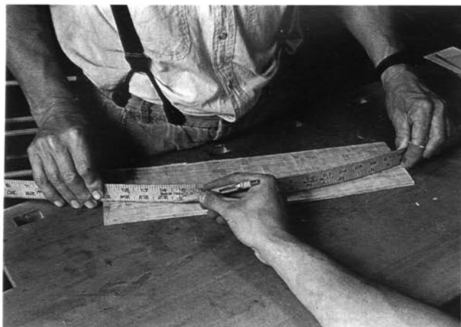
Arching a narrow ruler across the end and midpoints of each slat to create the curved upper edge. A helper is useful, but not necessary.
