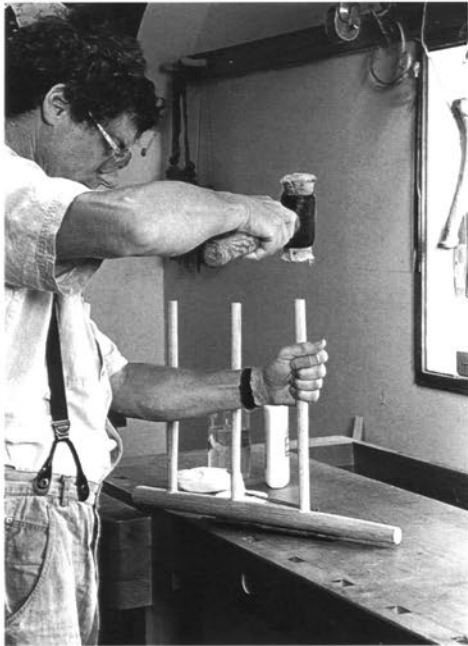
Pounding rungs into the post mortises with a rawhide-and-iron mallet
