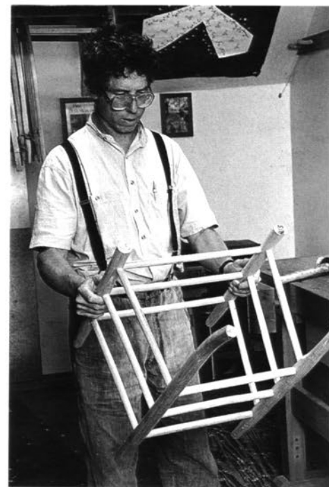
Looking across the frame of the assembled chair to see if the front and rear rungs are parallel. A side view shows if the bends in the rear posts line up.
