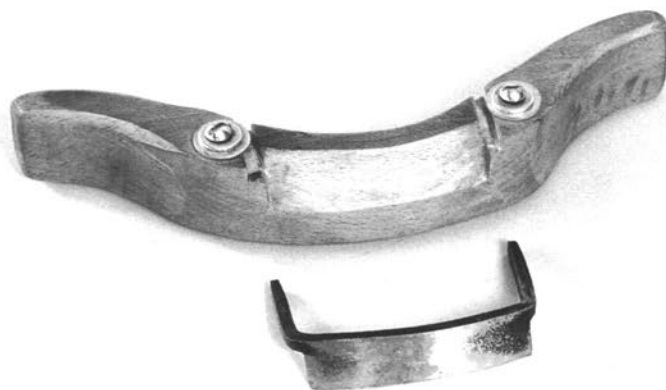
Shop-made travisher, with 01 tool-steel blade
