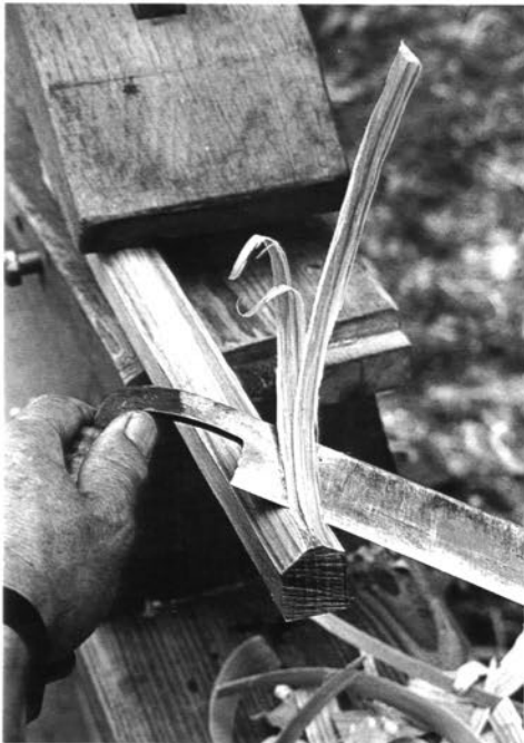
Taking an angled shaving on the side opposite the penciled line. Since the rung will eventually be round, you can guess how far to shave on this side of the riving. Note the resulting "gable roof" on the ray plane.
