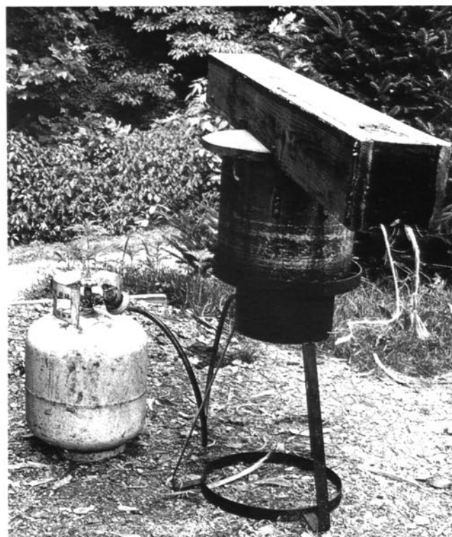
Country Workshops steamer. The heat source is propane, coupled with a burner made for outdoor cooking. For indoor steaming, use an electric hot plate.
