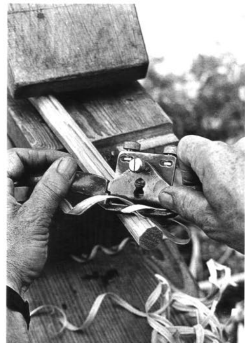
Spokeshaving the square rung billet into an octagonal section. Skewing produces a smoother surface and causes the shavings to eject to one side.
