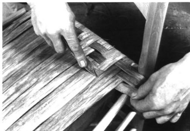
The third row of weft: Pass under two rounds of warp, then over two...
