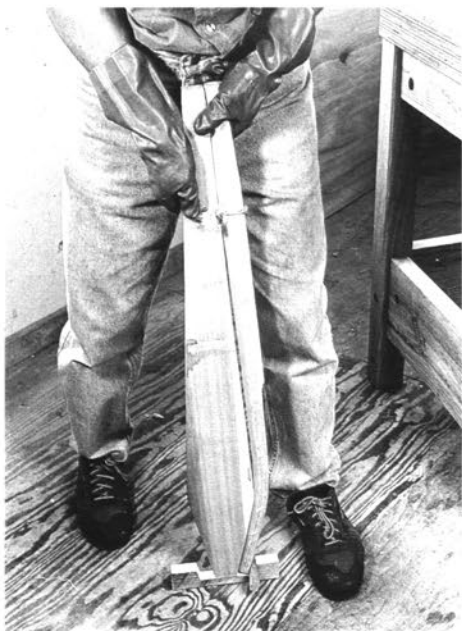
Holding the post against the bending form with a loop of twine. The upper end of the post (pictured upside down) was slightly undersized, so a wedge was driven between the post and retainer on the floor. The first loop of twine will be removed for the second post, if there is one.
