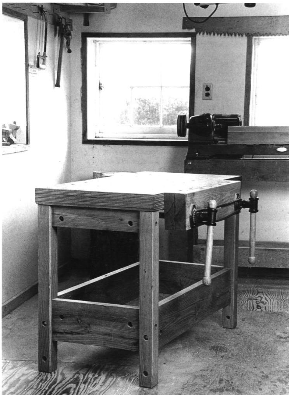
My design for a chairmaker's workbench. The vise on the right will hold a chair seat between the twin screws, which are 28 inches on center.
