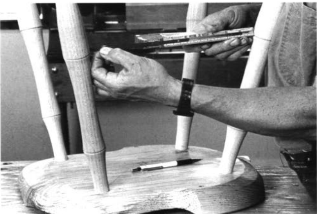
Determining the shoulder-to-shoulder length of the side stretchers with a folding rule and extension. Add 1/16 to 1/8 inch, depending on the tightness of the prefitted tapered leg joints in the seat.
