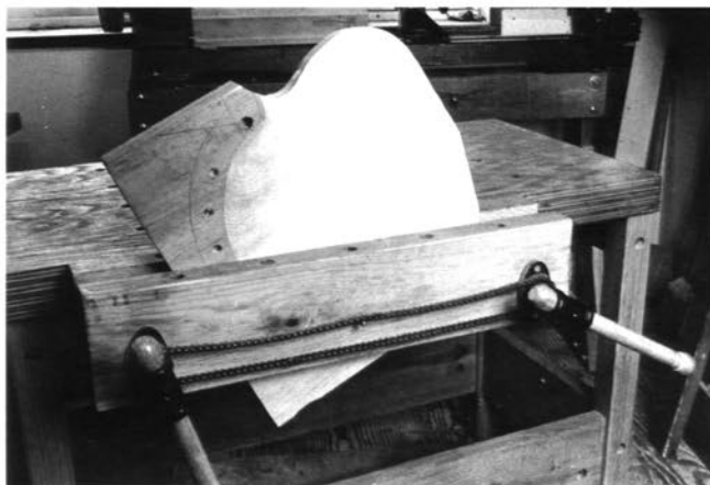
A twin-screw vise that will securely hold the largest Windsor chair seats. This chain-linked vise is made from a kit. You can also make a wide vise with independent screws.
