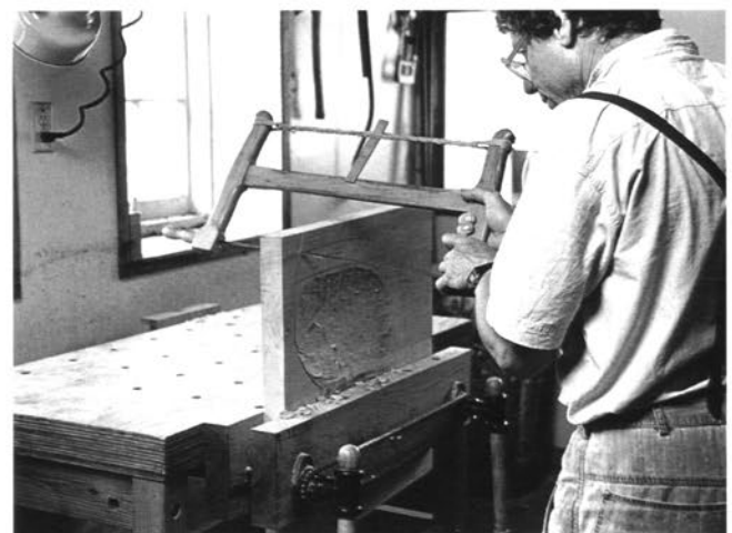
Sawing the front edge of the seat with a shop-made bow saw. The knobs at the bottom of the handles can be rotated to change the angle of the blade in order to saw the seat outline.
