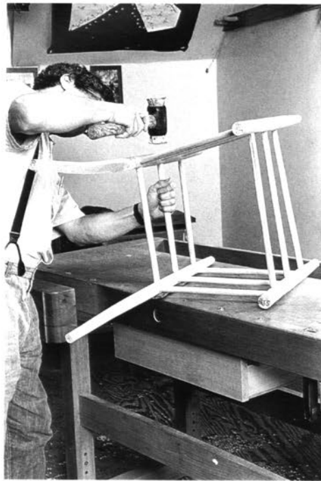
Starting to pound the left panel onto the front and rear rung tenons
