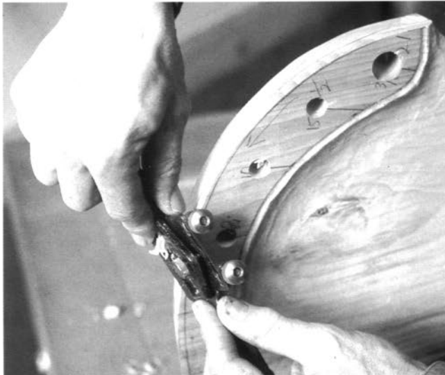
Chamfering the back edge of the deck with a spokeshave
