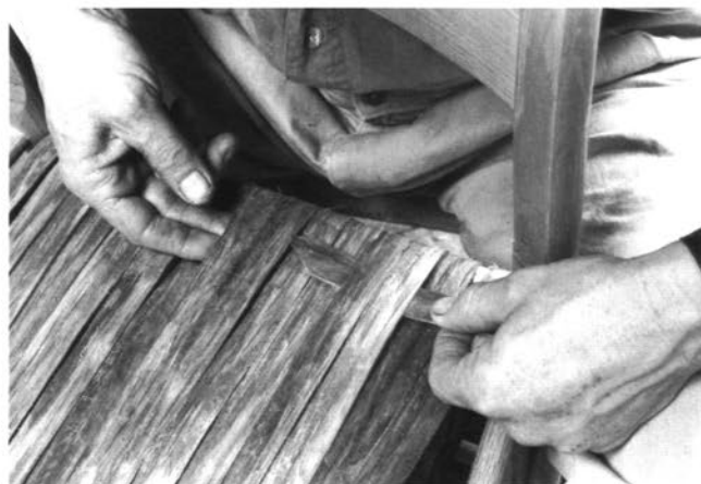
The first row of the herringbone weft on the upper side of the seat: Pass over two rounds of warp, then under two...
