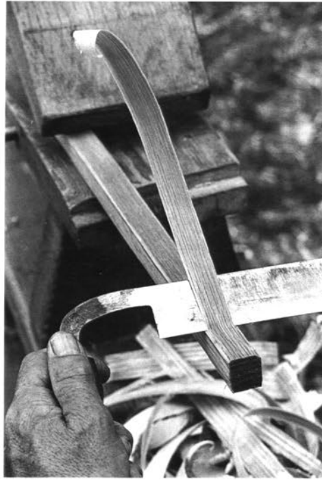
Flattening the gable roof. The rung blank is now very close to 3/4 inch in width across the growth ring plane.
