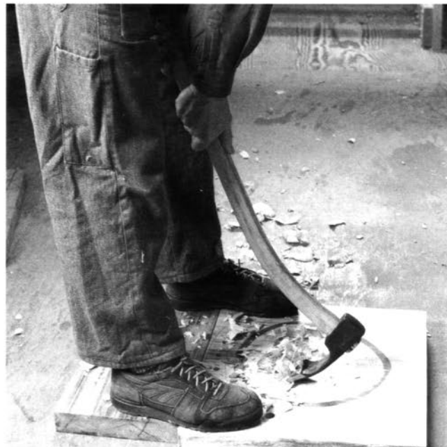
Adzing the seat is basically the same as doing the stick Windsor seat, although the outline of the adze zone differs slightly.
