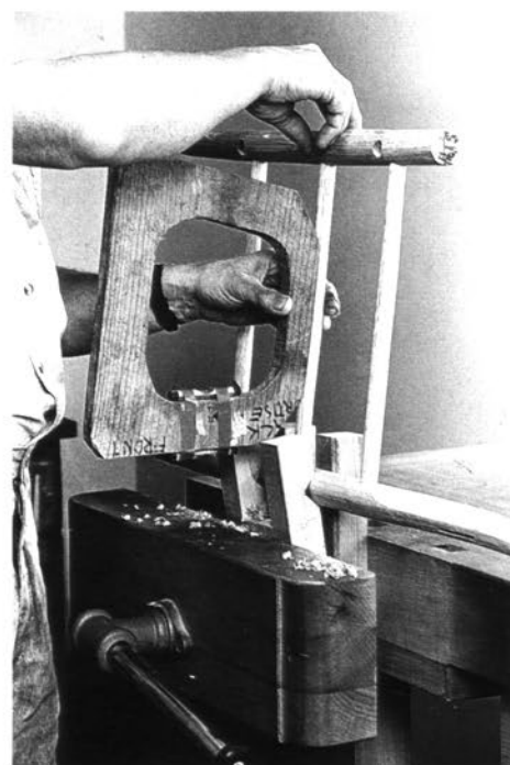
Adjusting the angle of the side panel using the potty seat. When you bore the rear-post rung mortises, the side panel must be at an obtuse angle.
