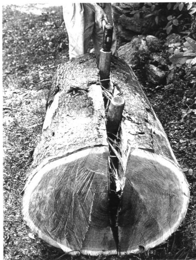
Using gluts to widen the crack. Never put your hands into the opening; the log is now a giant spring.
