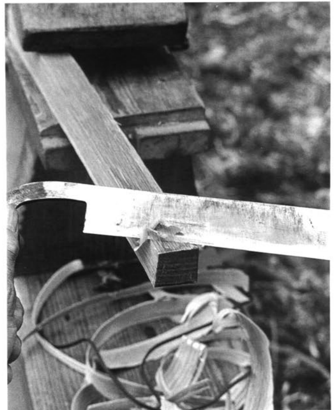
Shaving on the growth-ring plane surface before thickening. Note the skew angle of the drawknife.
