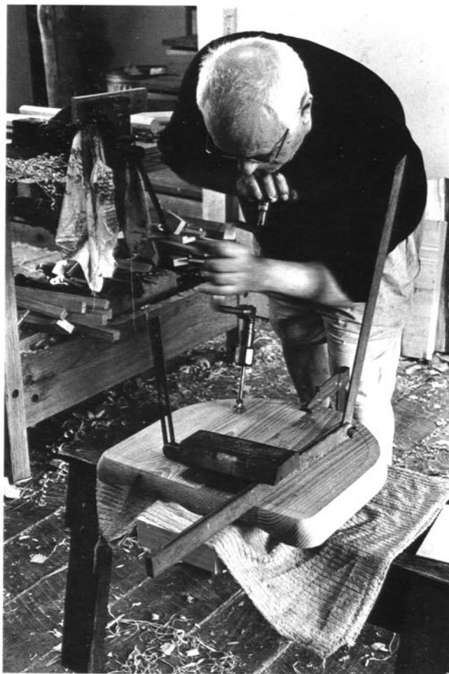
John Brown boring cylindrical leg mortises at Country Workshops, with his brace positioned at a compound angle aligned with the legs of both bevel gauges
