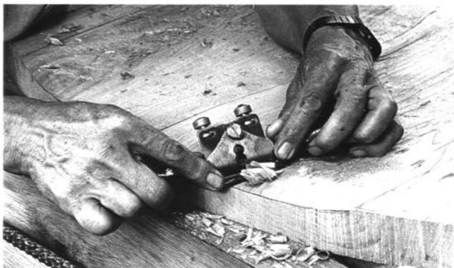
Using a spokeshave to shape the front edge of the seat and blend the convex rolled front into the concave inshaved area
