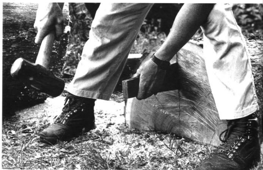
Splitting down the center of the half log, on the way to splitting it into four bolts, each an eighth of the original log.
