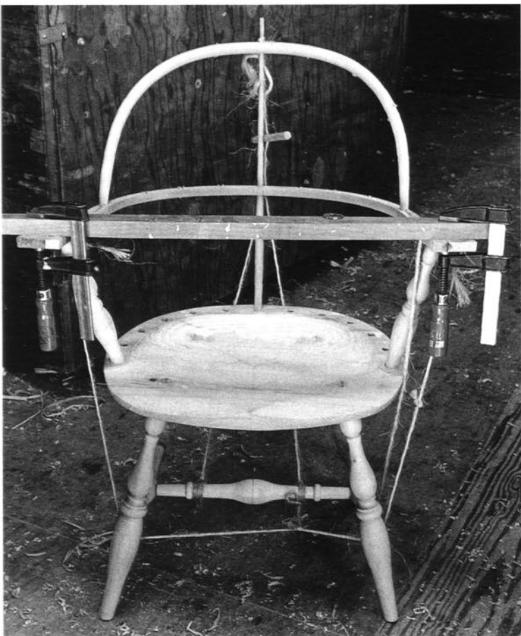
Preparing to bore spindle mortises in the back and arm bows. The board clamped across the arm bow prevents the hand pieces from twisting out of alignment.
