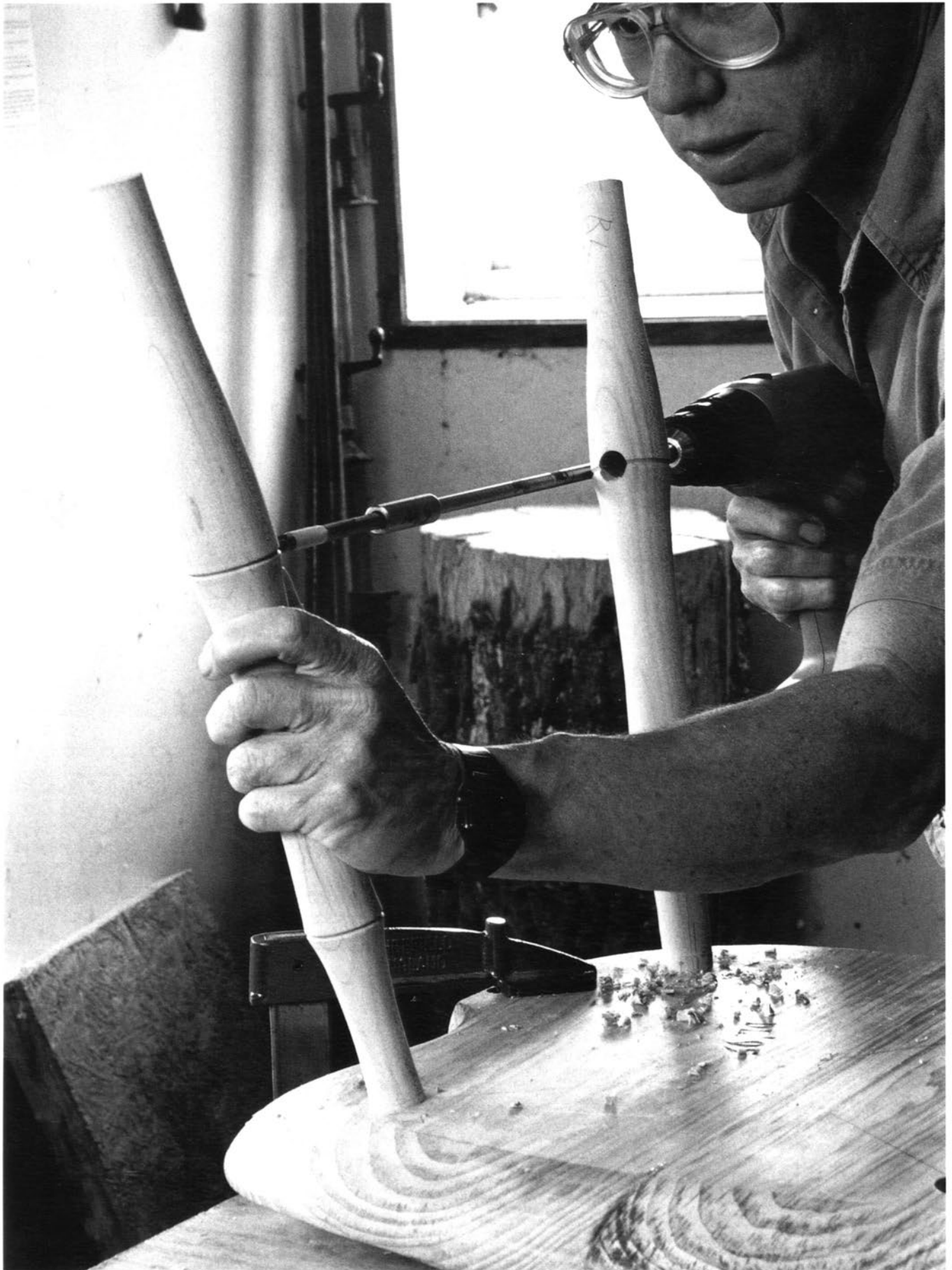
The author, boring stretcher mortises in the legs of an American Windsor
