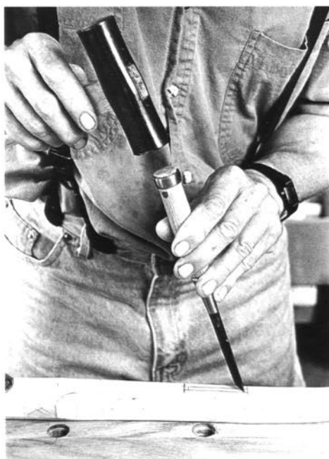
Starting the mortise by scoring the penciled outline
