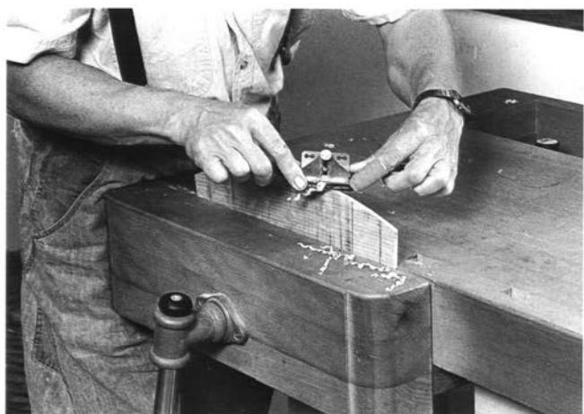
Roughing out the upper curve of a slat with a drawknife
