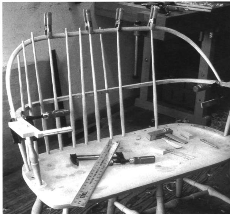
Experiment with the spindle spacing—the critical visual factor in a Windsor settee—before committing to boring mortises.
