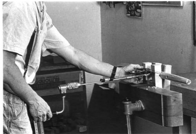
A rear post in the horizontal boring fixture. Use a combination square to align the boring rig perpendicular to the length of the post.
