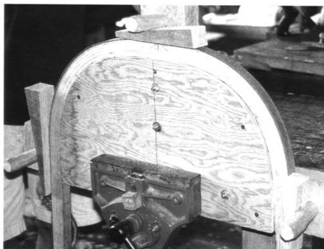
Steel bending straps help prevent tension failures on heavy bows.
