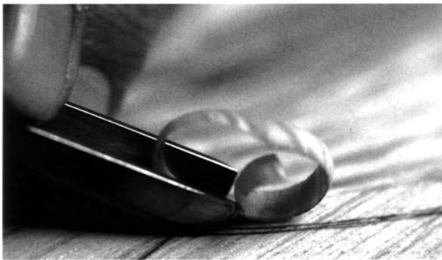
Carving the gutter, continually wiggling the gouge left and right while advancing in small increments
