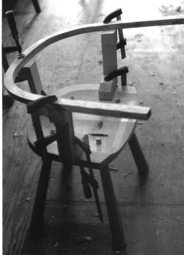
Using the boring fixture on a bent-bow low-back
