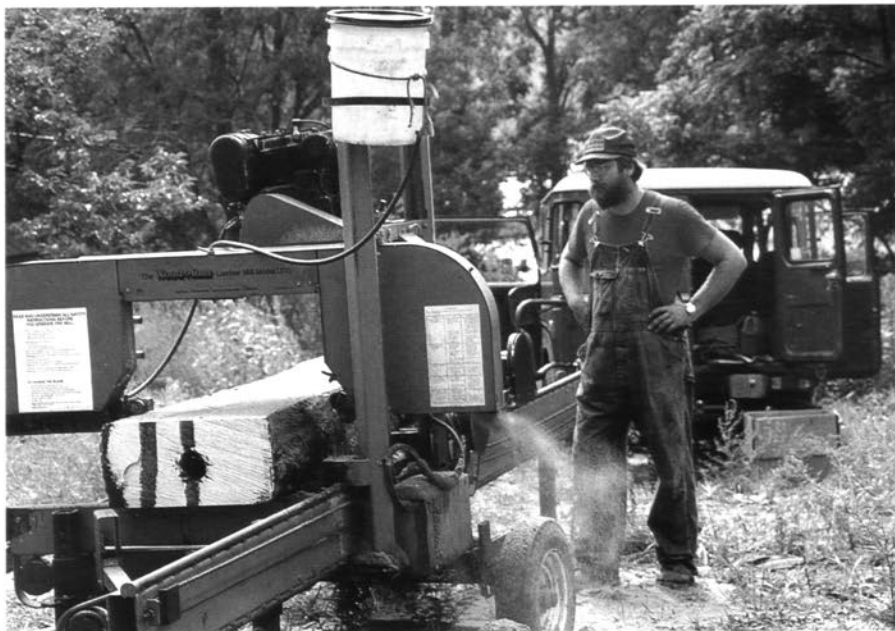
Portable band mills brought to the site cut slowly but accurately and can be operated by one or two people.
