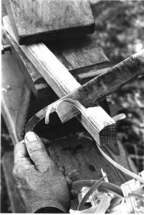
Taking an angled shaving down to one of the penciled lines. The ray plane is facing up.
