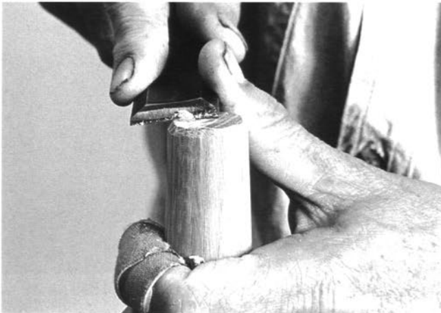
Trimming the top of a post by taking slicing cuts with a very sharp chisel. The arris has already been chamfered.
