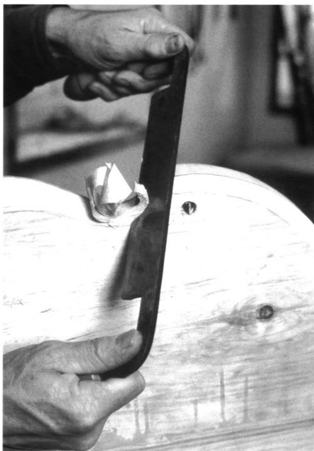
Drawknifing the pinched waist by taking a slicing cut while rotating the blade into the curve, with the drawknife bevel down. Make several downhill passes into ascending fiber, cutting from opposing high points of the curve.
