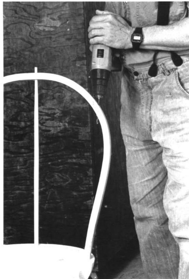
Boring the steep mortises at the extreme flanks of the bow with an electric drill and the chicken method.
