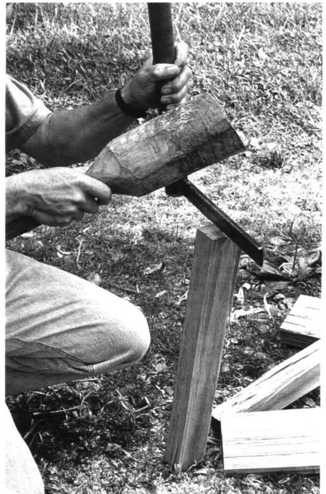
Riving small pieces with a froe and froe club, usually done on the shop floor, or on top of a chopping stump
