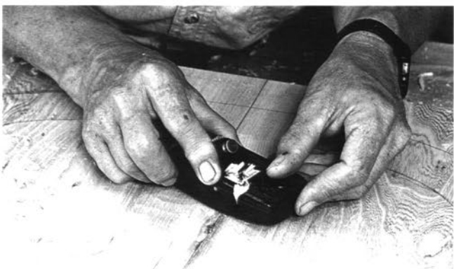
Smoothing the concave slope below the flat deck with a small plane whose sole curves lengthwise and crosswise. A travisher can also work this area.
