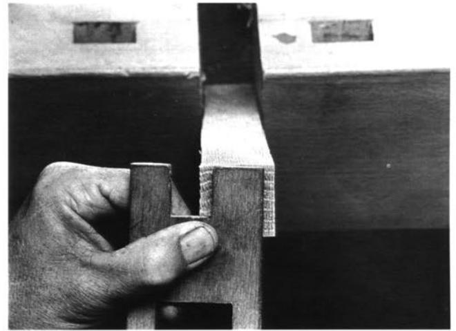
Using a 1-inch-wide strip to center the 1-inch foot on the bottom of the post
