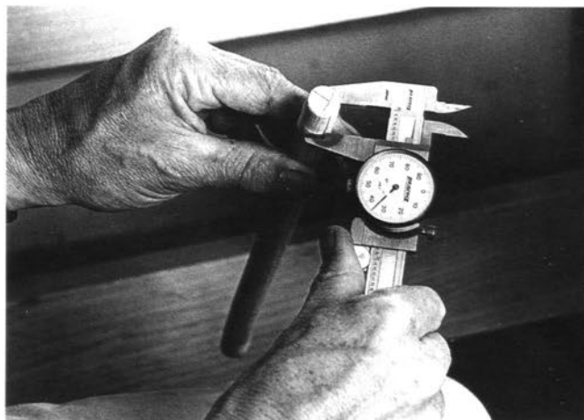
Checking tenon diameter with a machinist's dial gauge
