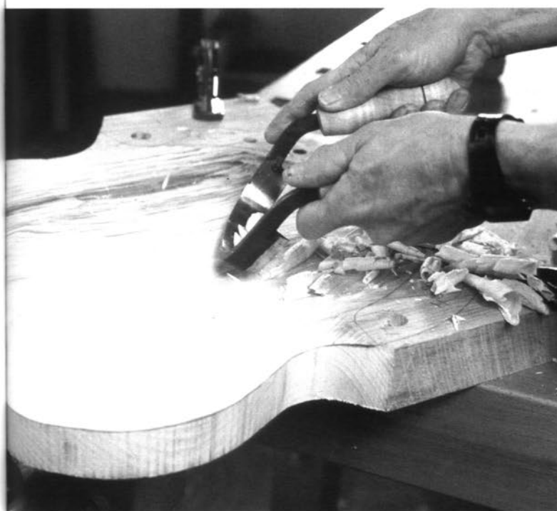
With practice, you can learn to use an inshave to quickly finish most of the seat surface. To take cuts into ascending fiber, you will need to read the grain continually.
