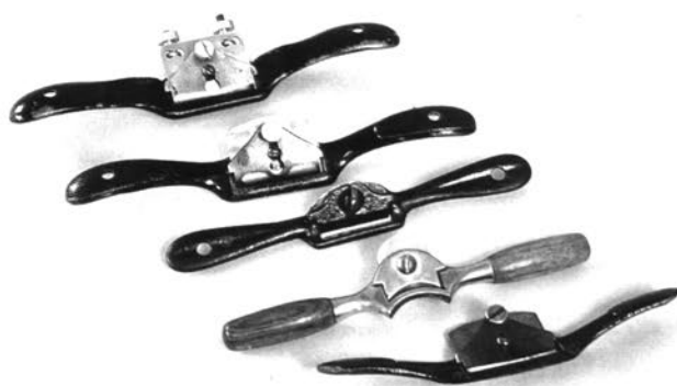
Spokeshaves, from top: standard spokeshave with flat sole and twin-blade adjusting screws; a basic spokeshave without adjusters holds blade setting better but is more difficult to adjust; a small flat spokeshave with excellent balance for shaving cylindrical chair parts; Brian Boggs's concave spokeshave, designed for finish work on post-and-rung chair legs; shop-made travisher made from a standard spokeshave.
