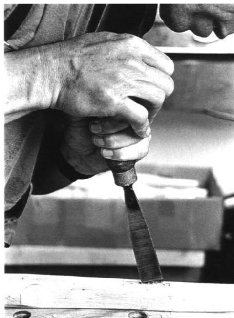
Cleaning the cheeks with the paring chisel. Use body pressure and a shearing (skewed) cut.
