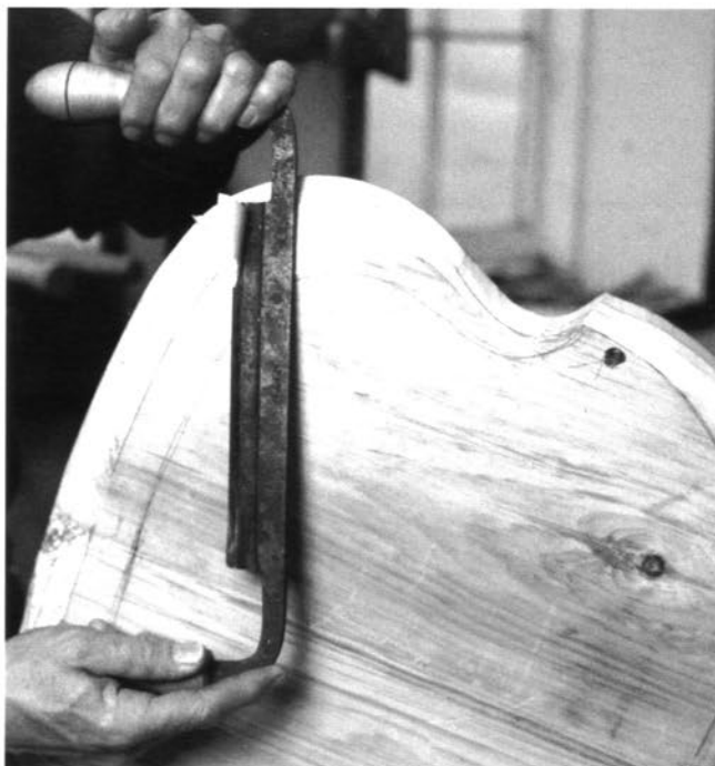
Extreme slicing and skewing to shave the end grain on the bottom of the seat, with the drawknife bevel facing up
