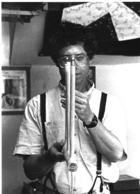
Checking across the tops of the rungs to see if they line up—it's important that the center rung is not longer than the upper and lower rungs. The misalignment to the sides will easily pull straight when the rear post is fitted.
