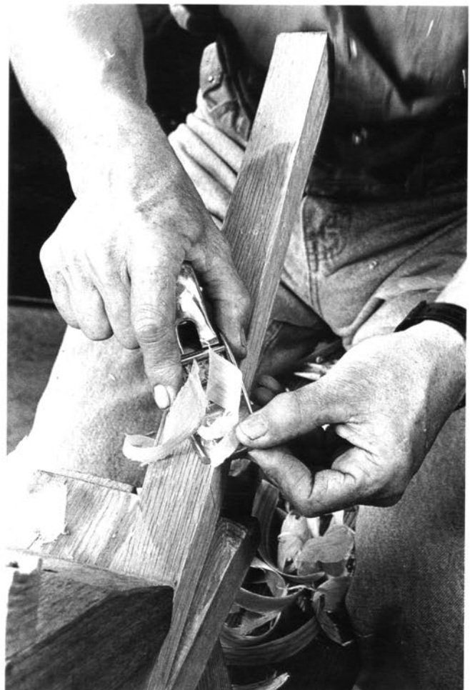
Shaving with a small block plane, very useful for straightening a curved post or dealing with wavy grain. Note the skewed angle.
