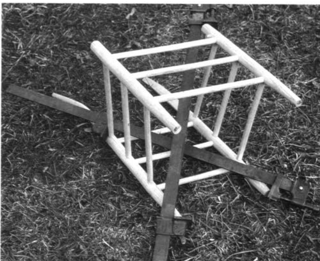
Remedial chiropractic can sometimes pull an unaligned frame into the desired geometry. Some frame irregularities can also be corrected when the frame is leveled and trimmed.
