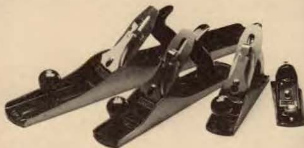
Left to right: try, jack, smoothing and block plane.
