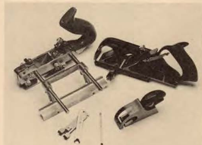
Clockwise from top right: rabbet, shoulder and combination plane with blades.
