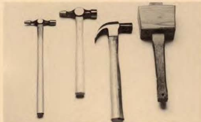
Striking tools used in woodworking. Left to right: tack, Warrington, claw hammer and wooden mallet.
