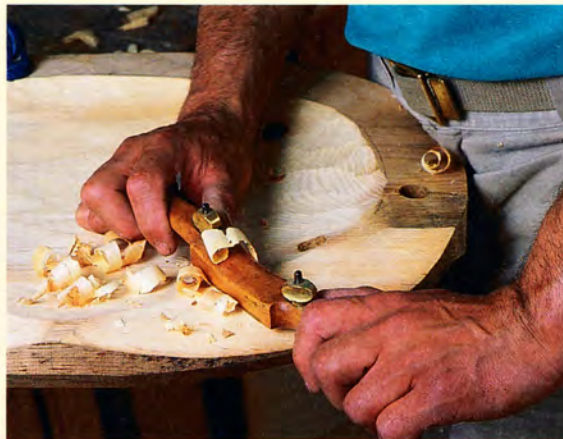
STEP 4: Remove gouges and ridges with spokeshaves.
