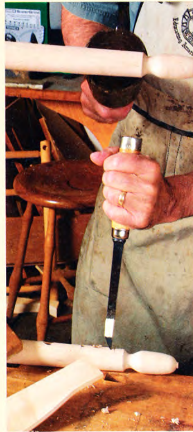
DETERMINE THE ANGLE of the mortise. Conover uses a mortising chisel to chop the mortises for the curved back slat. He rests the slat in place to set the proper angle for chopping (center). A piece of tape on the chisel marks the desired depth of the mortise (right) so that it can engage \frac{3}{8} in. of the tenon.
