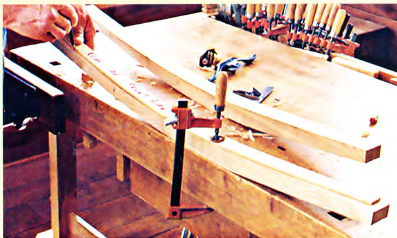
USING THE SIDE TEMPLATE , cut all of the legs from one wide 8/4 board to ensure uniform color (left). Lay out the legs for best grain orientation and strength (above).
