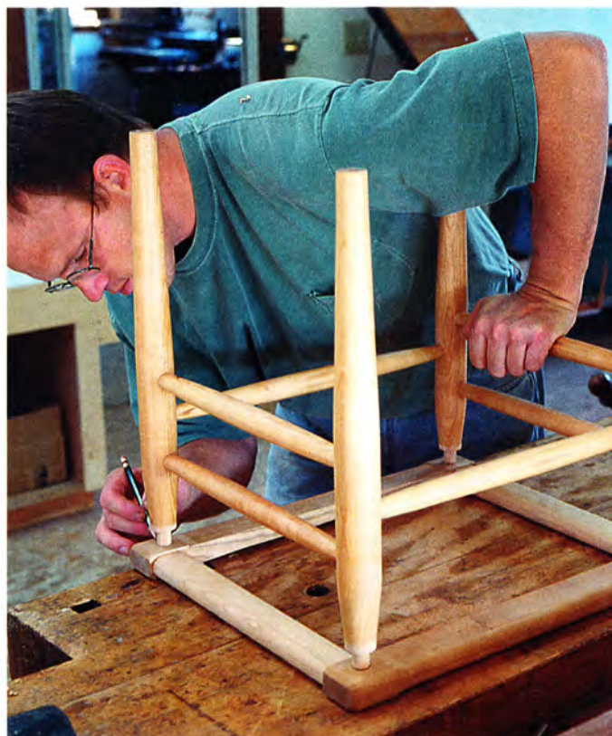
DRILL THE STEPPED MORTISES in the seat frame. Center the undercarriage on the seat frame and mark the mortise locations (left). The author uses a commercial counterbore bit (above) to machine the two-stage mortise accurately, in one shot.
