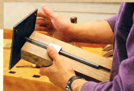
THE TAPPED STEEL BLOCK , buried in the glued-up pedestal, accepts the threaded rod attached to the seat bottom.
