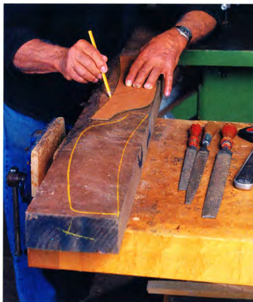
INTERLOCKING LAYOUT. Tracing a plan-view pattern, the author lays out chair arms in a 12/4 walnut board. He flops the pattern and nests the layouts to get as many arms as possible from the board.
