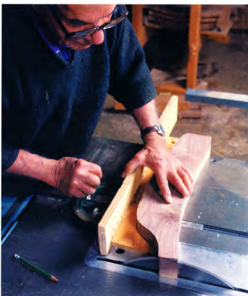
GOOD REFERENCES. The compound angle where the arm will join the chair's back leg is cut on the tablesaw while the arm is still flat on the top and bottom. A simple, curved plywood jig steadies the curved side of the arm for the cut.
