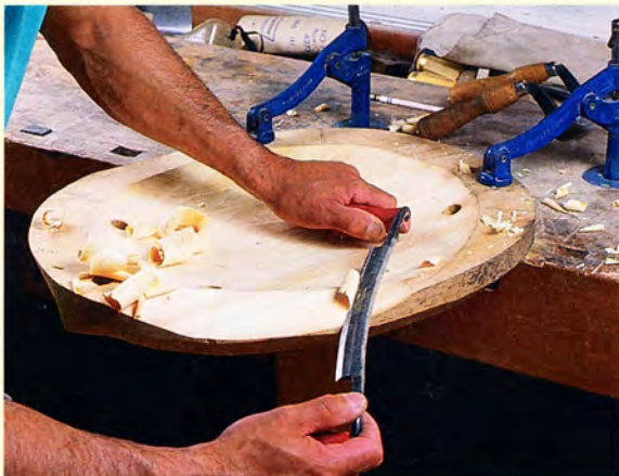
STEP 3: Shape convex surfaces with a drawknife.
