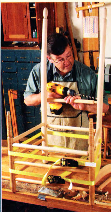
DRILL FOR THE CURVED back rails. With the chair temporarily assembled, Conover uses the curved back rail to align the drill at the correct angle.
