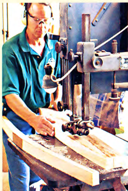
USING THE SIDE TEMPLATE , cut all of the legs from one wide 8/4 board to ensure uniform color (left). Lay out the legs for best grain orientation and strength (above).
