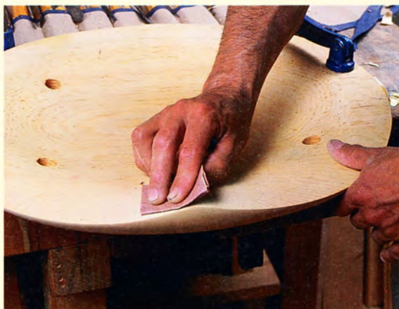
details with gouges. STEP 6: Smooth the seat contour with sandpaper.
