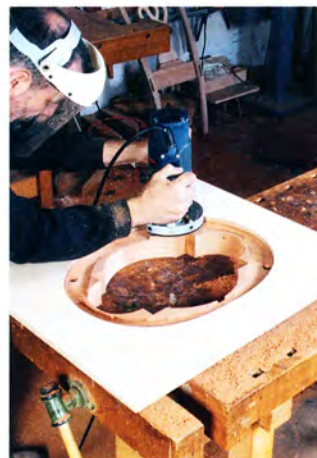
A ROUTER MAKES FAST WORK of the seat rabbet. Use a full-size oval pattern to establish the layout line.
