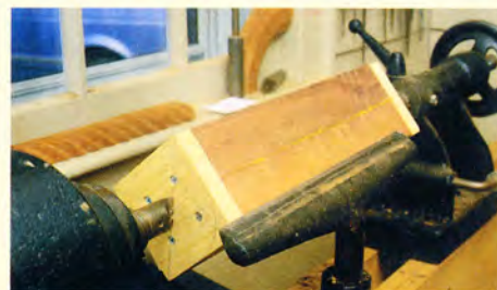
SCRAP PINE SHOES MAKE TURNING POSSIBLE. Take care placing the screws, so they won't interfere with turning tools.
