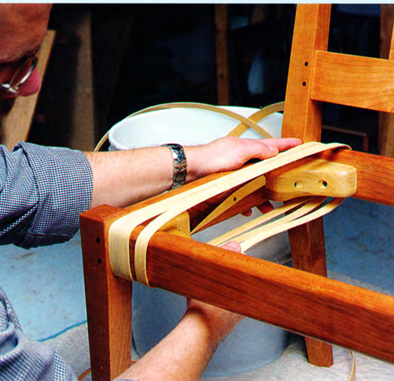
BEGINNING THE WARP. The first length of reed goes under the front seat rail and over the back and continues in this way to the end of the seat.
