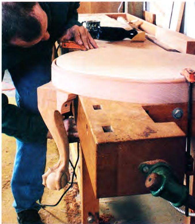
TEMPORARY FIXING. With the ball and claw complete, prepare to carve the knee by dry-fitting the leg to the frame. Use screws through the knee blocks to hold the leg in place.
