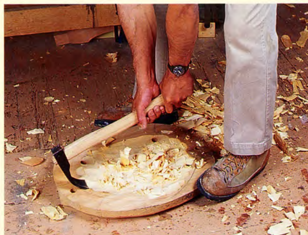
STEP 1: Rough the seat hollow with an adze.
