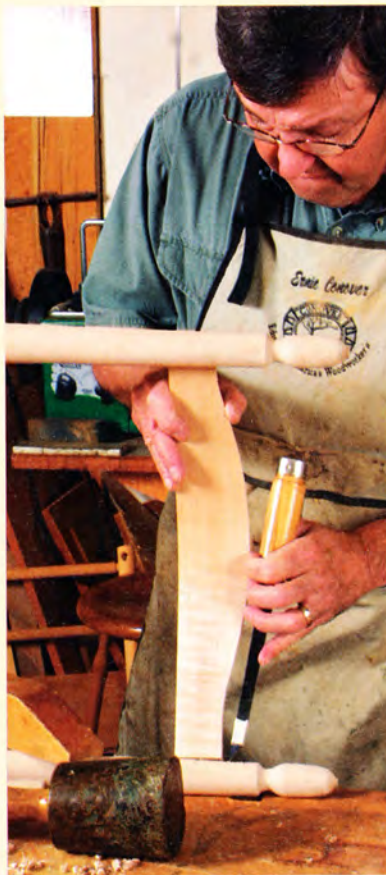
DETERMINE THE ANGLE of the mortise. Conover uses a mortising chisel to chop the mortises for the curved back slat. He rests the slat in place to set the proper angle for chopping (center). A piece of tape on the chisel marks the desired depth of the mortise (right) so that it can engage \frac{3}{8} in. of the tenon.
