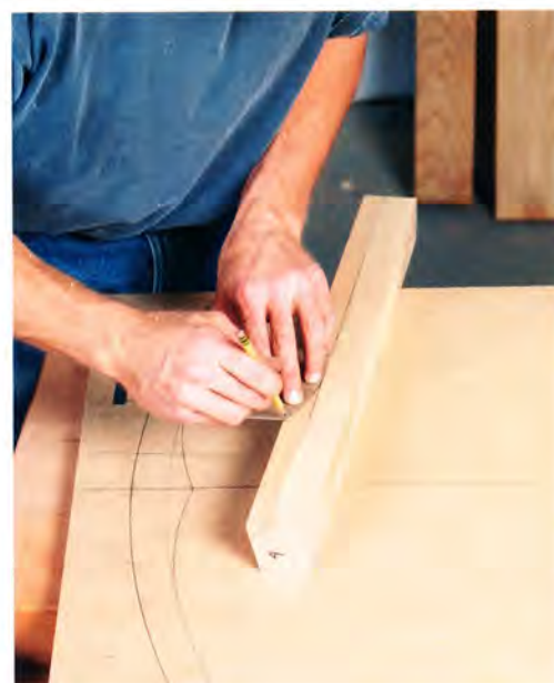
LAY OUT THE SECOND POMMEL CUT. The template drawing of the back of the seat, a straightedge, and a curved cardboard template are used to lay out the second cut that will finish up the rough pommel shape.
