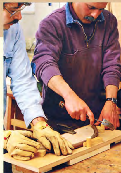
RAIL-BENDING JIG. Four hands are better than two for forcing the steamed rail into shape. The author is assisted by Les Katz, one of his students. Wedges hammered between the plywood form and the wooden pegs hold the rail tightly in place.
